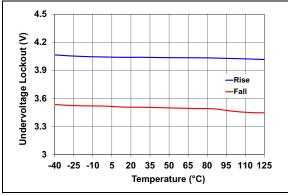
FIGURE 2-26: Undervoltage Lockout vs. Temperature.
