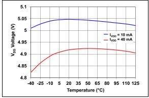
**FIGURE 2-18:**  $V_{DD}$  Voltage vs. Temperature.
