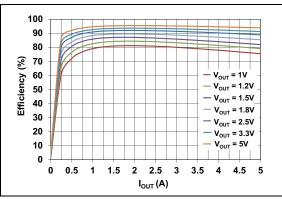
**FIGURE 2-2:** Efficiency vs. Output Current ( $V_{IN} = 12V$ ).
