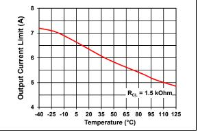
**FIGURE 2-24:** Output Current Limit vs. Temperature.
