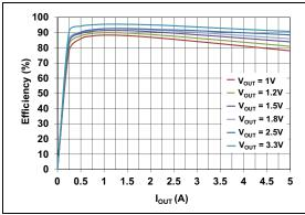
**FIGURE 2-1:** Efficiency vs. Output Current  $(V_{IN} = 5V)$ .
