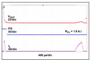
**FIGURE 2-36:** Behavior when Entering Short-Circuit.
