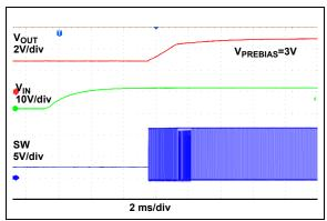
**FIGURE 2-30:** V<sub>IN</sub> Start-Up with Pre-biased Output.
