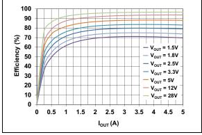
**FIGURE 2-4:** Efficiency vs. Output Current ( $V_{IN} = 48V$ ).
