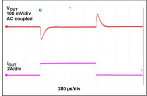
FIGURE 2-40: Load Transient Response (0 to 2.5A).
