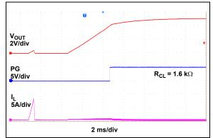
FIGURE 2-37: Recovery from Short-Circuit.
