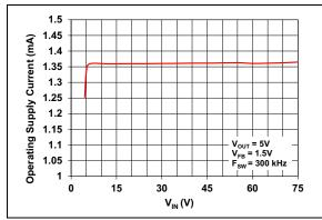
FIGURE 2-13: V<sub>IN</sub> Operating Supply Current vs. Input Voltage.
