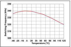
**FIGURE 2-22:** Switching Frequency vs. Temperature.
