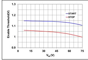
**FIGURE 2-19:** Enable Threshold vs. Input Voltage.
