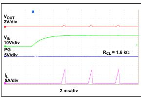
FIGURE 2-35: Power-Up into Short-Circuit.
