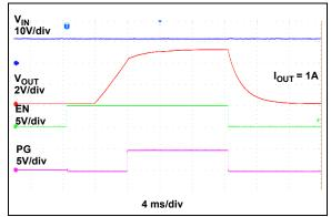
FIGURE 2-31: Enable Turn-On and Turn-Off.
