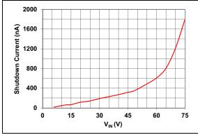
**FIGURE 2-15:** V<sub>IN</sub> Shutdown Current vs. Input Voltage.
