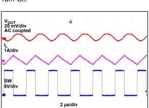
FIGURE 2-32: Switching Waveform (I<sub>OUT</sub> = 0A).
