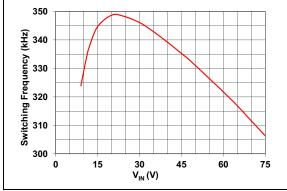
**FIGURE 2-21:** Switching Frequency vs. Input Voltage.
