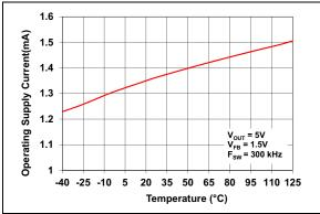
**FIGURE 2-14:** V<sub>IN</sub> Operating Supply Current vs. Temperature.
