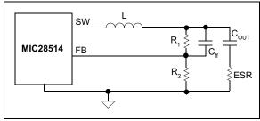
FIGURE 5-3: Inadequate Ripple at FB.
