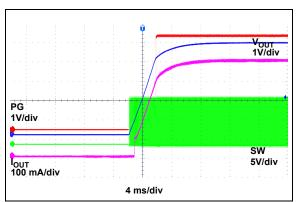
**FIGURE 2-39:** Recovery from Thermal Shutdown.
