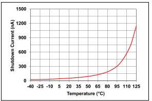
**FIGURE 2-16:**  $V_{IN}$  Shutdown Current vs. Temperature.
