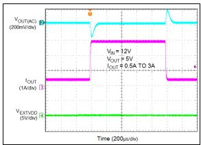
**FIGURE 4-4:** V<sub>OUT</sub> Load Transient with EXTVDD Connected to Ground.
