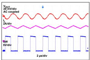
**FIGURE 2-33:** Switching Waveform  $(I_{OUT} = 5A)$ .
