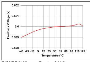
**FIGURE 2-27:** Feedback Voltage vs. Temperature.
