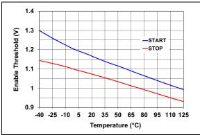
FIGURE 2-20: Enable Threshold vs. Temperature.
