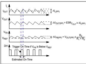
FIGURE 4-1: MIC28514 Control Loop Timing.
