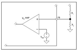
FIGURE 5-1: Voltage Divider Configuration.
