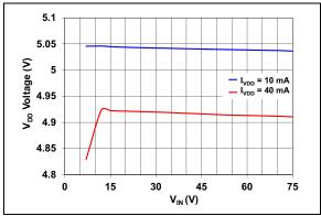
**FIGURE 2-17:**  $V_{DD}$  Voltage vs. Input Voltage.
