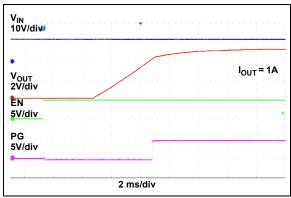
**FIGURE 2-28:** Enable Turn-On and Rise Time.
