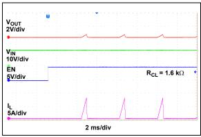
FIGURE 2-34: Enable into Short-Circuit.
