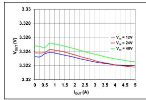
**FIGURE 2-7:** Output Voltage vs. Output Current ( $V_{OUT} = 3.3V$ ).
