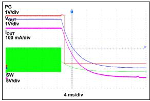
**FIGURE 2-38:** Behavior when Entering Thermal Shutdown.
