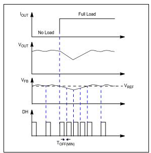
FIGURE 4-2: MIC28514 Load Transient Response.
