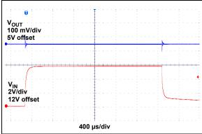
FIGURE 2-42: Line Transient Response (12V to 18V).
