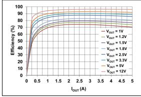
**FIGURE 2-3:** Efficiency vs. Output Current ( $V_{IN} = 24V$ ).
