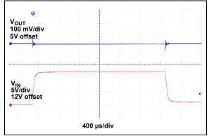
FIGURE 2-43: Line Transient Response (12V to 24V).
