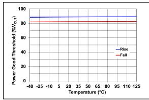
**FIGURE 2-25:** Power Good Threshold vs. Temperature.
