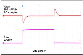
**FIGURE 2-41:** Load Transient Response (0 to 5A).
