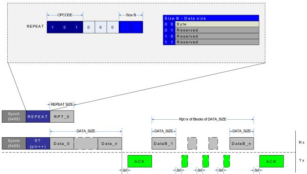
The figure above gives an example of repeat operation with an ST instruction using pointer post-increment operation. After the REPEAT instruction is sent with RPT\_0 = n, the first ST instruction is issued with SYNCH and Instruction frame, while the next n ST instructions are executed by only sending in data bytes according to the ST operand DATA SIZE, and maintaining the Acknowledge (ACK) handshake protocol.
