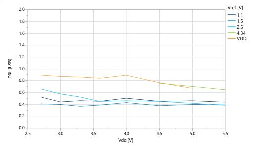
Figure 33-39. DNL vs. V<sub>ref</sub> (V<sub>DD</sub>=5.0V, f<sub>ADC</sub>=115 ksps), REFSEL = Internal Reference
