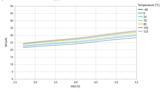
Figure 33-32. BOD Current vs.  $V_{DD}$  (Sampled BOD at 125 Hz)
