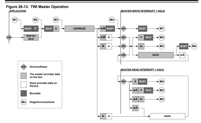
The number of interrupts generated is kept to a minimum by an automatic handling of most conditions.
