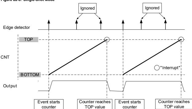
If the ASYNC bit in TCBn.CTRLB is '0', the event pulse needs to be longer than one system clock cycle in order to ensure edge detection.
