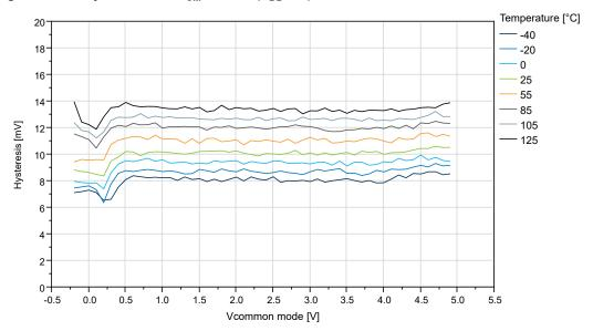
Figure 33-47. Hysteresis vs.  $V_{CM}$  - 10 mV to 50 mV ( $V_{DD}$ =5V, T=25°C)
