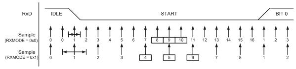
When the clock recovery logic detects a high-to-low (i.e., idle-to-start) transition on the RxD line, the Start bit detection sequence is initiated. Sample 1 denotes the first zero-sample, as shown in the figure. The clock recovery logic then uses three subsequent samples (samples 8, 9, and 10 in Normal mode, samples 4, 5, and 6 in Double-Speed mode) to decide if a valid Start bit is received:
