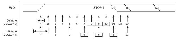
A new high-to-low transition indicating the Start bit of a new frame can come right after the last of the bits used for majority voting. For Normal-Speed mode, the first low-level sample can be at the point marked (A) in Stop Bit Sampling and Next Start Bit Sampling. For Double-Speed mode, the first low level must be delayed to point (B). Point (C) marks a Stop bit of full length at the nominal baud rate. The early Start bit detection influences the operational range of the receiver.
