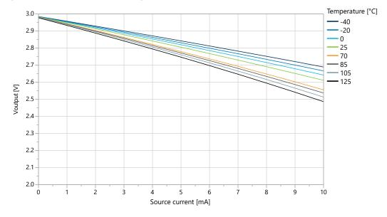
Figure 33-23. I/O Pin Output Voltage vs. Source Current (V<sub>DD</sub>=5.0V)
