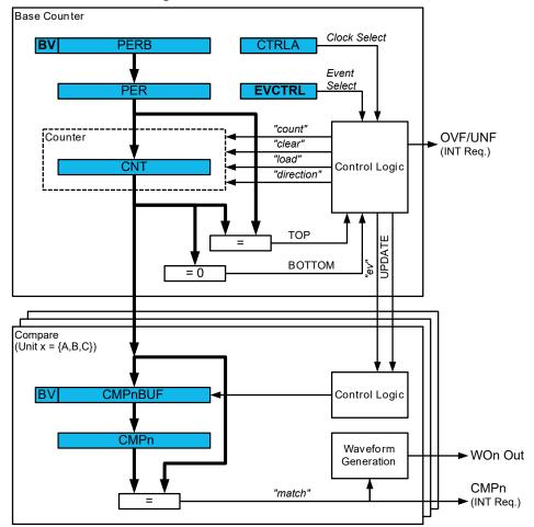
The counter register (TCAn.CNT), period registers with buffer (TCAn.PER and TCAn.PERBUF), and compare registers with buffers (TCAn.CMPx and TCAn.CMPBUFx) are 16-bit registers. All buffer registers have a buffer valid (BV) flag that indicates when the buffer contains a new value.
