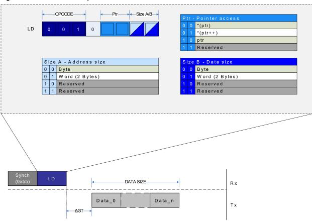
The figure above shows an example of a typical LD sequence, where data is received after the Guard Time period. Loading data from the UPDI Pointer register follows the same transmission protocol.
