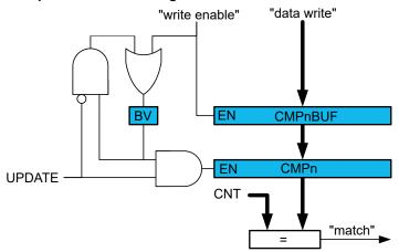
Both the TCAn.CMPn and TCAn.CMPnBUF registers are available as I/O registers. This allows initialization and bypassing of the buffer register and the double buffering function.
