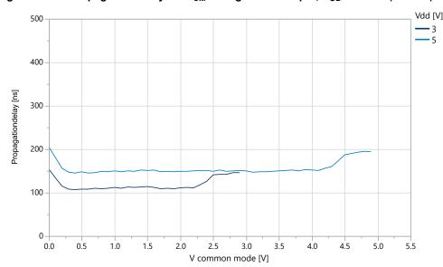
Figure 33-51. Propagation Delay vs. V<sub>CM</sub> Rising Positive Input, V<sub>OD</sub> = 30 mV (T=25°C)
