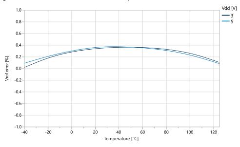
Figure 33-28. Internal 1.1V Reference vs. Temperature
