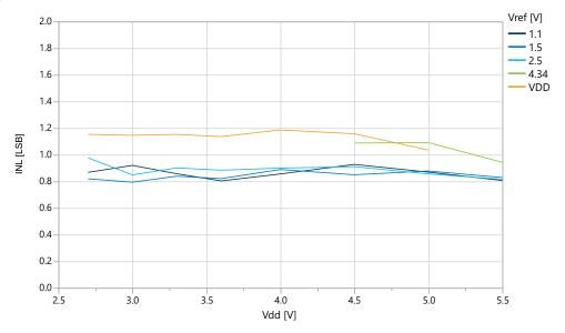
Figure 33-43. INL vs.  $V_{ref}$  ( $V_{DD}$ =5.0V,  $f_{ADC}$ =115 ksps), REFSEL = Internal Reference
