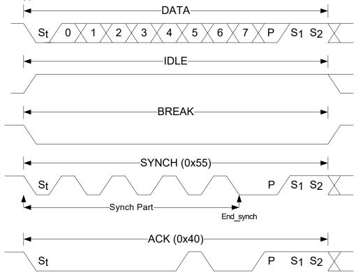
Data Frame Data frame consist of one Start bit (always low), eight data bits, one parity bit (even parity), and two Stop bits (always high). If the Start bit, parity bit, or Stop bits have an incorrect value, an error will be detected and signalized by the UPDI. The parity bit-check in the UPDI can be disabled by writing the PARD bit in UPDI.CTRLA, in which case the parity generation from the debugger can be ignored.
