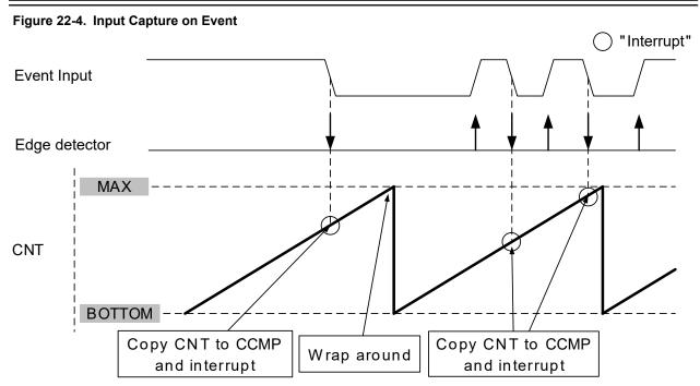
It is recommended to write zero to the TCBn.CNT register when entering this mode from any other mode.
