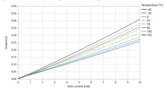
Figure 33-20. I/O Pin Output Voltage vs. Sink Current (V<sub>DD</sub>=5.0V)
