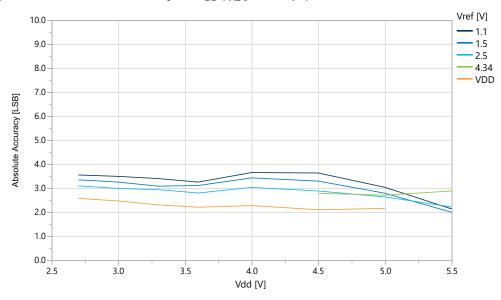
Figure 33-37. Absolute Accuracy vs. V<sub>ref</sub> (V<sub>DD</sub>=5.0V, f<sub>ADC</sub>=115 ksps), REFSEL = Internal Reference
