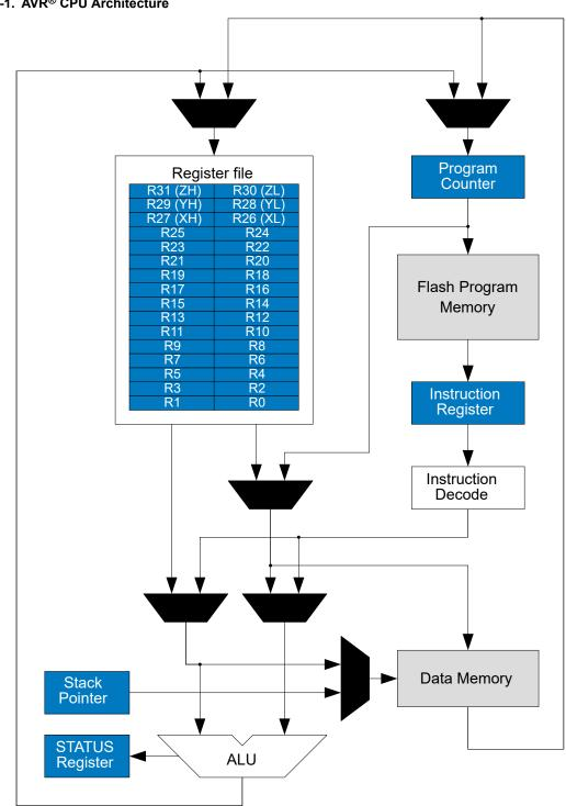
Figure 9-1. AVR® CPU Architecture
