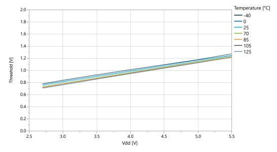
Figure 33-16. I/O Pin Input Threshold Voltage vs.  $V_{DD}$  (T=25°C)
