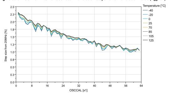
Figure 33-53. OSC20M Internal Oscillator: Frequency vs. Calibration Value (V<sub>DD</sub>=3V)
