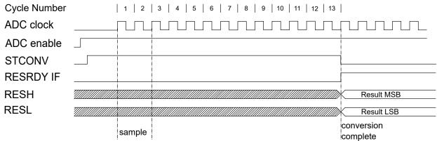
Both sampling time and sampling length can be adjusted using Sample Delay bit field in Control D (ADC.CTRLD) and sampling Sample Length bit field in the Sample Control register (ADC.SAMPCTRL). Both of these control the ADC sampling time in a number of CLK\_ADC cycles. This allows sampling high-impedance sources without relaxing conversion speed. See register description for further information. Total sampling time is given by:
