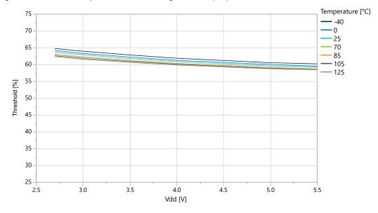
Figure 33-18. I/O Pin Input Threshold Voltage vs.  $V_{DD}\ (V_{IL})$
