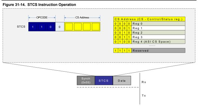
Figure 31-14 shows the data frame transmitted after the SYNCH and instruction frames. There is no response generated from the STCS instruction, as is the case for ST and STS.
