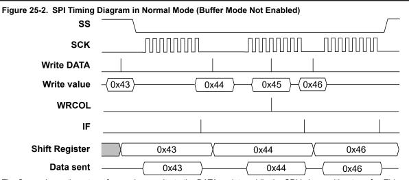
The figure shows three transfers and one write to the DATA register while the SPI is busy with a transfer. This write will be ignored and the Write Collision Flag (WRCOL in SPIn.INTFLAGS) is set.
