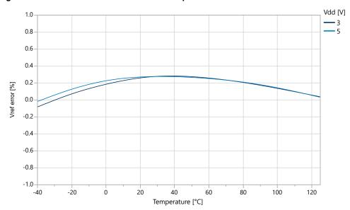
Figure 33-29. Internal 2.5V Reference vs. Temperature
