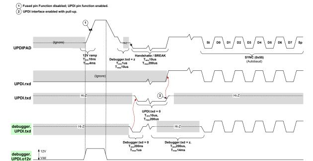
When enabled by 12V, only a POR will disable the UPDI configuration on the RESET pin, and restore the default setting. If issuing a UPDI Disable command through the UPDIDIS bit in UPDI.CTRLB, the UPDI will be reset and the clock request will be canceled, but the RESET pin will remain in UPDI configuration.
