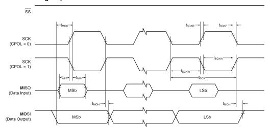
Figure 32-5. SPI - Timing Requirements in Slave Mode
