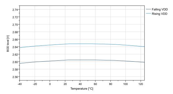
Figure 33-35. BOD Threshold vs. Temperature (Level 4.3V)
