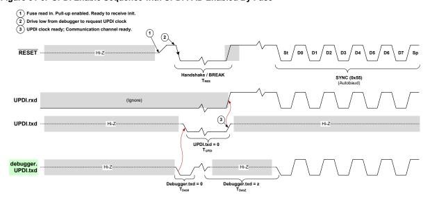
When the pull-up is detected, the debugger initiates the enable sequence by driving the line low for a duration of  $T_{Deb0}$  to ensure that the line is released from the debugger before the UPDI enable sequence is done.
