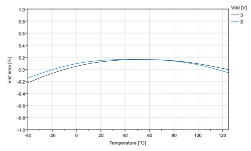
Figure 33-30. Internal 4.3V Reference vs. Temperature
