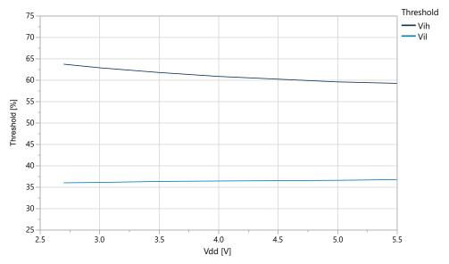
Figure 33-17. I/O Pin Input Threshold Voltage vs. V<sub>DD</sub> (V<sub>IH</sub>)
