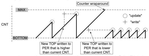
A counter wrap-around can occur in any mode of operation when up-counting without buffering. This is due to the fact that the registers TCAn.CNT and TCAn.PER are continuously compared: if a new TOP value is written to TCAn.PER that is lower than current TCAn.CNT, the counter will wrap first, before a compare match happens.
