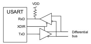
The XDIR pin goes high one baud clock cycle in advance of data being shifted out, to allow some guard time to enable the external line driver. The XDIR pin will remain high for the complete frame including Stop bit(s).
