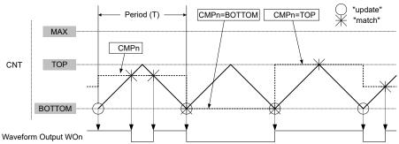
Using dual-slope PWM results in a lower maximum operation frequency compared to the single-slope PWM operation.
