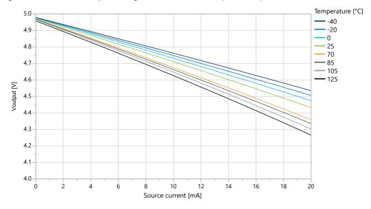
Figure 33-24. I/O Pin Output Voltage vs. Source Current (T=25°C)
