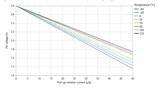
Figure 33-26. I/O Pin Pull-Up Resistor Current vs. Input Voltage (V<sub>DD</sub>=5.0V)
