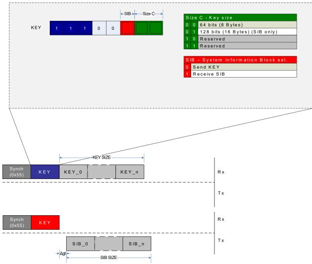
The figure above shows the transmission of a KEY and the reception of a SIB. In both cases, the <code>SIZE\_C</code> field in the opcode determines the number of frames being sent or received. There is no response after sending a <code>KEY</code> to the UPDI. When requesting the SIB, data will be transmitted from the UPDI according to the current Guard Time setting.
