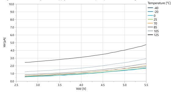
Figure 33-14. Standby Mode Supply Current vs. V<sub>DD</sub> (Sampled BOD Running at 1 kHz)
