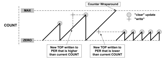
Figure 27-8. Changing the Top Value with Down-Counting Operation
