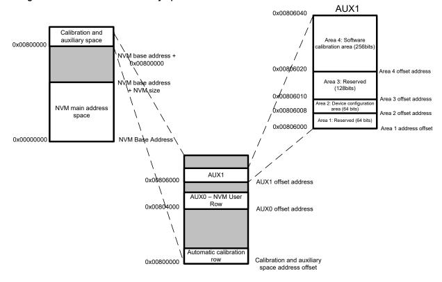
The values from the automatic calibration row are loaded into their respective registers at startup.
