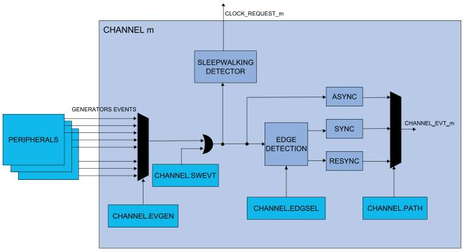
The path is selected by writing to the Path Selection bit group in the Channel register (CHANNEL.PATH).
