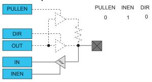
Figure 21-5. I/O Configuration - Input with Pull
