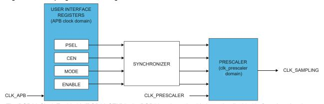
The BOD33 Clock Enable bit (BOD33.CEN) in the BOD33 register should always be disabled before changing the prescaler value. To change the prescaler value for the BOD33 during sampling mode, the following steps need to be taken:
