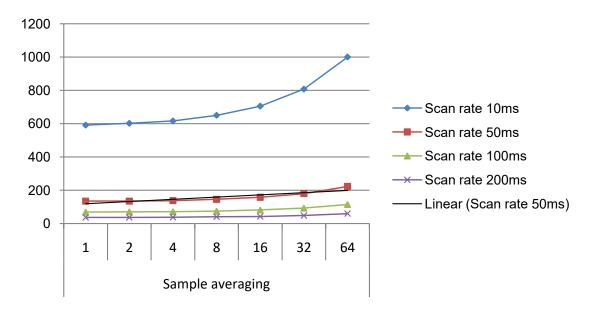
Figure 32-10. Power Consumption [μA] 10 sensors, noise countermeasures Enabled, f=48MHz, Vcc=3.3V
