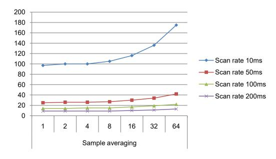
Figure 32-9. Power Consumption [μA] 10 sensors, noise countermeasures disabled, f=48MHz, Vcc=3.3V
