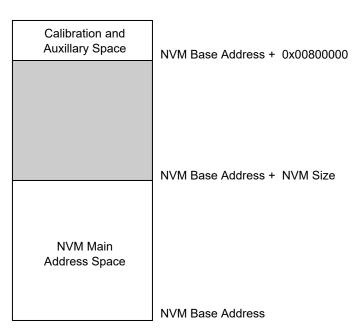
The lower rows in the NVM main address space can be allocated as a boot loader section by using the BOOTPROT fuses, and the upper rows can be allocated to EEPROM Emulation, as shown in the figure below.
