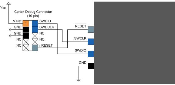
Table 36-9. Cortex Debug Connector (10-pin)
