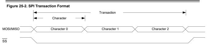
The SPI host must pull the SPI select line  $(\overline{SS})$  of the desired client low to initiate a transaction if multiple clients are connected to the bus. The SPI select line can be wired low if there is only one SPI client on the bus. The host and client prepare data to send via their respective Shift registers, and the host generates the serial clock on the SCK
