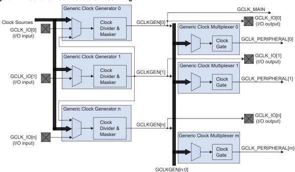
Figure 14-2. Generic Clock Controller Block Diagram<sup>(1)</sup>
