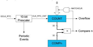
Figure 18-2. RTC Block Diagram (Mode 1 — 16-Bit Counter)
