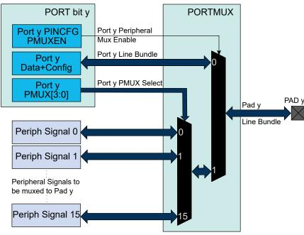
Figure 21-3. Overview of the peripheral functions multiplexing
