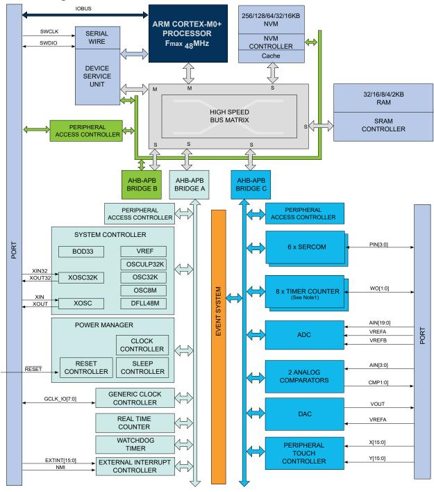
**Note:** 1. Some products have different number of SERCOM instances, Timer/Counter instances, PTC signals and ADC signals. Refer to *Peripherals Configuration Summary* for details.
