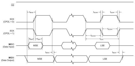
Figure 34-8. SPI Timing Requirements in Client Mode
