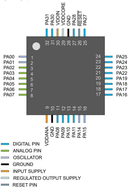
Note: In the VQFN32/TQFP32 package, both VDDIO and VDDANA are internally connected.
