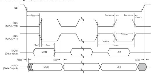
Table 34-46. SPI Timing Characteristics and Requirements<sup>(1)</sup>
