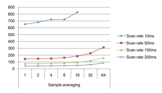
Figure 32-11. Power Consumption [μA] 100 sensors, noise countermeasures disabled, f=48MHz, Vcc=3.3V
