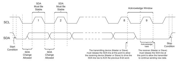
Figure 5-1. Start Condition, Data Transitions, Stop Condition and Acknowledge
