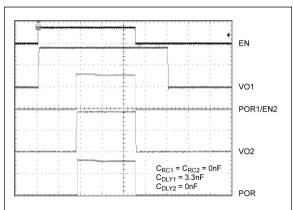
FIGURE 5-4: Window Sequencing Example.
