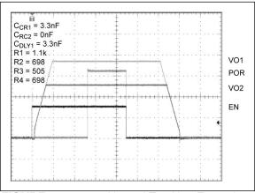
FIGURE 5-7: Normal Tracking Example.
