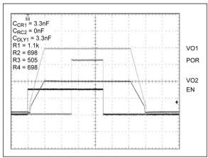
**FIGURE 5-11:** DDR Memory Tracking Example.
