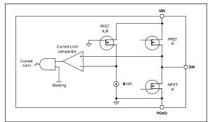
FIGURE 5-12: Current Limit Detail.
