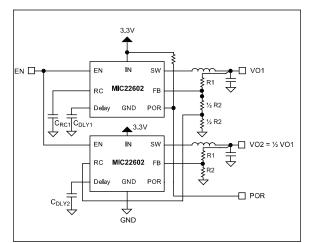
**FIGURE 5-10:** DDR Memory Tracking Circuit.
