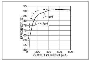
FIGURE 5-2: Efficiency vs. Inductance.
