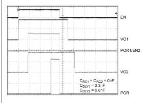
FIGURE 5-5: Delayed Sequencing Example.
