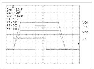
FIGURE 5-9: Ratio Metric Tracking Example.
