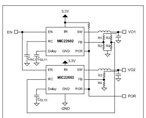
FIGURE 5-6: Normal Tracking Circuit.
