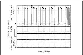
FIGURE 2-24: Hiccup Current Limit Behavior.
