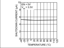
FIGURE 2-1: Shutdown Current vs. ' Temperature
