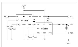
FIGURE 5-3: Sequencing MIC22602 Circuit.
