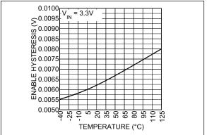
FIGURE 2-6: Enable Hysteresis vs. Temperature.
