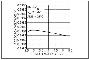
FIGURE 2-3: Feedback Voltage vs. Input Voltage.
