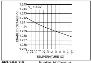
FIGURE 2-5: Enable Voltage vs. Temperature.
