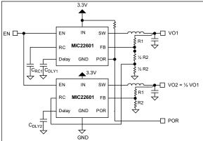
FIGURE 5-9: DDR Memory Tracking Circuit.
