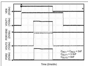
FIGURE 5-3: Window Sequencing Example.
