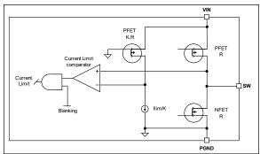
FIGURE 5-11: Current Limit Detail.
