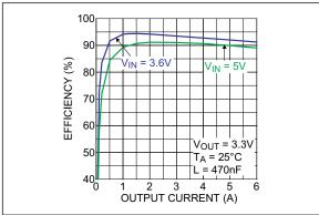
FIGURE 2-13: Efficiency vs. Load Current.
