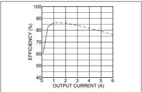
**FIGURE 5-1:** Efficiency 3.6V to 1.8V, L = 470 nH.
