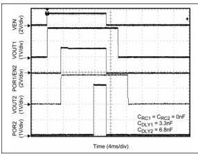
**FIGURE 5-4:** Delayed Sequencing Example.
