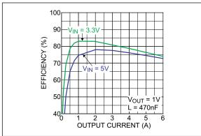
FIGURE 2-15: Efficiency vs. Output Current.
