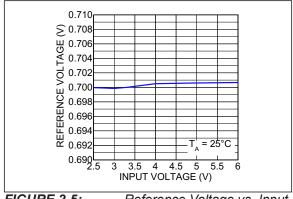
FIGURE 2-5: Reference Voltage vs. Input Voltage.
