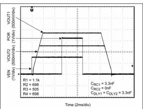
FIGURE 5-6: Normal Tracking Example.
