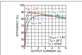
FIGURE 2-14: Efficiency vs. Output Current.
