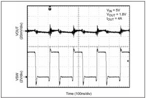
**FIGURE 2-24:** Output Noise and Ripple.
