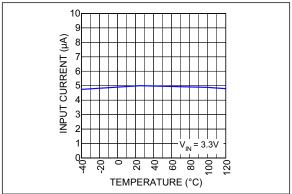
FIGURE 2-2: Shutdown Current vs. Temperature.
