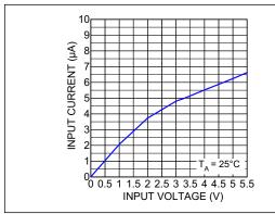
FIGURE 2-1: Shutdown Current vs. Input Voltage.
