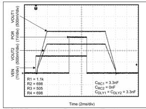
FIGURE 5-8: Ratio Metric Tracking Example.
