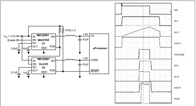
FIGURE 2-25: Sequencing Circuit and Waveform.
