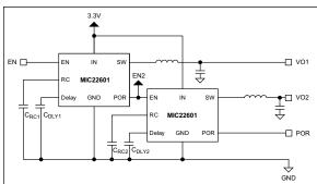
FIGURE 5-2: Sequencing MIC22601 Circuit.
