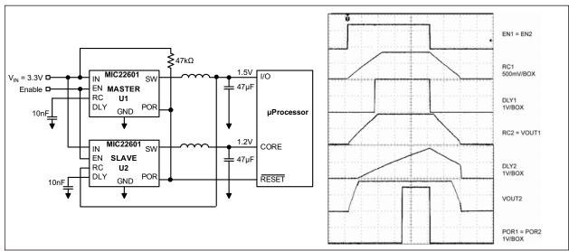
FIGURE 2-26: Tracking Circuit and Waveform.
