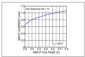
**FIGURE 2-3:** Quiescent Current vs. Input Voltage.
