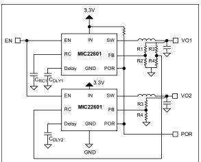
FIGURE 5-5: Normal Tracking Circuit.
