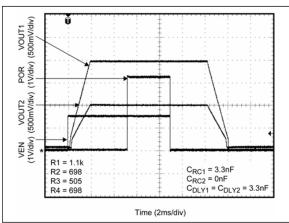
**FIGURE 5-10:** DDR Memory Tracking Example.
