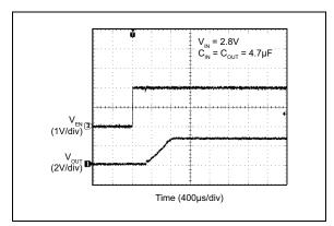
FIGURE 2-20: Enable Turn-On.
