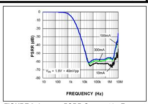
FIGURE 2-4:  $PSRR C_{OUT} = 10 \mu F.$
