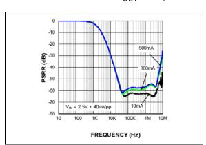
FIGURE 2-2: PSRR  $C_{OUT} = 4.7 \mu F$ .
