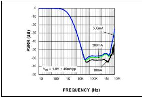
**FIGURE 2-1:** PSRR  $C_{OUT} = 4.7 \mu F$ .
