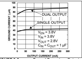
FIGURE 2-5: Ground Current vs. Output Current.
