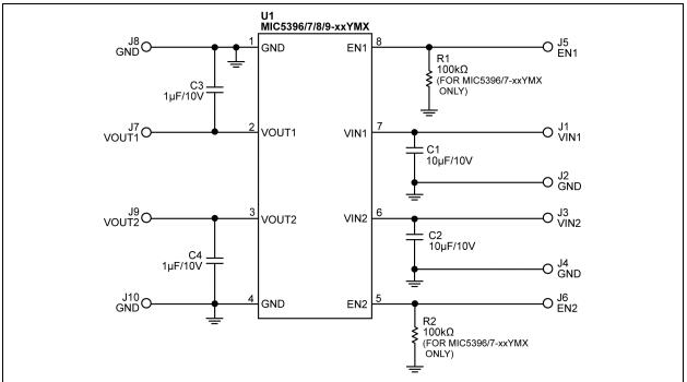
FIGURE 5-1: MIC5396/7/8/9-x.xYMX Typical Application Schematic.
