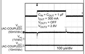
FIGURE 2-13: Line Transient V<sub>IN2</sub>.
