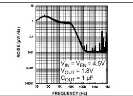
FIGURE 2-10: Output Noise Spectral Density.
