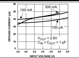
FIGURE 2-4: Ground Current vs. Input Voltage.
