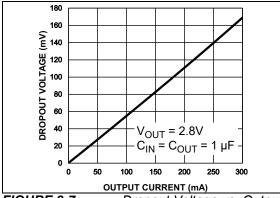
FIGURE 2-7: Dropout Voltage vs. Output Current.
