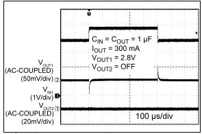
FIGURE 2-12: Line Transient V<sub>IN1</sub>.
