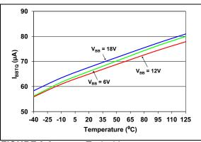
FIGURE 2-3: Typical IBBTO vs. Temperature – 5.0V.
