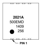
8-Lead SOIC (150 mil) (MCP2021A)
