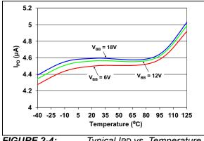
FIGURE 2-4: Typical IPD vs. Temperature – 5.0V.
