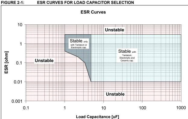
Note 1: The graph shows the minimum required capacitance after derating due to tolerance, temperature and voltage.
