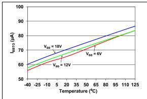
FIGURE 2-6: Typical IBBTO vs. Temperature – 3.3V.
