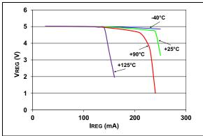
**FIGURE 2-8:** 5.0V VREG vs. IREG at VBB = 12V.
