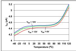
FIGURE 2-7: Typical IPD vs. Temperature – 3.3V.
