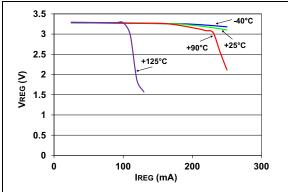
**FIGURE 2-9:** 3.3V VREG vs. IREG at VBB = 12V.
