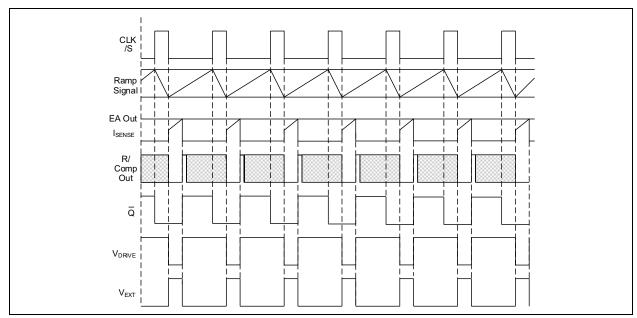
FIGURE 4-1: PWM Timing Diagram.
