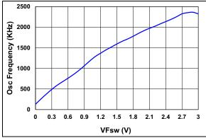
**FIGURE 2-19:** Oscillator Frequency vs.  $F_{sw}$  Pin Voltage ( $V_{CC} = 5V$ , Temperature = 25°C).
