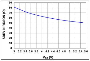
**FIGURE 2-7:** SRDV P-Channel RDSON vs. Input Voltage.
