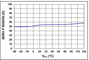
**FIGURE 2-28:** SRDV P-Channel RDSON vs. Temperature.
