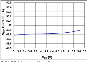
**FIGURE 2-3:** V<sub>REF</sub> Current vs. Input Voltage.
