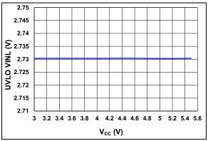
FIGURE 2-10: UVLO VINL Threshold vs. Input Voltage.
