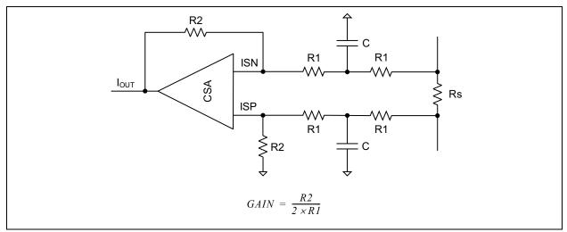
FIGURE 4-6: Current Sense Amplifier Gain Set.
