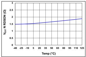
**FIGURE 2-25:**  $V_{EXT}$  N-Channel RDSON vs. Temperature.
