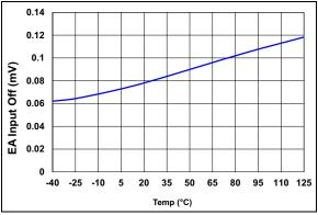
**FIGURE 2-22:** Error Amplifier Input Offset vs. Temperature.
