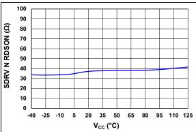
FIGURE 2-27: SRDV N-Channel RDSON vs. Temperature.
