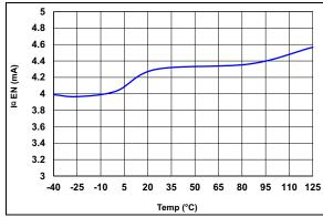
**FIGURE 2-24:** Input Quiescent Enable Current vs. Temperature.
