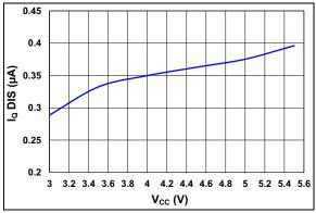
**FIGURE 2-1:** Input Quiescent Disable Current vs. Input Voltage.
