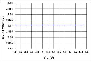
FIGURE 2-11: UVLO VINH Threshold vs. Input Voltage.
