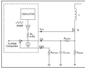
FIGURE 4-3: Slope Compensation Circuit.
