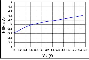
**FIGURE 2-2:** Input Quiescent Enable Current vs. Input Voltage.
