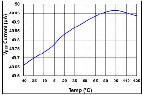
**FIGURE 2-13:**  $V_{REF}$  Current vs. Temperature.
