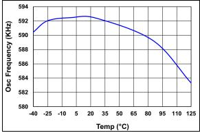
**FIGURE 2-18:** Oscillating Frequency vs. Temperature at 600 kHz.
