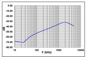
**FIGURE 2-30:** Current Sense Amplifier CMRR at  $V_{CC} = 5V$ .
