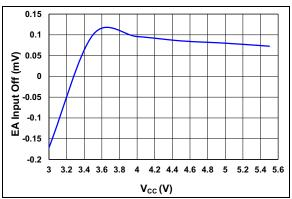
**FIGURE 2-8:** Error Amplifier Input Offset vs. Input Voltage.
