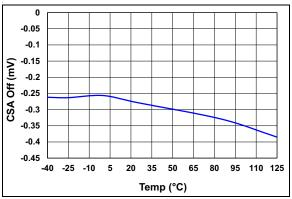
**FIGURE 2-14:** Current Sense Amplifier Offset Voltage vs. Temperature.
