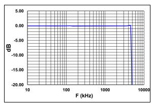
**FIGURE 2-29:** Current Sense Amplifier BW at  $V_{CC} = 5V$ .
