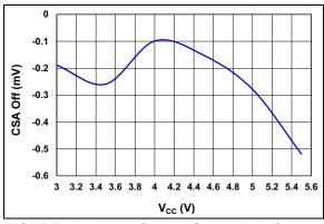
**FIGURE 2-9:** Current Sense Amplifier Offset vs. Input Voltage.
