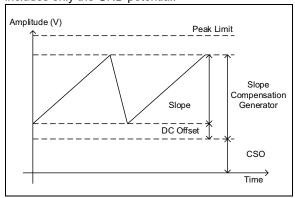
FIGURE 4-2: Slope Compensation Signal.
