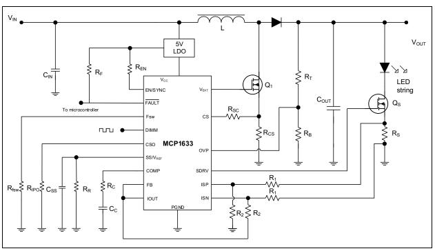
FIGURE 5-1: MCP1633 Typical Boost Converter.
