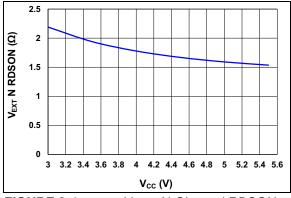
**FIGURE 2-4:**  $V_{EXT}$  N-Channel RDSON vs. Input Voltage.
