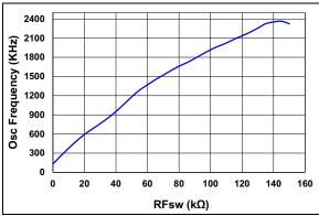
**FIGURE 2-20:** Oscillator Frequency vs.  $RF_{SW}$  ( $V_{CC}$  = 5V, Temperature = 25°C).
