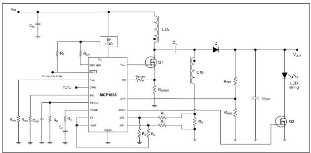
FIGURE 5-2: MCP1633 Typical SEPIC Converter — Demo Board ADM01002.
