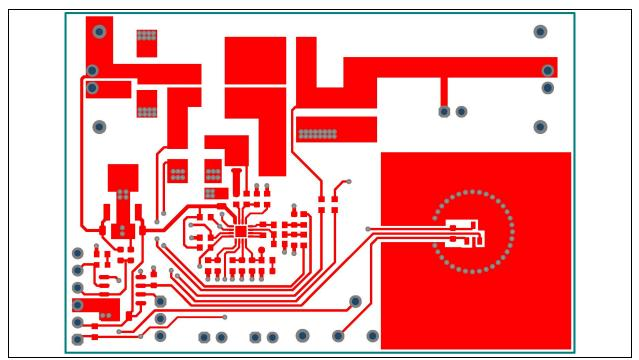
FIGURE 5-6: MCP1633 Demo Board ADM01002 — Top Copper.
