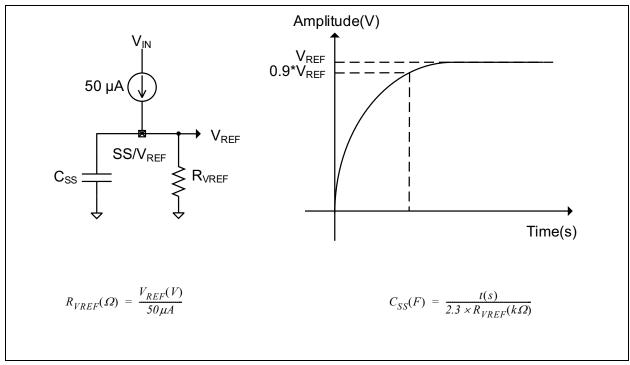
FIGURE 4-4: Reference Voltage Generator.
