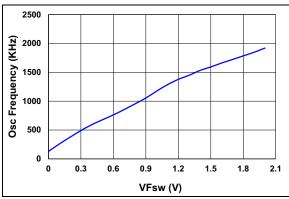
**FIGURE 2-21:** Oscillator Frequency vs.  $F_{sw}$  Pin Voltage ( $V_{CC} = 3V$ , Temperature = 25°C).
