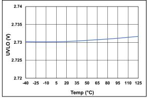
**FIGURE 2-16:** UVLO VINLO Threshold vs. Temperature.
