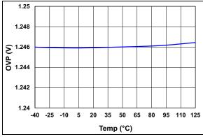
FIGURE 2-15: OVP vs. Temperature.
