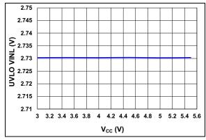
FIGURE 2-12: OVP VINL Threshold vs. Input Voltage.
