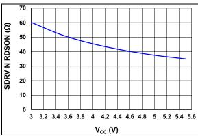
FIGURE 2-6: SRDV N-Channel RDSON vs. Input Voltage.
