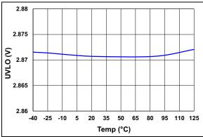
FIGURE 2-17: UVLO VINHI Threshold vs. Temperature.
