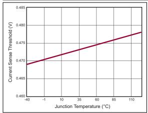
**FIGURE 2-1:** Threshold Voltage  $V_{TH}$  vs. Junction Temperature  $T_{J}$ .
