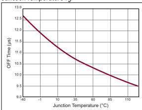
**FIGURE 2-2:** Off-Time  $T_{OFF}$  vs. Junction Temperature  $T_{J}$ .
