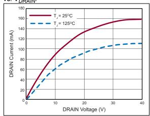
**FIGURE 2-6:** Output Characteristics  $I_{DRAIN}$  vs  $V_{DRAIN}$ .
