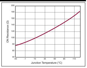
**FIGURE 2-4:** ON Resistance  $R_{ON}$  vs. Junction Temperature  $T_J$ .
