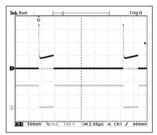
**FIGURE 5-4:** Switching Waveforms. CH1: V<sub>RSENSE</sub>, CH2: V<sub>DRAIN</sub>.
