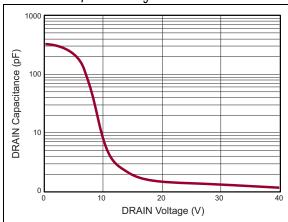
FIGURE 2-5: DRAIN Capacitance  $C_{DRAIN}$  vs.  $V_{DRAIN}$ .
