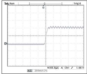
**FIGURE 5-6:** PWM Dimming–Rising Edge. CH4: 10 × I<sub>OUT</sub>.
