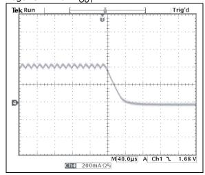
FIGURE 5-7: PWM Dimming–Falling Edge. CH4: 10 × I<sub>OUT</sub>.
