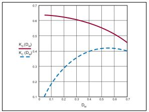
**FIGURE 5-1:** Conduction Loss Coefficients  $K_C$  and  $K_D$ .
