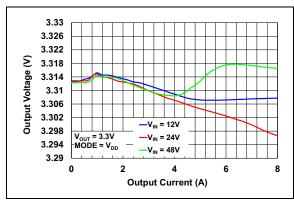
**FIGURE 2-6:** Output Voltage vs. Output Current ( $V_{OUT} = 3.3V$ ).
