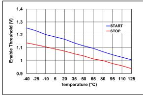
FIGURE 2-32: Enable Threshold vs. Temperature.
