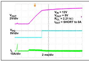
FIGURE 2-55: Recovery from Short Circuit.
