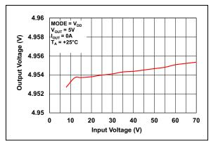
**FIGURE 2-13:** Output Voltage vs. Input Voltage  $(V_{OUT} = 5V)$ .
