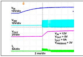
**FIGURE 2-44:** V<sub>IN</sub> Start-up with Pre-Biased Output.
