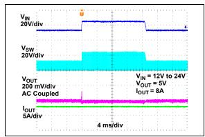
**FIGURE 2-65:** Line Transient Response  $(V_{IN} = 12V \text{ to } 24V)$ .
