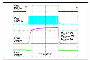
FIGURE 2-47: Enable Turn-On/Turn-Off.
