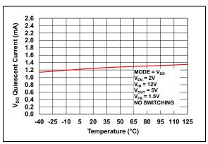
**FIGURE 2-26:**  $V_{DD}$  Quiescent Current vs. Temperature (MODE =  $V_{DD}$ ).
