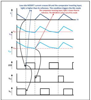
FIGURE 4-3: MIC28517 Control Loop Timing (HLL Mode).
