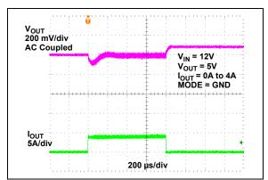
FIGURE 2-59: Load Transient Response – HLL (I<sub>OUT</sub> = 0A to 4A).
