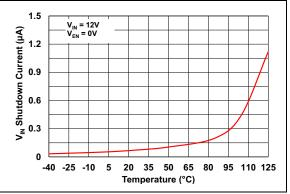
**FIGURE 2-22:**  $V_{IN}$  Shutdown Current vs. Temperature.
