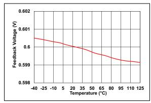
**FIGURE 2-41:** Feedback Voltage vs. Temperature.
