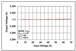
**FIGURE 2-12:** Output Voltage vs. Input Voltage  $(V_{OUT} = 3.3V)$ .
