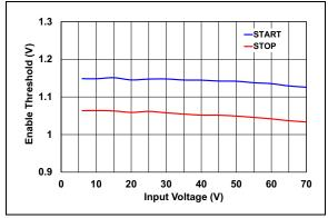
FIGURE 2-31: Enable Threshold vs. Input Voltage.
