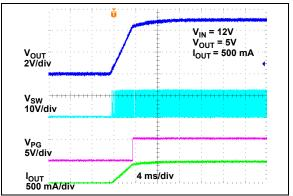
FIGURE 2-57: Recovery from Thermal Shutdown.
