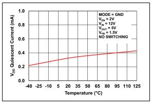
**FIGURE 2-28:**  $V_{DD}$  Quiescent Current vs. Temperature (MODE = GND).
