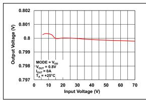
**FIGURE 2-9:** Output Voltage vs. Input Voltage  $(V_{OUT} = 0.8V)$ .
