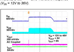
**FIGURE 2-67:** Line Transient Response  $(V_{IN} = 12V \text{ to } 48V).$
