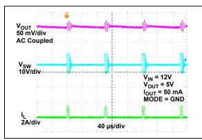
**FIGURE 2-48:** Switching Waveforms – HLL  $(V_{OUT} = 5V, I_{OUT} = 50 \text{ mA}).$
