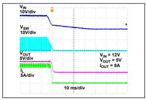
FIGURE 2-46: V<sub>IN</sub> Soft Turn-Off.
