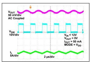
**FIGURE 2-49:** Switching Waveforms – CCM ( $V_{OUT} = 5V$ ,  $I_{OUT} = 50$  mA).
