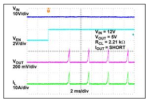
FIGURE 2-52: Enable into Short Circuit.
