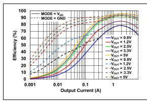
**FIGURE 2-1:** Efficiency vs. Output Current ( $V_{IN} = 12V$ ).
