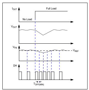
**FIGURE 4-2:** MIC28517 Load Transient Response.
