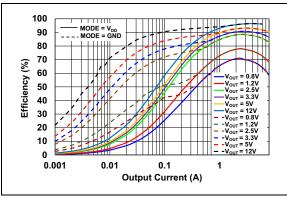
**FIGURE 2-2:** Efficiency vs. Output Current ( $V_{IN} = 24V$ ).
