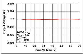
**FIGURE 2-11:** Output Voltage vs. Input Voltage  $(V_{OUT} = 2.5V)$ .
