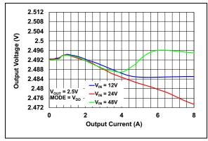
**FIGURE 2-5:** Output Voltage vs. Output Current ( $V_{OUT} = 2.5V$ ).
