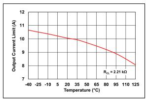
**FIGURE 2-37:** Output Current Limit vs. Temperature.
