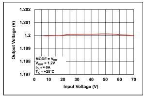
**FIGURE 2-10:** Output Voltage vs. Input Voltage  $(V_{OUT} = 1.2V)$ .
