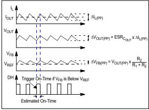
FIGURE 4-1: MIC28517 Control Loop Timing.
