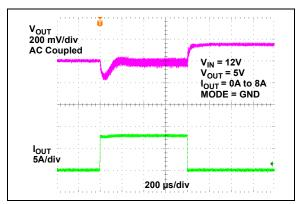
**FIGURE 2-61:** Load Transient Response –  $HLL(I_{OUT} = 0A \text{ to } 8A, V_{IN} = 12V).$
