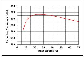
FIGURE 2-33: Switching Frequency vs. Input Voltage.
