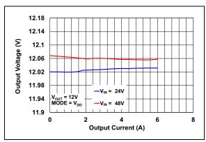
**FIGURE 2-8:** Output Voltage vs. Output Voltage  $(V_{OUT} = 12V)$ .
