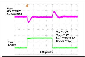
**FIGURE 2-62:** Load Transient Response –  $CCM(I_{OUT} = 0A \text{ to } 8A, V_{IN} = 70V).$
