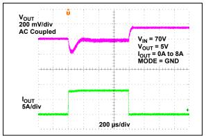
**FIGURE 2-63:** Load Transient Response –  $HLL(I_{OUT} = 0A \text{ to } 8A, V_{IN} = 70V).$
