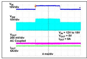
**FIGURE 2-64:** Line Transient Response  $(V_{IN} = 12V \text{ to } 18V)$ .
