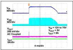
**FIGURE 2-68:** Line Transient Response  $(V_{IN} = 12V \text{ to } 70V).$
