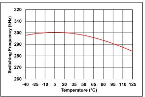
**FIGURE 2-34:** Switching Frequency vs. Temperature.
