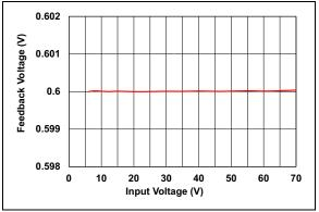
**FIGURE 2-40:** Feedback Voltage vs. Input Voltage.
