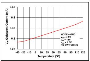
**FIGURE 2-18:**  $V_{IN}$  Quiescent Current vs. Temperature (MODE = GND).
