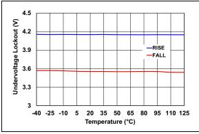
**FIGURE 2-39:** Undervoltage Lockout vs. Temperature.
