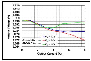
FIGURE 2-4: Output Voltage vs. Output Current ( $V_{OUT} = 0.8V$ ).
