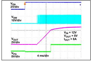
**FIGURE 2-42:** Enable Turn-On and Rise Time.
