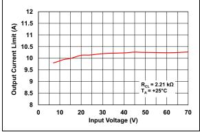
**FIGURE 2-36:** Output Current Limit vs. Input Voltage.
