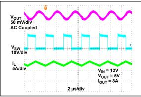
**FIGURE 2-50:** Switching Waveforms  $(V_{OUT} = 5V, I_{OUT} = 8A)$ .
