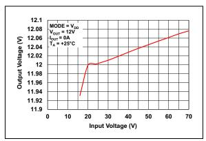
**FIGURE 2-14:** Output Voltage vs. Input Voltage  $(V_{OUT} = 12V)$ .
