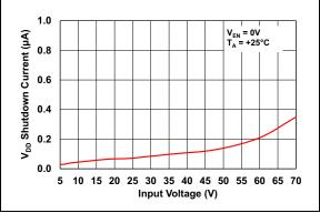
**FIGURE 2-30:**  $V_{DD}$  Shutdown Current vs. Input Voltage.
