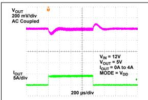
**FIGURE 2-58:** Load Transient Response –  $CCM (I_{OUT} = 0A \text{ to } 4A).$
