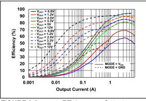
**FIGURE 2-3:** Efficiency vs. Output Current ( $V_{IN} = 48V$ ).
