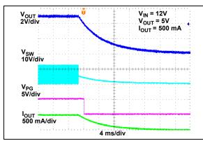
**FIGURE 2-56:** Behavior when Entering Thermal Shutdown.
