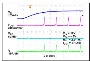
FIGURE 2-53: Power-up into Short Circuit.
