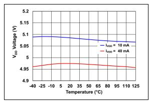
**FIGURE 2-24:**  $V_{DD}$  Voltage vs. Temperature.
