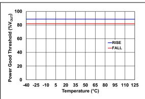
FIGURE 2-38: Power Good Threshold vs. Temperature.
