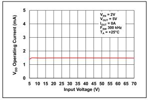
**FIGURE 2-29:**  $V_{DD}$  Operating Current vs. Input Voltage.
