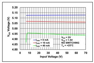
**FIGURE 2-23:**  $V_{DD}$  Voltage vs. Input Voltage.
