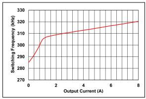
**FIGURE 2-35:** Switching Frequency vs. Output Current.
