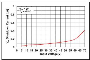
**FIGURE 2-21:** V<sub>IN</sub> Shutdown Current vs. Input Voltage.
