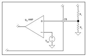
FIGURE 5-1: Voltage Divider Configuration.
