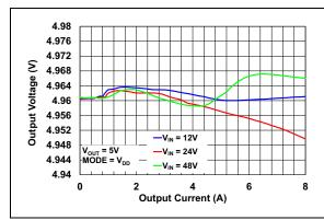
**FIGURE 2-7:** Output Voltage vs. Output Current  $(V_{OUT} = 5V)$ .
