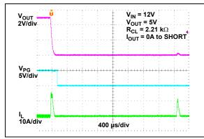
**FIGURE 2-54:** Behavior when Entering Short Circuit.
