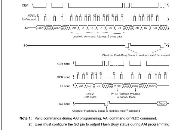
FIGURE 5-7: AUTO ADDRESS INCREMENT (AAI) WORD PROGRAM SEQUENCE WITH SOFTWARE END OF WRITE DETECTION
