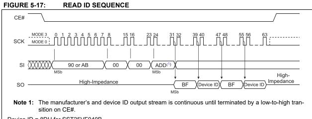
Device ID = 8DH for SST25VF040B.
