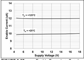
FIGURE 2-27: Enable Current vs. Supply Voltage.
