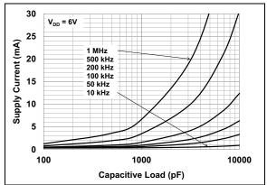
**FIGURE 2-23:** Supply Current vs. Capacitive Load ( $V_{DD} = 6V$ ).
