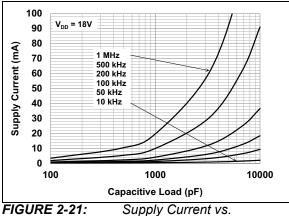
Capacitive Load ( $V_{DD} = 18V$ ).
