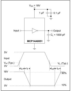
FIGURE 4-1: Inverting Driver Timing Waveform.
