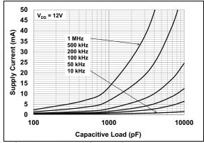
**FIGURE 2-22:** Supply Current vs. Capacitive Load ( $V_{DD}$  = 12V).
