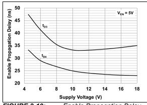
**FIGURE 2-10:** Enable Propagation Delay vs. Supply Voltage.
