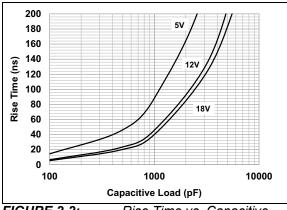
FIGURE 2-2: Rise Time vs. Capacitive Load.
