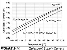
FIGURE 2-14: vs. Temperature.
