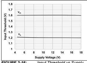
FIGURE 2-16: Input Threshold vs Supply Voltage.
