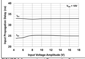
**FIGURE 2-8:** Input Propagation Delay Time vs. Input Amplitude.
