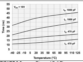
FIGURE 2-5: Rise and Fall Time vs. Temperature.
