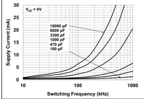
**FIGURE 2-26:** Supply Current vs. Frequency  $(V_{DD} = 6V)$ .
