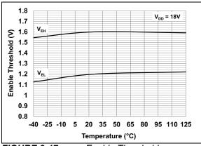
**FIGURE 2-17:** Enable Threshold vs. Temperature.
