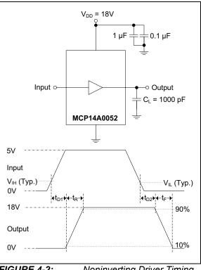
FIGURE 4-2: Noninverting Driver Timing Waveform.
