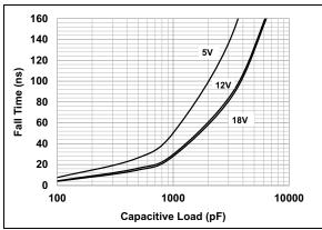
FIGURE 2-4: Fall Time vs. Capacitive Load.
