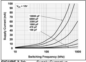
**FIGURE 2-24:** Supply Current vs. Frequency (V<sub>DD</sub> = 18V).
