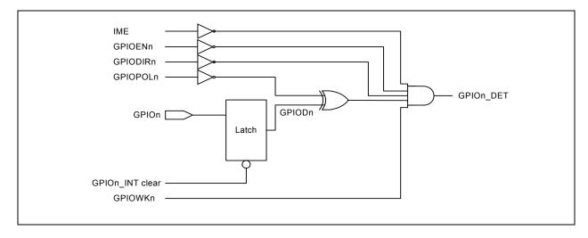
**Note:** The IME bit is in the Hardware Configuration Register (HW\_CFG). General Purpose IO Configuration Register (GPIO\_CFG) and General Purpose IO Wake Enable and Polarity Register (GPIO\_WAKE) must be set accordingly. Diagram does not represent actual hardware implementation.
