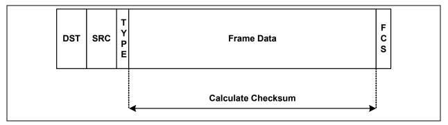
In mode 1, the RXCOE supports VLAN tags and a SNAP header. In this mode, the RXCOE calculates the checksum at the start of L3 packet. The VLAN1 tag register is used by the RXCOE to indicate what protocol type is to be used to indicate the existence of a VLAN tag. This value is typically 8100h.
