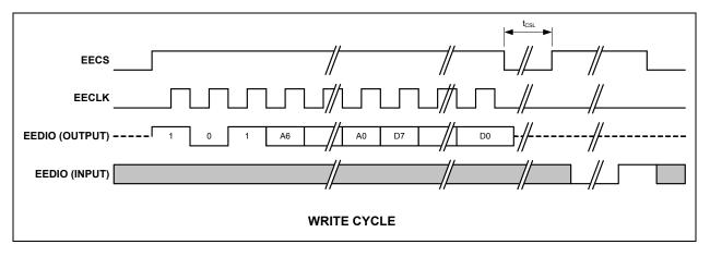
**WRAL (Write All):** If erase/write operations are enabled in the EEPROM, this command will cause the contents of the E2P\_DATA register to be written to every EEPROM memory location. The EPC\_TO bit is set if the EEPROM does not respond within 30 ms.
