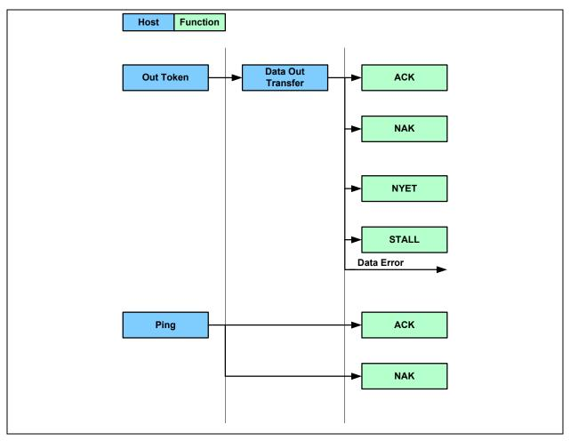
In the case where the Bulk-Out packet is errored, the URX does not respond to the host. The URX will request that the FCT rewinds the packet. It is the host's responsibility to retransmit the packet at a later time.
