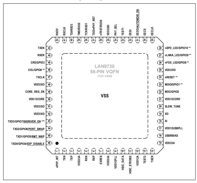
**Note:** \*\* This pin provides additional PME related functionality. Refer to the respective pin descriptions and Chapter 5.0, "PME Operation" for additional information.
