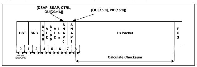
The RXCOE supports a maximum of two VLAN tags. If there are more than two VLAN tags, the VLAN protocol identifier for the third tag is treated as an Ethernet type field. The checksum calculation will begin immediately after the type field.
