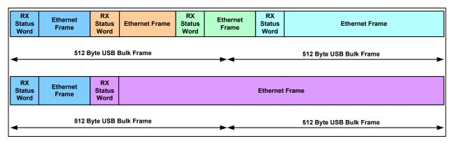
In accordance with the USB protocol, the UTX terminates a burst with either a ZLP or a Bulk-In packet with a size of less than the Bulk-In maximum packet size (512 bytes). The ZLP is needed when the total amount of data transmitted is a multiple of a Bulk-In packet size. The UTX monitors the RX FIFO size signal from the FCT to determine when a burst has ended.
