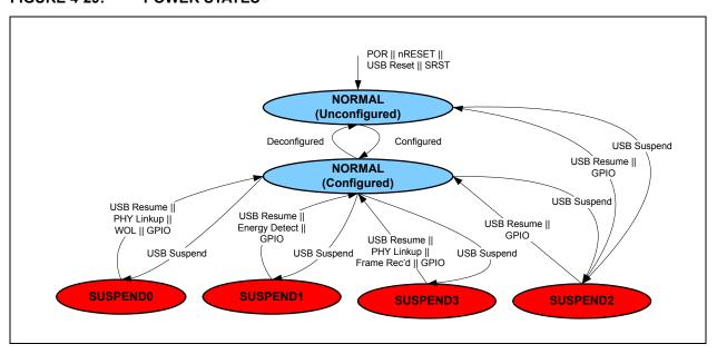
**Note:** It is not possible to transition from SUSPEND2 to NORMAL Configured if SUSPEND2 was entered via a transition from NORMAL Unconfigured.
