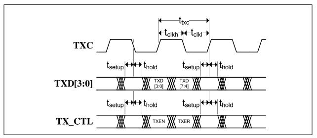
TABLE 7-16: RGMII TRANSMIT TIMING VALUES (TXC INTERNAL DELAY ENABLED)
