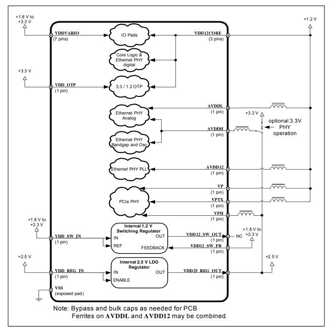
FIGURE 4-4: LAN7431 POWER CONNECTIVITY ON-CHIP REGULATORS DISABLED
