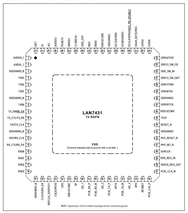
**Note:** Configuration straps are identified by an underlined symbol name. Signals that function as configuration straps must be augmented with an external resistor when connected to a load.
