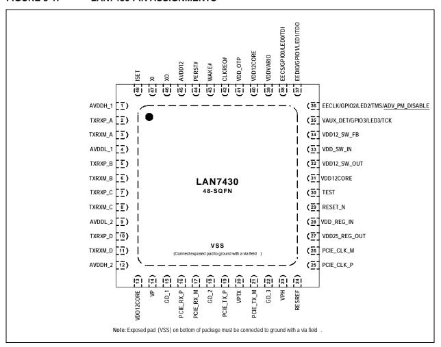
**Note:** Configuration straps are identified by an underlined symbol name. Signals that function as configuration straps must be augmented with an external resistor when connected to a load.
