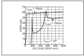
FIGURE 2-3: Power Supply Rejection Ratio vs. Voltage Drop.
