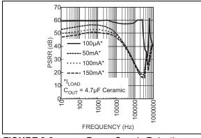
FIGURE 2-2: Power Supply Rejection Ratio.
