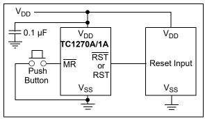
FIGURE 4-2: Typical Push-Pull Application Circuit.
