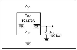
**FIGURE 5-9:** Ensuring a valid active-low Reset pin output state as V<sub>DD</sub> approaches 0V.
