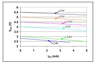
FIGURE 2-24: V<sub>OH</sub> vs. I<sub>OH</sub> (TC1270AR, TC1270ANR, TC1271AR - 2.55V min./2.63V typ./2.70V max.) @ +25°C).
