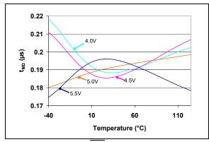
**FIGURE 2-39:** MR Low to Reset Propagation Delay  $(t_{MD})$  vs. Temperature (TC1270AR, TC1270ANR, TC1271AR - 2.55V min./2.63V typ./2.70V max.).
