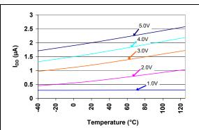
FIGURE 2-2: I<sub>DD</sub> vs. Temperature (Reset Power-up Timer Inactive) (TC1270AT, TC1270ANT, TC1271AT - 3.00V min./3.08V typ./3.15V max.).
