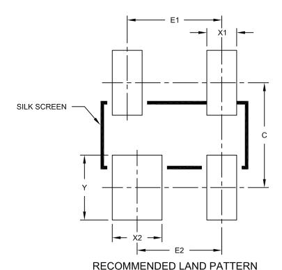
Units **MILLIMETERS** MAX **Dimension Limits** MIN NOM Contact Pitch 1.90 BSC E1 E2 1.60 BSC Contact Pitch 0.60 Contact Width X1 Contact Width X2 1.00 Contact Length 1.30 С 2.10 Contact Pad Spacing
