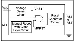
FIGURE 4-1: TC127XA High Level Block Diagram.
