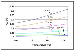
**FIGURE 2-20:**  $V_{\rm OL}$  vs. Temperature (TC1270AT, TC1270ANT, TC1271AT - 3.00V min./3.08V typ./3.15V max.). @  $V_{\rm DD}$  = 2.7V).
