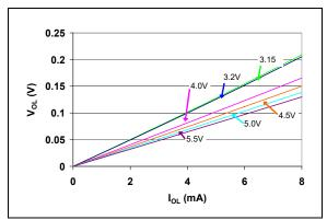
FIGURE 2-17: V<sub>OL</sub> vs. I<sub>OL</sub> (TC1270AT, TC1270ANT, TC1271AT - 3.00V min./3.08V typ./3.15V max.).
