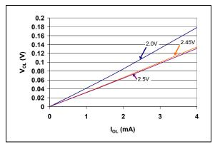
FIGURE 2-18: V<sub>OL</sub> vs. I<sub>OL</sub> (TC1270AR, TC1270ANR, TC1271AR - 2.55V min./2.63V typ./2.70V max.).
