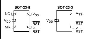
FIGURE 5-8: SOT-23 5-pin to 3-pin Comparison.
