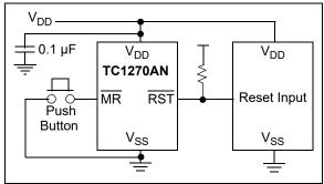
FIGURE 4-3: Typical Open-Drain Application Circuit.
