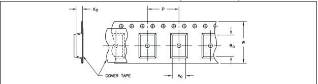
TABLE 1: CARRIER TAPE/CAVITY DIMENSIONS
