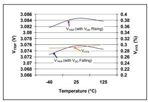
FIGURE 2-14:  $V_{TRIP}$  and  $V_{HYS}$  vs. Temperature (TC1270AT, TC1270ANT, TC1271AT - 3.00V min./3.08V typ./3.15V max.).
