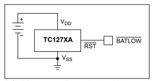
FIGURE 5-2: Battery Voltage Monitor.
