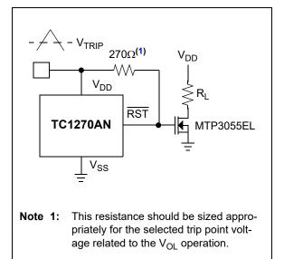
FIGURE 5-6: MOSFET Low-Drive Protection.
