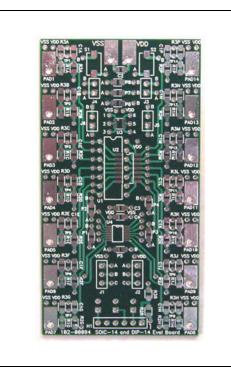
FIGURE 8-2: SOIC-14 Evaluation Board (Microchip Part Number SOIC14EV).
