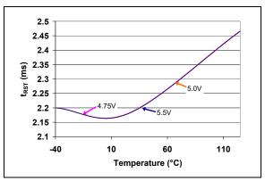
FIGURE 2-34: Reset Time-Out Period (t<sub>RST</sub>) (B time out option) vs. Temperature (TC1270AL, TC1270ANL, TC1271AL - 4.50V min./4.63V typ./4.75V max.).
