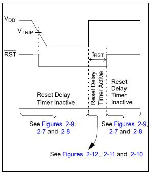
**FIGURE 4-12:** Reset Power-up Timer Waveform.
