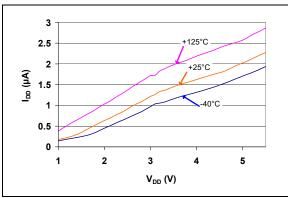
**FIGURE 2-8:**  $I_{DD}$  vs.  $V_{DD}$  (Reset Power-up Timer Inactive) (TC1270AT, TC1270ANT, TC1271AT - 3.00V min./3.08V typ./3.15V max.).
