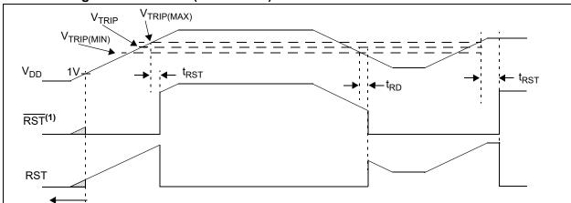
$V_{DD}$  < 1V is outside the device operating specification. The RST (or  $\overline{RST}$ ) output state is unknown while  $V_{DD}$  < 1V. **Note 1:** The TC1270AN requires an external pull-up resistor.
