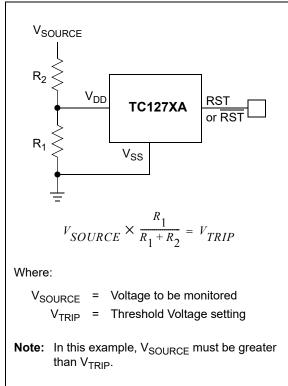
**FIGURE 5-5:** Modifying Trip-Point using External Resistor Divider.
