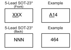
Note: Package marking code for MIC7211 is A14. Package marking code for MIC7221 is A15.
