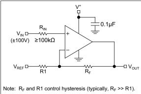
FIGURE 3-1: Driving the Input Beyond the Supply Rails.
