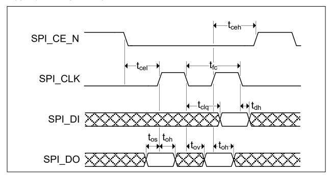
**Note:** The SPI can be configured for 30 MHz or 60 MHz operation via the <u>SPI\_SPD\_SEL</u> configuration strap. 30 MHz operation timing values are shown in Table 9-9. 60 MHz operation timing values are shown in Table 9-10.
