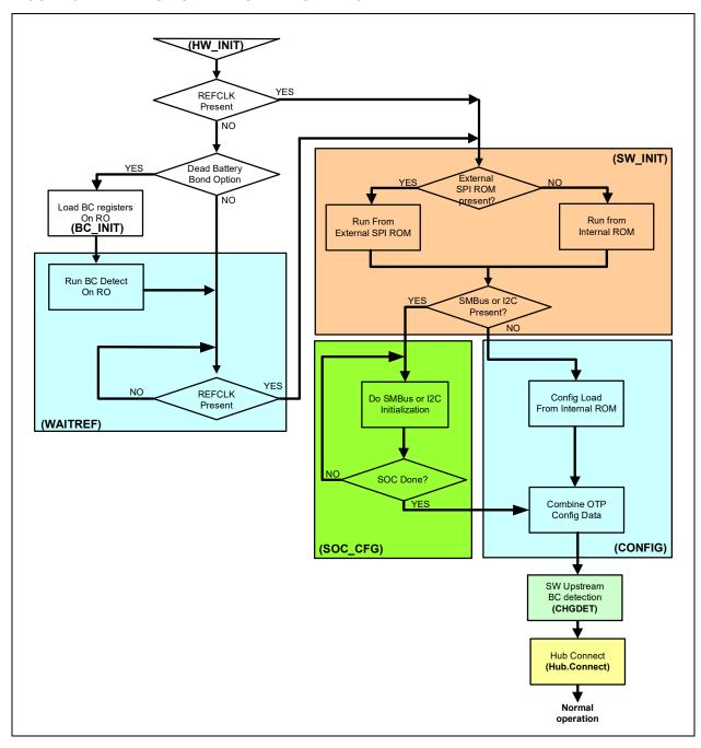
FIGURE 5-1: HUB OPERATIONAL MODE FLOWCHART
