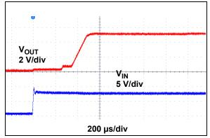
FIGURE 2-22: Start-Up From  $V_{IN}$ .
