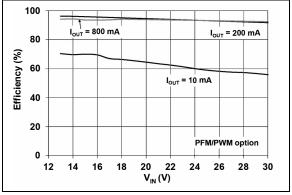
**FIGURE 2-6:** 12.0V  $V_{OUT}$  Efficiency vs.  $V_{IN}$ .
