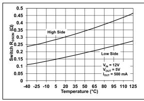
**FIGURE 2-9:** Switch  $R_{DSON}$  vs. Temperature.
