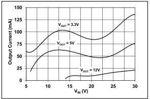
**FIGURE 2-17:** PFM/PWM  $I_{OUT}$  Threshold vs.  $V_{IN}$ .
