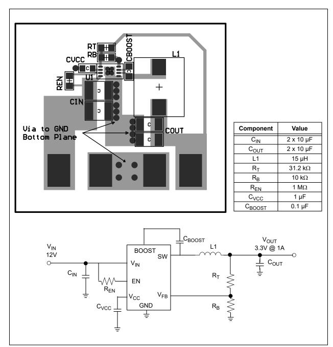
FIGURE 5-2: DFN Recommended Layout, 3.3V Output Design.
