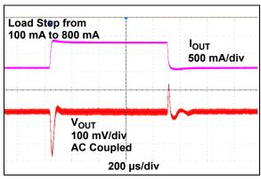
FIGURE 2-24: Load Transient Response.
