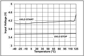
**FIGURE 2-10:** Undervoltage Lockout vs. Temperature.
