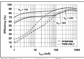
**FIGURE 2-2:** 5.0V  $V_{OUT}$  Efficiency vs.  $I_{OUT}$ .
