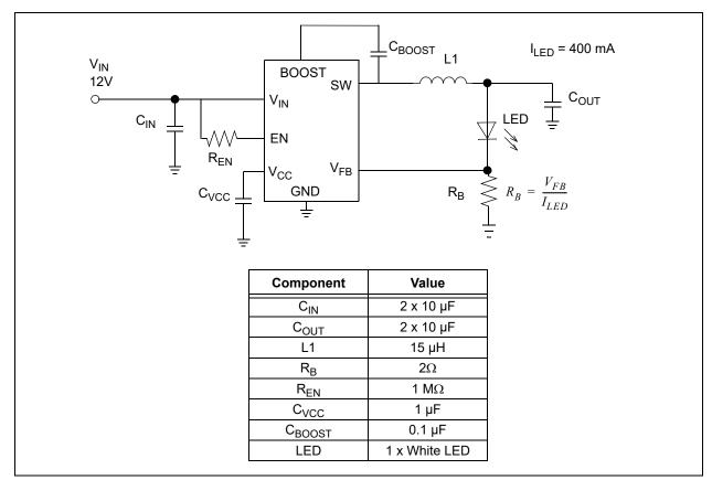
FIGURE 5-3: MCP16312 - Typical LED Driver Application: 400 mA Output.
