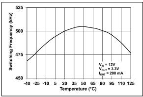
**FIGURE 2-20:** Switching Frequency vs. Temperature.
