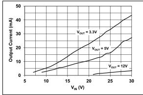
FIGURE 2-18: Skipping/PWM I<sub>OUT</sub> Threshold vs. Input Voltage.
