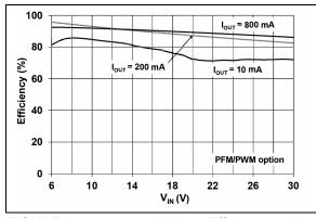
FIGURE 2-5: 5.0V V<sub>OUT</sub> Efficiency vs.V<sub>IN</sub>.
