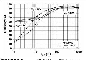
FIGURE 2-3: 12.0V V<sub>OUT</sub> Efficiency vs. I<sub>OUT</sub>.
