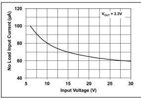
**FIGURE 2-15:** PFM No Load Input Current vs. Input Voltage, MCP16311.
