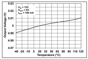
FIGURE 2-12: V<sub>OUT</sub> vs. Temperature.
