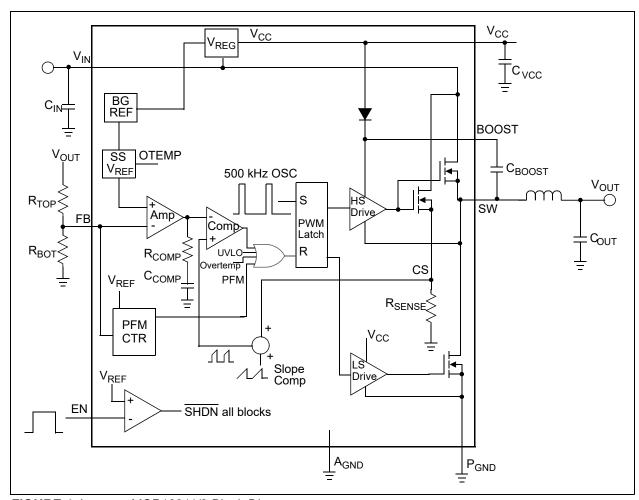
FIGURE 4-1: MCP16311/2 Block Diagram.
