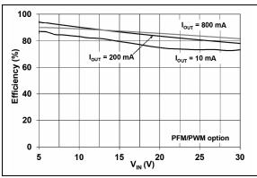
FIGURE 2-4: 3.3V  $V_{OUT}$  Efficiency vs.  $V_{IN}$ .
