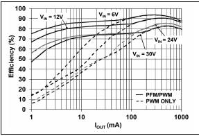
**FIGURE 2-1:** 3.3V  $V_{OUT}$  Efficiency vs.  $I_{OUT}$ .
