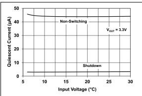
FIGURE 2-14: Input Quiescent Current vs. Input Voltage.
