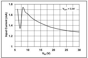
**FIGURE 2-16:** PWM No Load Input Current vs.V<sub>IN</sub>, MCP16312.
