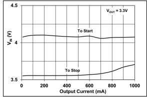
**FIGURE 2-19:** Typical Minimum Input Voltage vs. Output Current.
