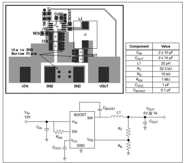
FIGURE 5-1: MSOP-8 Recommended Layout, 5V Output Design.
