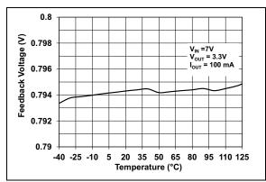
**FIGURE 2-8:**  $V_{FB}$  vs. Temperature;  $V_{OUT} = 3.3V$ .
