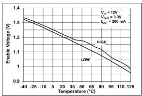
**FIGURE 2-11:** Enable Threshold Voltage vs. Temperature.
