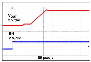
FIGURE 2-21: Start-Up From Enable.
