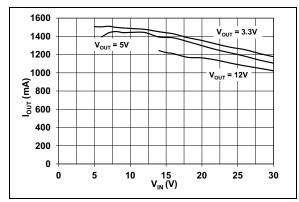
FIGURE 2-7:  $Max I_{OUT} vs. V_{IN.}$
