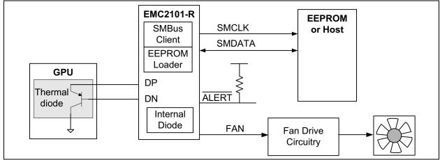
FIGURE 4-2: System Diagram for EMC2101-R.
