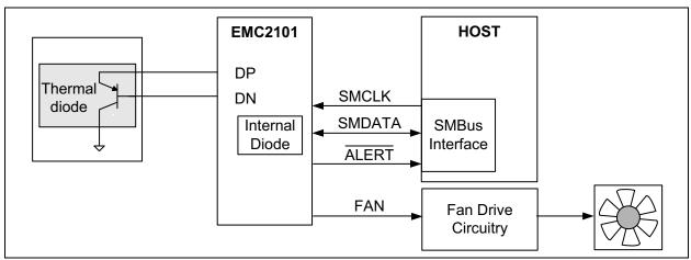
FIGURE 4-1: System Diagram for EMC2101.
