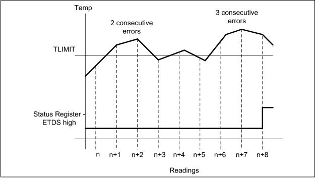
FIGURE 4-8: Example Fault Queue Response.
