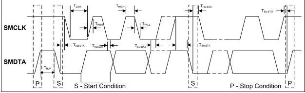
FIGURE 2-1: SMBus Timing Diagram.
