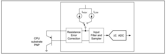
FIGURE 4-3: Block Diagram of Temperature Monitoring Circuit.
