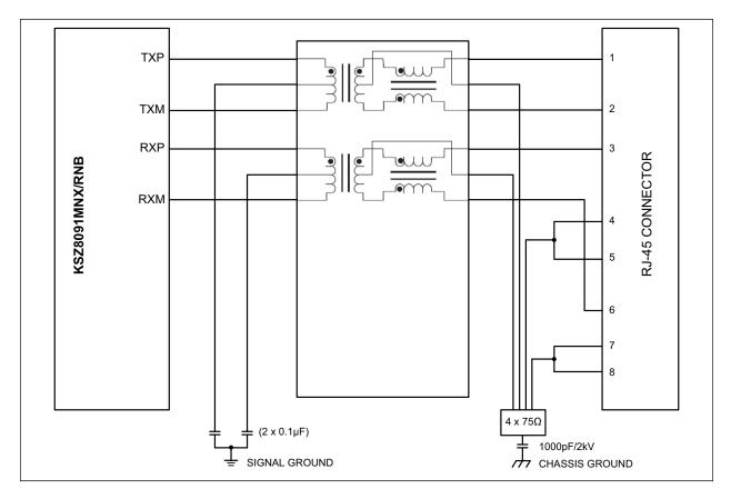
FIGURE 11-1: TYPICAL MAGNETIC INTERFACE CIRCUIT
