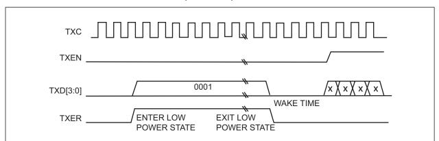
Similarly, the KSZ8091RNB enters LPI mode for the transmit direction when its attached EEE-compliant RMII MAC deasserts TXEN and sets TXD [1:0] to 01. The KSZ8091RNB remains in the LPI transmit state while the RMII MAC maintains the states of these signals. When the RMII MAC changes any of the TXEN or TX data signals from their LPI state values, the KSZ8091RNB exits the LPI transmit state.
