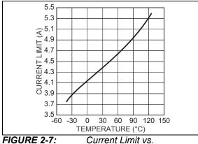
FIGURE 2-7: Current L Temperature.
