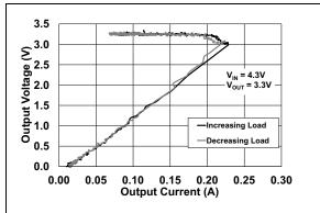
**FIGURE 2-30:** Short-Circuit Current Foldback.
