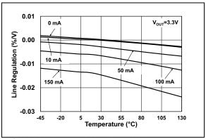
**FIGURE 2-22:** Line Regulation vs. Temperature.
