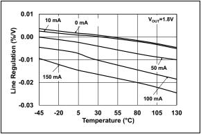
**FIGURE 2-21:** Line Regulation vs. Temperature.
