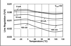
**FIGURE 2-23:** Line Regulation vs. Temperature.
