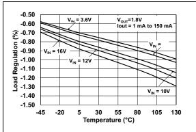
FIGURE 2-18: Load Regulation vs. Temperature.
