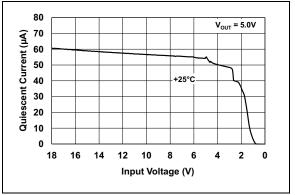
**FIGURE 2-6:** Quiescent Current vs. Input Voltage.
