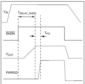
FIGURE 4-3: Power Good Timing from Shutdown.
