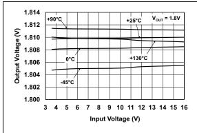
FIGURE 2-7: Output Voltage vs. Input Voltage.
