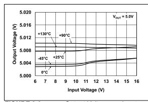
FIGURE 2-9: Output Voltage vs. Input Voltage.
