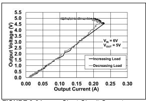
FIGURE 2-31: Short-Circuit Current Foldback.
