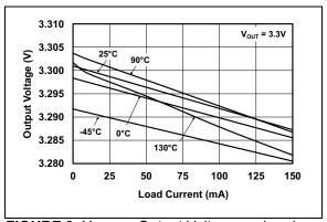
FIGURE 2-11: Output Voltage vs. Load Current.
