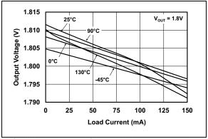
FIGURE 2-10: Output Voltage vs. Load Current.
