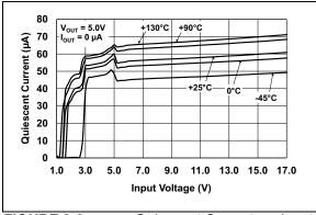
**FIGURE 2-3:** Quiescent Current vs. Input Voltage.
