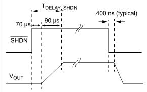
FIGURE 4-4: Shutdown Input Timing Diagram.
