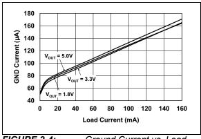
FIGURE 2-4: Ground Current vs. Load Current.
