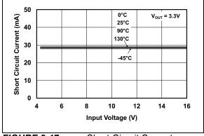
FIGURE 2-17: Short-Circuit Current vs. Input Voltage.
