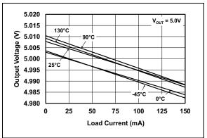
FIGURE 2-12: Output Voltage vs. Load Current.
