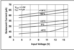
FIGURE 2-2: Quiescent Current vs. Input Voltage.
