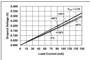
FIGURE 2-14: Dropout Voltage vs. Load Current.
