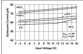
FIGURE 2-1: Quiescent Current vs. Input Voltage.
