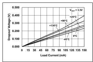
FIGURE 2-13: Dropout Voltage vs. Load Current.
