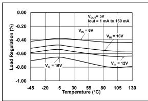
**FIGURE 2-20:** Load Regulation vs. Temperature.
