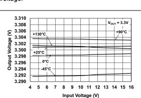
FIGURE 2-8: Output Voltage vs. Input Voltage.
