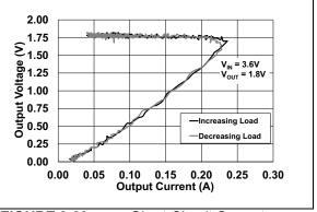
FIGURE 2-29: Short-Circuit Current Foldback.
