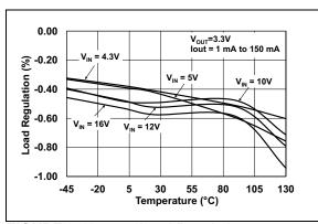
**FIGURE 2-19:** Load Regulation vs. Temperature.
