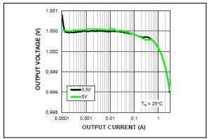
**FIGURE 2-10:** Buck Output Voltage (1.0V) vs. Output Current.
