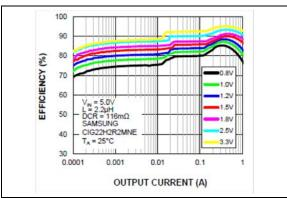
FIGURE 2-8: Buck Efficiency (LDCR = 116 mΩ) vs. Output Current.
