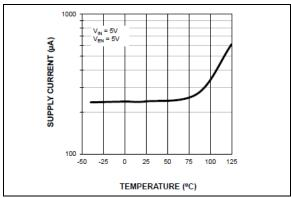
**FIGURE 2-17:** V<sub>IN</sub> Supply Current vs. Temperature.
