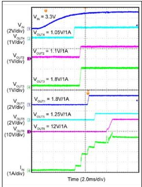
FIGURE 2-46: Input Supply Inrush Current – Loaded.
