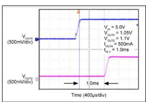
FIGURE 2-25: Standard Delay.
