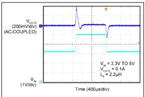
FIGURE 2-37: Boost 6 Line Transient – 3.3V to 5.0V.
