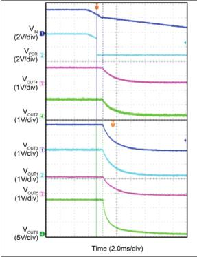
FIGURE 4-11: Hot Unplug – V<sub>IN</sub> Falling.
