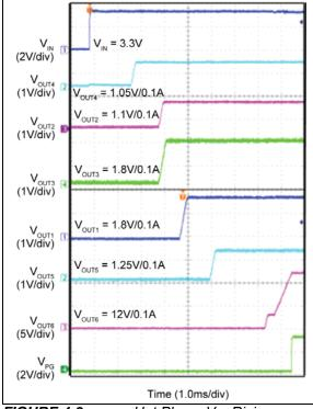
**FIGURE 4-9:** Hot Plug – V<sub>IN</sub> Rising.
