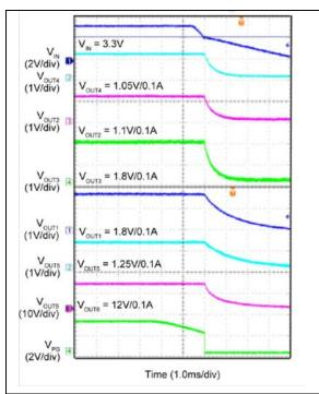
**FIGURE 2-21:** Unplug – Falling  $V_{IN}$ .
