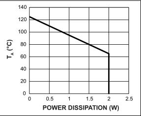
FIGURE 4-17: Power Derating Curve.
