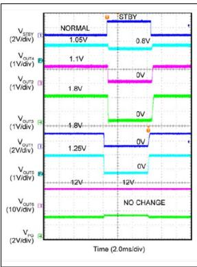
FIGURE 2-48: Rising Edge Trigger Standby.
