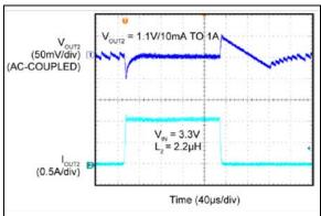
FIGURE 2-28: Buck 2 Load Transient – 10 mA to 1A.
