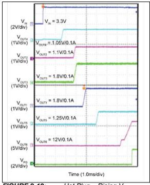
**FIGURE 2-19:** Hot Plug – Rising  $V_{IN}$ .
