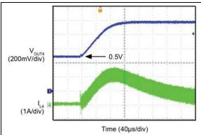
FIGURE 4-15: Pre-Biased Output Voltage.
