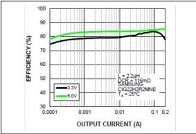
FIGURE 2-3: Boost Efficiency (12V) vs. Output Current.
