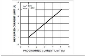
**FIGURE 2-18:** Programmed Current-Limit vs. Measured Current-Limit.
