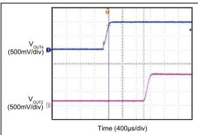
FIGURE 4-8: Standard Delay Time.
