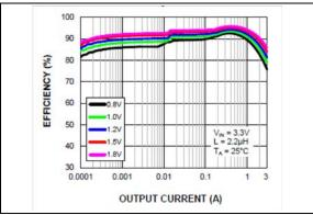
**FIGURE 2-1:** Buck Efficiency (LDCR =  $0 \text{ m}\Omega$ ) vs. Output Current.
