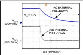
FIGURE 2-27: Output Pull-Down Resistance.
