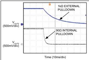
FIGURE 4-13: Output Pull-Down Resistance.
