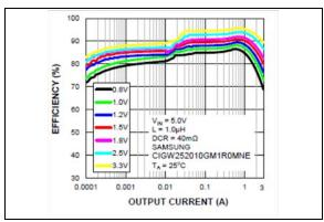
**FIGURE 2-5:** Buck Efficiency (LDCR =  $40 \text{ m}\Omega$ ) vs. Output Current.
