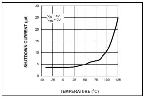
**FIGURE 2-16:** V<sub>IN</sub> Shutdown Supply Current vs. Temperature.
