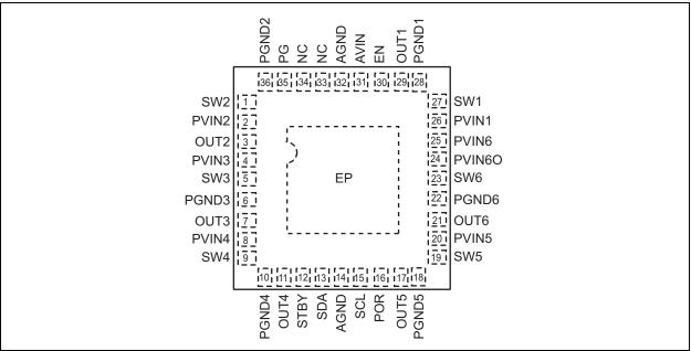
FIGURE 3-1: MIC7401 Pin Configuration.
