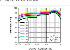
**FIGURE 2-2:** Buck Efficiency (LDCR =  $0 \text{ m}\Omega$ ) vs. Output Current.
