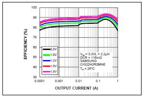
**FIGURE 2-7:** Buck Efficiency (LDCR =  $116 \text{ m}\Omega$ ) vs. Output Current.
