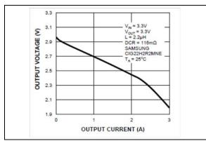
**FIGURE 2-13:** Dropout Output Voltage vs. Output Current.
