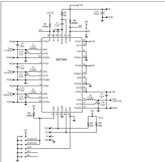
FIGURE 6-1: Connections for Unused Pins.
