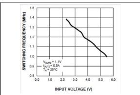
FIGURE 2-15: Buck 2 Switching Frequency vs. Input Voltage.
