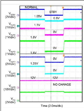
**FIGURE 2-47:** Falling Edge Trigger Standby (DEFAULT).
