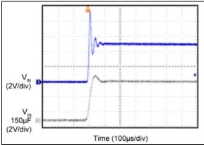
FIGURE 4-18: Hot Plug Input Voltage Spike.
