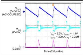
FIGURE 2-40: Buck 2 PFM Switching Waveforms.
