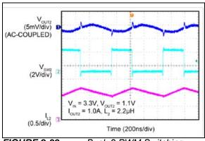
FIGURE 2-39: Buck 2 PWM Switching Waveforms.
