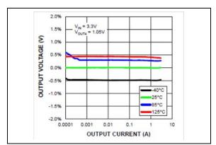
FIGURE 2-6: Output Voltage vs. Output Current.
