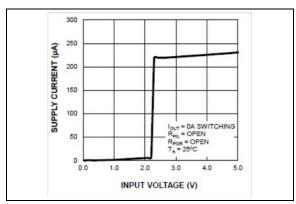
**FIGURE 2-14:**  $V_{IN}$  Operating Supply Current vs. Input Voltage.
