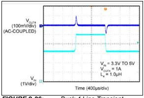
FIGURE 2-36: Buck 4 Line Transient – 3.3V to 5.0V.
