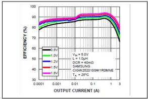
**FIGURE 2-4:** Buck Efficiency (LDCR =  $40 \text{ m}\Omega$ ) vs. Output Current.
