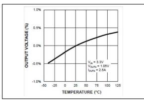
**FIGURE 2-9:** Output Voltage vs. Temperature.
