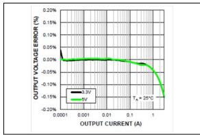
FIGURE 2-11: Buck Output Voltage Regulator vs. Output Current.
