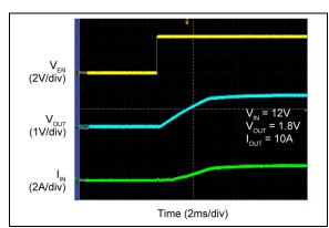
FIGURE 2-24: Enable Turn-On Delay and Rise Time.
