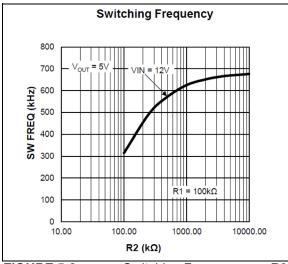
FIGURE 5-2: Switching Frequency vs. R2.
