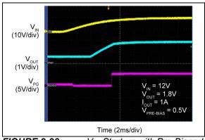
**FIGURE 2-26:** V<sub>IN</sub> Start-up with Pre-Biased Output.
