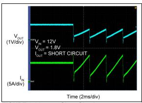
FIGURE 2-30: Short Circuit.
