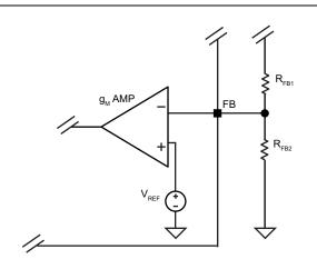
FIGURE 5-3: Voltage/Divider Configuration.
