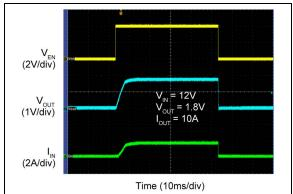
FIGURE 2-27: Enable Turn-On/Off.
