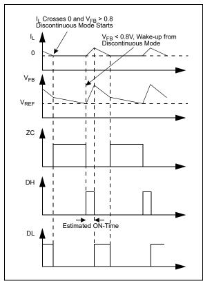
FIGURE 4-4: MIC45208-1 Control Loop Timing (Discontinuous Mode).
