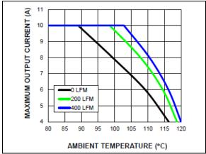
**FIGURE 5-6:** MIC45208 Power Derating vs. Airflow (5  $V_{IN}$  to 1.5  $V_{OLIT}$ ).
