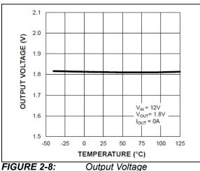
FIGURE 2-8: vs. Temperature.
