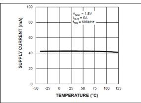
**FIGURE 2-2:** V<sub>IN</sub> Operating Supply Current vs. Temperature (MIC45208-2).
