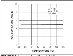
**FIGURE 2-4:** V<sub>DD</sub> Supply Voltage vs. Temperature.
