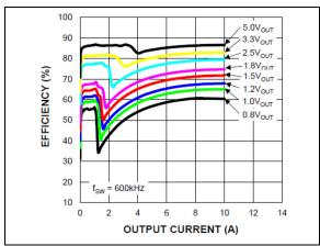
**FIGURE 2-13:** Efficiency  $(V_{IN} = 24V)$  vs. Output Current (MIC45208-1).
