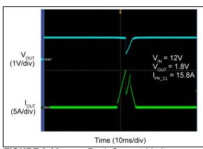
FIGURE 2-32: Peak Current-Limit Threshold.
