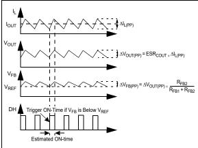
FIGURE 4-2: MIC45208 Control Loop Timing.
