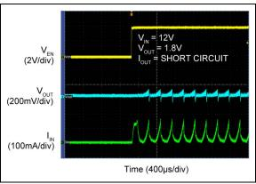
FIGURE 2-29: Enabled into Short Circuit.
