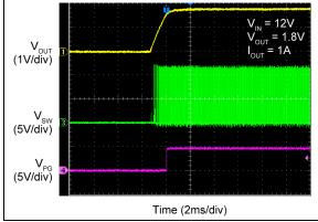
FIGURE 2-33: Output Recovery from Thermal Shutdown.
