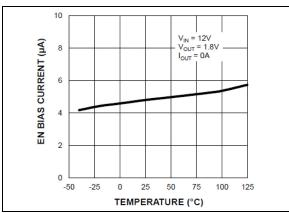
FIGURE 2-6: EN Bias Current vs. Temperature.
