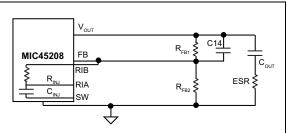
FIGURE 5-5: FB via RIB Pin.
