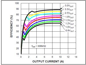
**FIGURE 2-16:** Efficiency  $(V_{IN} = 24V)$  vs. Output Current (MIC45208-2).
