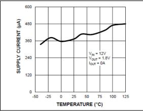
**FIGURE 2-1:** V<sub>IN</sub> Operating Supply Current vs. Temperature (MIC45208-1).
