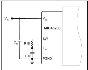
FIGURE 4-5: MIC45208 Current-Limiting Circuit.
