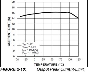
**FIGURE 2-10:** vs. Temperature.
