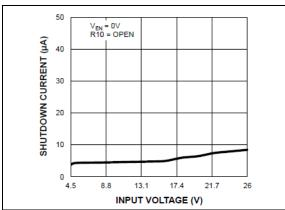
**FIGURE 2-3:** V<sub>IN</sub> Shutdown Current vs. Input Voltage.
