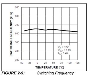
FIGURE 2-9: vs. Temperature.
