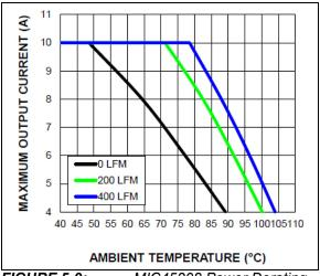
**FIGURE 5-9:** MIC45208 Power Derating vs. Airflow (24 V<sub>IN</sub> to 1.5 V<sub>OUT</sub>).
