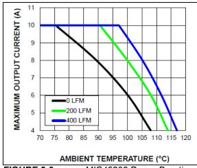
FIGURE 5-8: MIC45208 Power Derating vs. Airflow (12 V<sub>IN</sub> to 3.3 V<sub>OUT</sub>).
