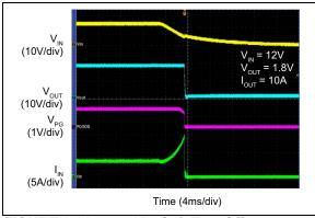
FIGURE 2-23: V<sub>IN</sub> Soft Turn-Off.
