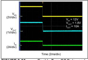
FIGURE 2-25: Enable Turn-Off Delay and Fall Time.
