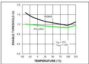
FIGURE 2-5: Enable Threshold vs. Temperature.
