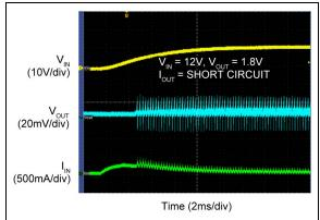
FIGURE 2-28: Power-up into Short Circuit.
