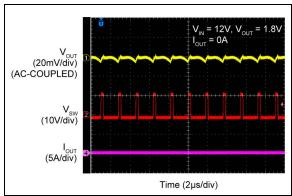
**FIGURE 2-35:** Waveforms.
