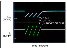
FIGURE 2-31: Output Recovery from Short Circuit.
