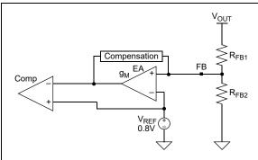
FIGURE 4-1: Output Voltage Sense via FB Pin.
