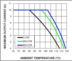
**FIGURE 5-7:** MIC45208 Power Derating vs. Airflow (12 V<sub>IN</sub> to 1.5 V<sub>OUT</sub>).
