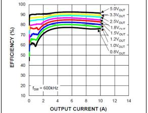
**FIGURE 2-12:** Efficiency (V<sub>IN</sub> = 12V) vs. Output Current (MIC45208-1).
