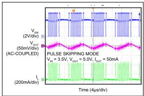
**FIGURE 2-16:** Output Ripple (Pulse Skipping Mode).
