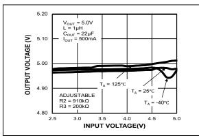
**FIGURE 2-3:** Output Voltage vs. Input Voltage.
