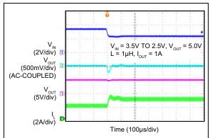
**FIGURE 2-13:** Line Transient (3.5V to 2.5V).
