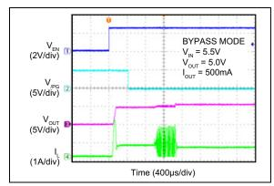
FIGURE 2-19: Soft-Start Bypass Mode.
