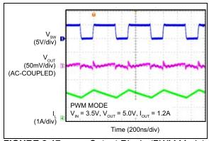
FIGURE 2-17: Output Ripple (PWM Mode).
