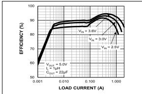
FIGURE 2-1: Efficiency vs. Load Current.
