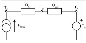
FIGURE 7-2: Series Thermal Resistance Circuit.
