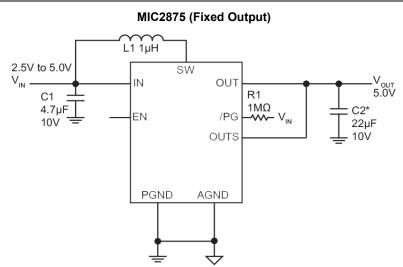
$^{\star}$  Two more 22  $\mu F$  capacitors should be added in parallel with C2 for  $V_{\text{IN}}$  > 5.0V.
