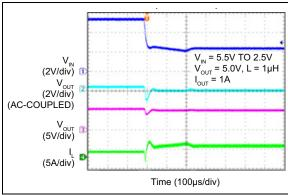
**FIGURE 2-15:** Line Transient (5.5V to 2.5V).
