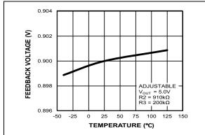
FIGURE 2-6: Feedback Voltage vs. Temperature.
