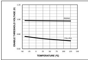
FIGURE 2-8: Enable Threshold vs. Temperature.
