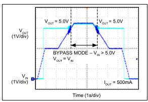
FIGURE 2-23: Bypass Mode.
