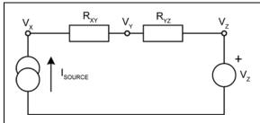
FIGURE 7-1: Series Electrical Resistance Circuit.
