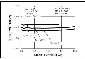
FIGURE 2-2: Output Voltage vs. Load Current.
