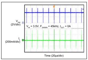
FIGURE 2-20: Minimum Switching.
