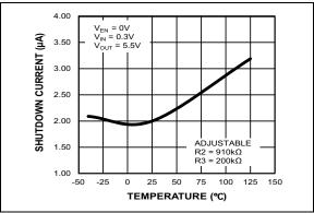
**FIGURE 2-5:** Output Shutdown Current vs. Temperature.
