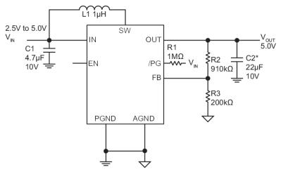
$^{\star}$  Two more 22  $\mu\text{F}$  capacitors should be added in parallel with C2 for  $V_{\text{IN}}$  > 5.0V.
