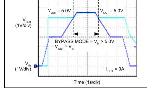
FIGURE 2-22: Bypass Mode.
