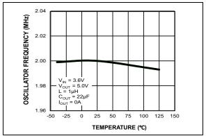
**FIGURE 2-4:** Oscillator Frequency vs. Temperature.
