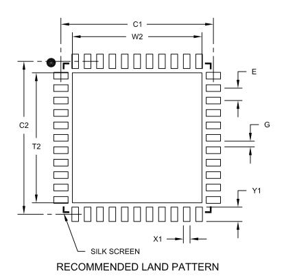
**MILLIMETERS** Units **Dimension Limits** MIN MOM MAX Contact Pitch Ε 0.65 BSC Optional Center Pad Width W2 6.80 Optional Center Pad Length T2 6.80 Contact Pad Spacing C1 8.00 Contact Pad Spacing C2 8.00 Contact Pad Width (X44) X1 0.35 Contact Pad Length (X44) Y1 0.80 Distance Between Pads 0.25 G
