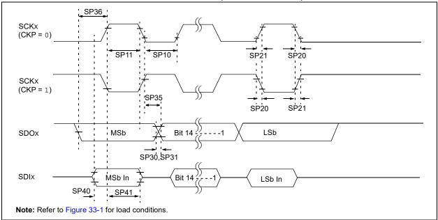
TABLE 33-31: SPIX MODULE MASTER MODE (CKE = 1, SMP = 1) TIMING REQUIREMENTS
