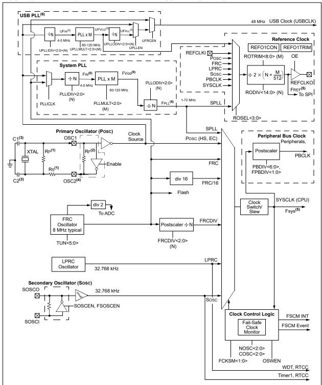
Notes: 1. A series resistor, Rs, may be required for AT strip cut crystals, or to eliminate clipping. Alternately, to increase oscillator circuit gain, add a parallel resistor, RP, with a value of 1 MΩ.
