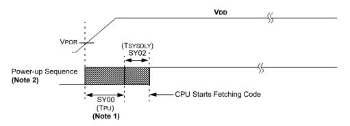
Internal Voltage Regulator Enabled Clock Sources = (HS, HSPLL, XT, XTPLL and Sosc)
