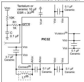
Note 1: If the USB module is not used, this pin must be connected to VDD.
