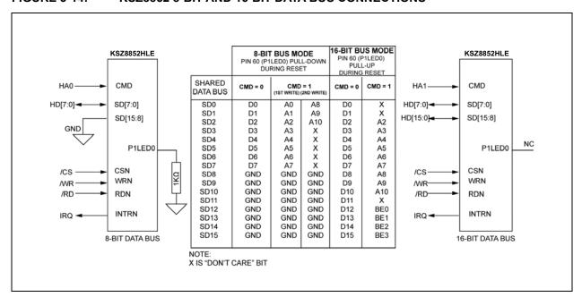
FIGURE 3-14: KSZ8852 8-BIT AND 16-BIT DATA BUS CONNECTIONS
