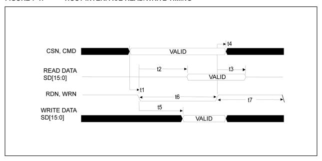
TABLE 7-1: HOST INTERFACE READ/WRITE TIMING PARAMETERS
