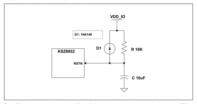
Figure 7-6 is the recommended reset circuit for applications where reset is driven by another device (e.g., CPU or FPGA). At power-on-reset, R, C and D1 provide the necessary ramp rise time to reset the KSZ8852 device. The RST\_OUT\_N from CPU/FPGA provides the warm reset after power up.
