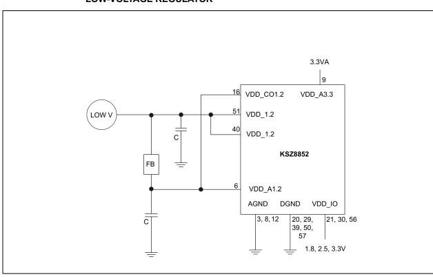
FIGURE 3-11: RECOMMENDED LOW-VOLTAGE POWER CONNECTION USING AN EXTERNAL LOW-VOLTAGE REGULATOR
