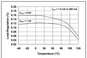
FIGURE 2-17: Load Regulation vs. Temperature ( $V_{OUT}$  < 2.5V Fixed).
