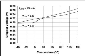
FIGURE 2-20: Dropout Voltage vs. Temperature.
