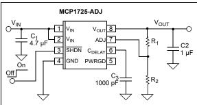
FIGURE 4-1: Typical Adjustable Output Voltage Application Circuit.
