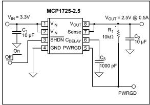
FIGURE 5-1: Typical Application Circuit.
