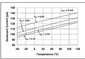
FIGURE 2-3: Quiescent Current vs. Junction Temperature (1.8V Adjustable).
