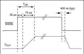
FIGURE 4-5: Shutdown Input Timing Diagram.
