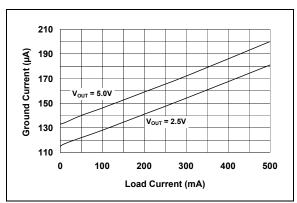
FIGURE 2-12: Ground Current vs. Load Current.
