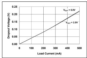
FIGURE 2-19: Dropout Voltage vs. Load Current.
