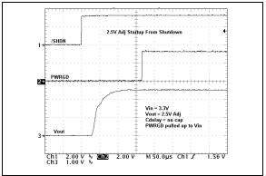
**FIGURE 2-28:** 2.5V (Adj.) Startup from Shutdown.
