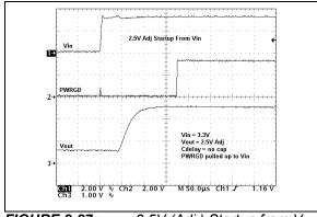
FIGURE 2-27: 2.5V (Adj.) Startup from V<sub>IN</sub>.
