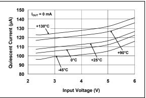
FIGURE 2-10: Quiescent Current vs. Input Voltage (0.8V Fixed).
