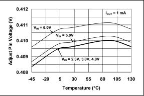
FIGURE 2-6: Adjust Pin Voltage vs. Temperature.
