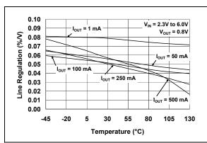
**FIGURE 2-15:** Line Regulation vs. Temperature (0.8V Fixed).
