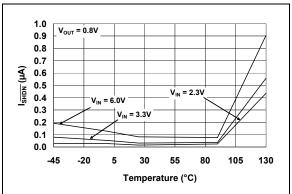
FIGURE 2-14: I<sub>SHDN</sub> vs. Temperature.
