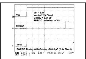
**FIGURE 2-30:** Power Good (PWRGD) Timing with  $C_{DELAY}$  of 0.01  $\mu$ F (2.5V Fixed).
