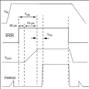
FIGURE 4-3: Power Good Timing from Shutdown.
