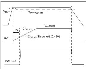
**FIGURE 4-4:** C<sub>DELAY</sub> and PWRGD Timing Diagram.
