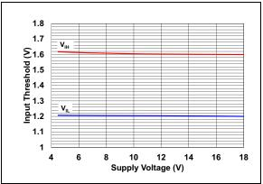
FIGURE 2-16: Input Threshold vs. Supply Voltage.
