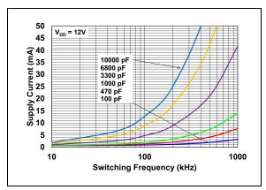
**FIGURE 2-25:** Supply Current vs. Frequency  $(V_{DD} = 12V)$ .
