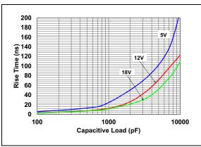
FIGURE 2-2: Rise Time vs. Capacitive Load.
