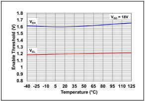
**FIGURE 2-17:** Enable Threshold vs. Temperature.
