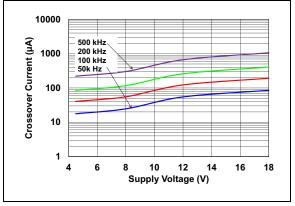
**FIGURE 2-6:** Crossover Current vs. Supply Voltage.
