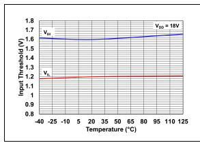
**FIGURE 2-15:** Input Threshold vs. Temperature.
