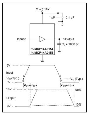
**FIGURE 4-2:** Non-Inverting Driver Timing Waveform.
