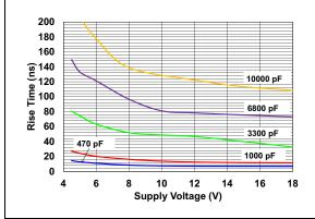
**FIGURE 2-1:** Rise Time vs. Supply Voltage.
