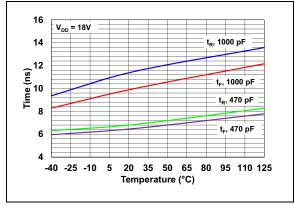
**FIGURE 2-5:** Rise and Fall Time vs. Temperature.
