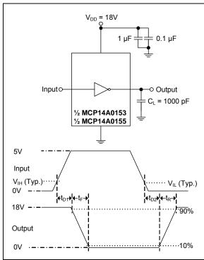
FIGURE 4-1: Inverting Driver Timing Waveform.
