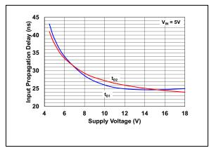
**FIGURE 2-7:** Input Propagation Delay vs. Supply Voltage.
