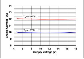
FIGURE 2-27: Enable Current vs. Supply Voltage.
