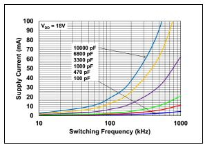
**FIGURE 2-24:** Supply Current vs. Frequency ( $V_{DD} = 18V$ ).
