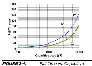
FIGURE 2-4: Fall Time vs. Capacitive Load.
