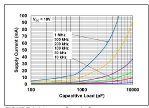
**FIGURE 2-21:** Supply Current vs. Capacitive Load ( $V_{DD} = 18V$ ).
