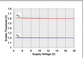
FIGURE 2-18: Enable Threshold vs. Supply Voltage.
