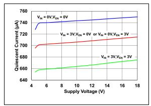
**FIGURE 2-13:** Quiescent Supply Current vs. Supply Voltage.
