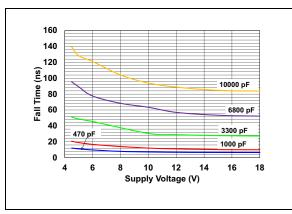
**FIGURE 2-3:** Fall Time vs. Supply Voltage.
