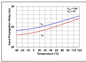
**FIGURE 2-9:** Input Propagation Delay vs. Temperature.
