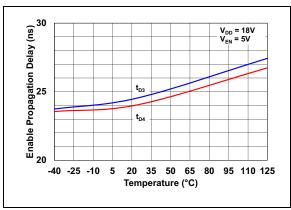
**FIGURE 2-12:** Enable Propagation Delay vs. Temperature.
