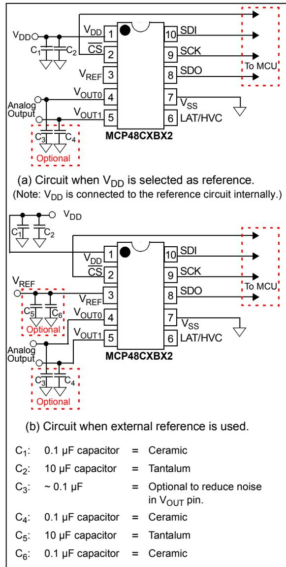
**FIGURE 8-1:** Example Circuit.
