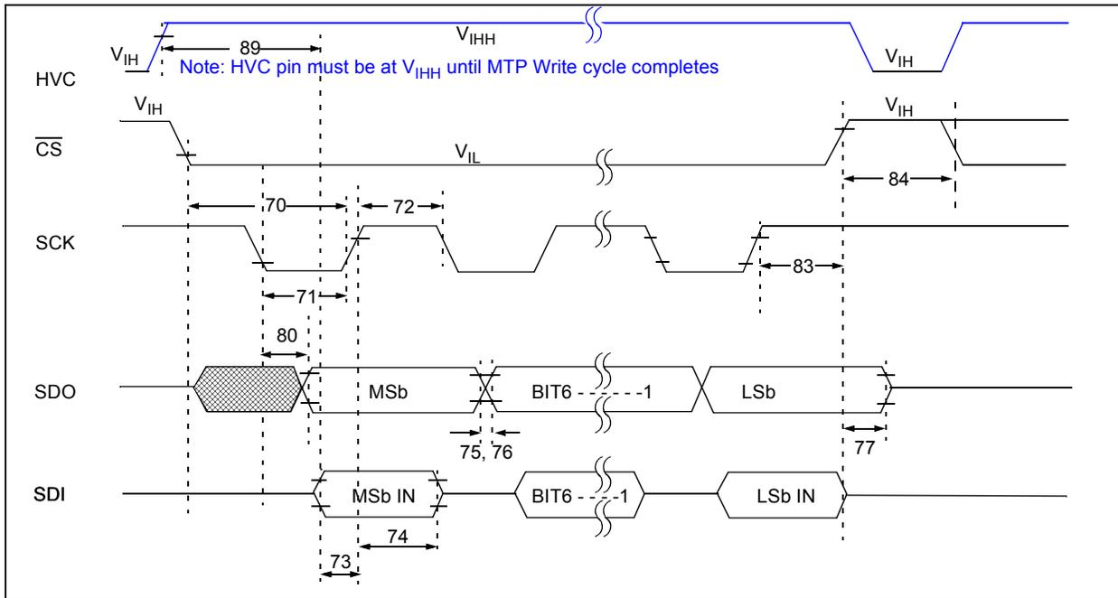
**FIGURE 1-5:** SPI Timing Waveform (Mode = '11').
