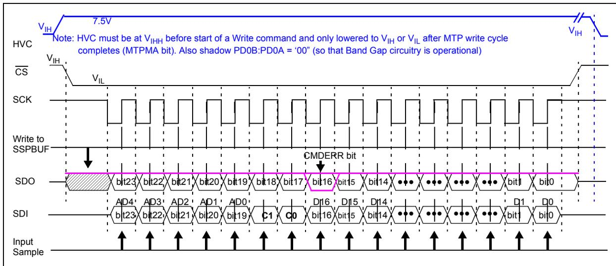
**FIGURE 6-3:** 24-Bit Commands (Write, Read) - SPI Waveform (Mode 1,1).
