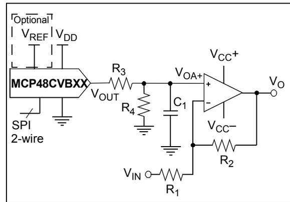
**FIGURE 8-4:** Digitally-Controlled Bipolar Voltage Source Example Circuit.
