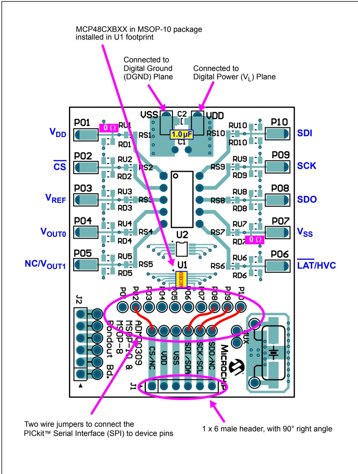
**FIGURE 9-1:** MCP48CXBXX Evaluation Board Circuit Using ADM00309.
