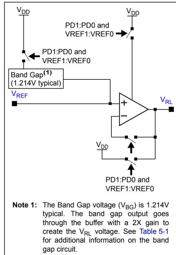
**Note 1:** The Band Gap voltage (V<sub>BG</sub>) is 1.214V typical. The band gap output goes through the buffer with a 2X gain to create the V<sub>RL</sub> voltage. See Table 5-1 for additional information on the band gap circuit.
