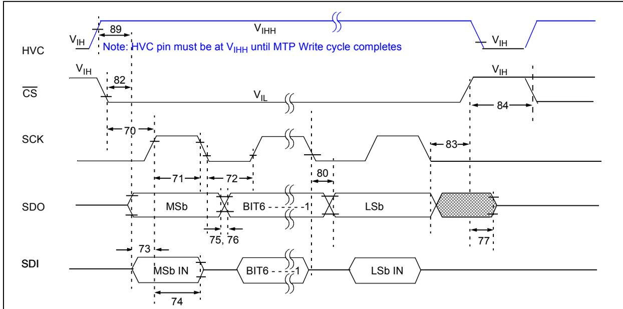
**FIGURE 1-6:** SPI Timing Waveform (Mode = 00).
