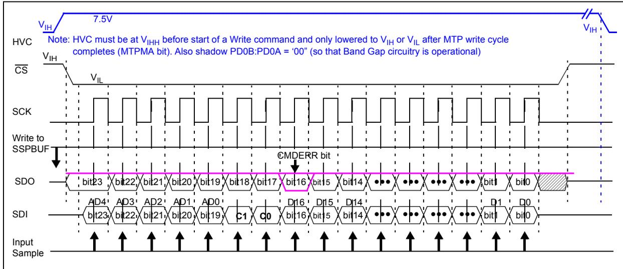
**FIGURE 6-2:** 24-Bit Commands (Write, Read) - SPI Waveform (Mode 0,0).
