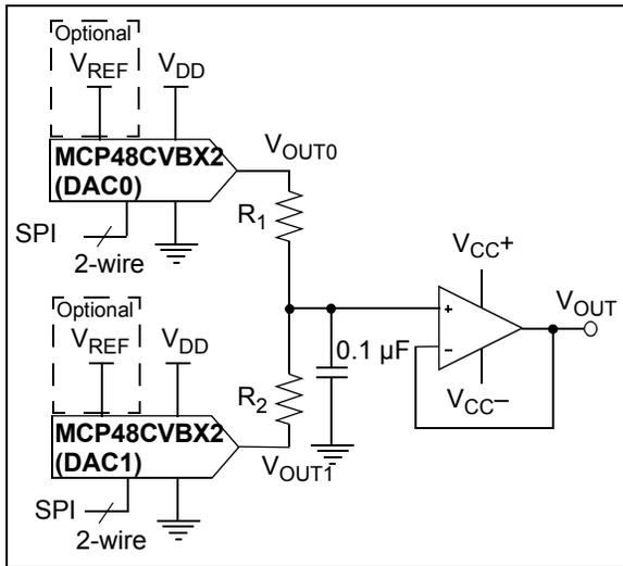
**FIGURE 8-6:** Simple Double Precision DAC Using MCP48CVBX2.
