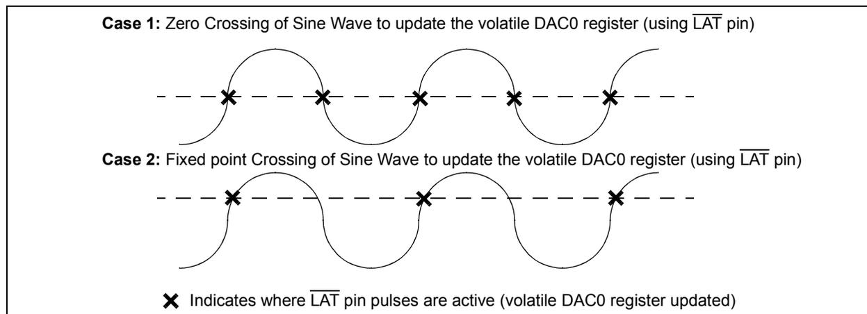
**FIGURE 5-9:** Example Use of  $\overline{\text{LAT}}$  Pin Operation.
