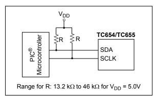
FIGURE 7-1: Pull-Up Resistors On SMBus.
