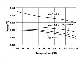
FIGURE 2-9:  $V_{CMIN}$  vs. Temperature.
