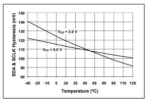
**FIGURE 2-12:** SDA, SCLK Hysteresis vs. Temperature.
