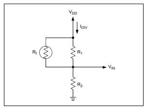
**FIGURE 7-3:** Temperature Sensing Circuit.
