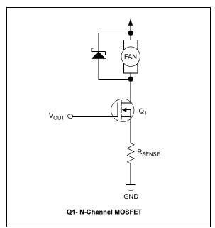
**FIGURE 7-8:** Clamp Diode For Fan Turn-Off.
