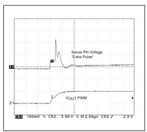
FIGURE 7-10: Extra Pulse at Sense Pin.
