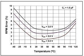
**FIGURE 2-10:** RPM % error vs. Temperature.
