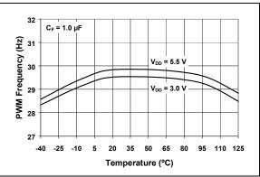
FIGURE 2-6: PWM Frequency vs. Temperature.
