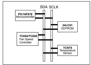
FIGURE 7-2: Multiple Devices on SMBus.
