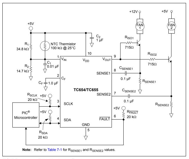
FIGURE 4-1: Typical Application Circuit.
