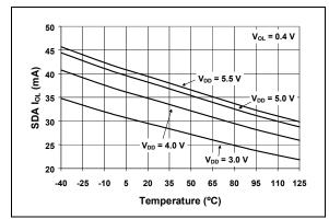
FIGURE 2-7: SDA I<sub>OL</sub> vs. Temperature.
