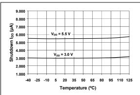
**FIGURE 2-2:** I<sub>DD</sub> Shutdown vs. Temperature.
