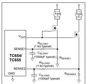
**FIGURE 7-12:** FET Drive with  $R_{SLOW}/C_{SLOW}$  Sense Scheme.
