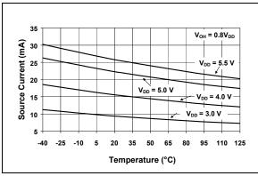
**FIGURE 2-3:** PWM, Source Current vs. Temperature.
