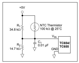
FIGURE 4-6: NTC Thermistor Sensor Network.
