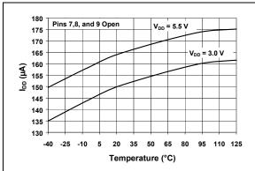
FIGURE 2-1: I<sub>DD</sub> vs. Temperature.
