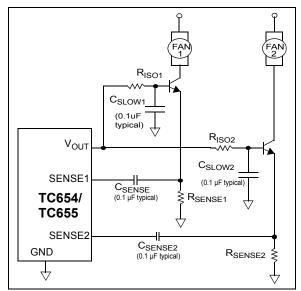
**FIGURE 7-11:** Transistor Drive with  $C_{SLOW}$  Capacitor.
