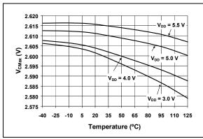
FIGURE 2-8: V<sub>CMAX</sub> vs. Temperature.
