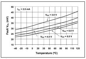
FIGURE 2-5: Fault V<sub>OL</sub> vs. Temperature.
