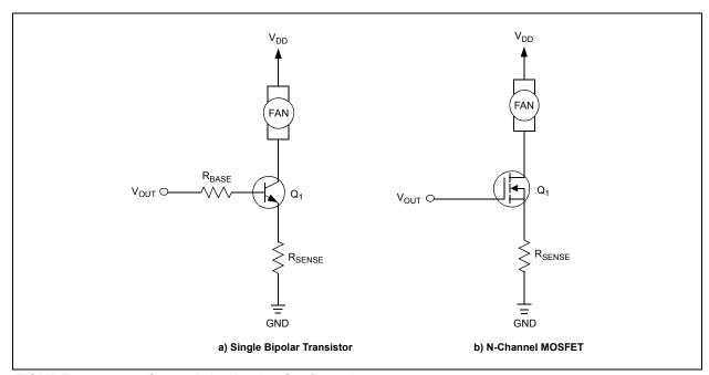
FIGURE 7-7: Output Drive Device Configurations.
