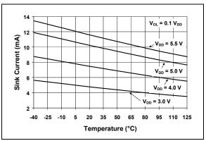
**FIGURE 2-4:** PWM, Sink Current vs. Temperature.
