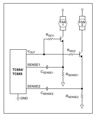
FIGURE 4-7: Fan Current Sensing.
