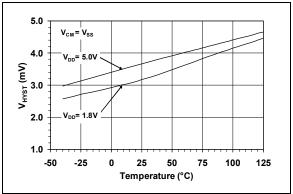
**FIGURE 2-10:** Input Hysteresis Voltage vs. Temperature.
