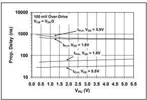
FIGURE 2-36:Propagation Delay vs.Pull-up Voltage.
