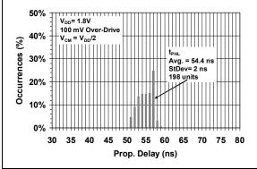
FIGURE 2-25: High-to-Low Propagation Delays.
