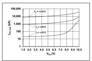
**FIGURE 2-23:** Output Leakage Current vs. Pull-up Voltage.
