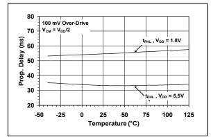
**FIGURE 2-29:** Propagation Delay vs. Temperature.
