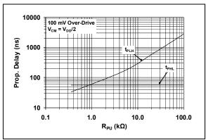
*FIGURE 2-35:* Propagation Delay vs. Pull-up Resistor.
