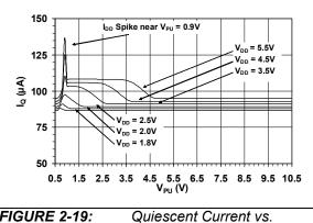
FIGURE 2-19: Pull-up Voltage.
