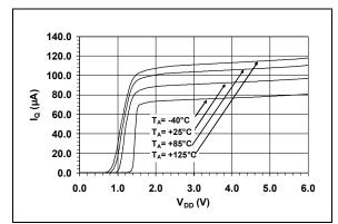
**FIGURE 2-17:** Quiescent Current vs. Supply Voltage vs. Temperature.
