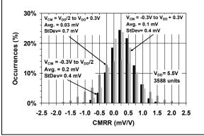
FIGURE 2-41: Common-Mode Rejection Ratio (CMRR).
