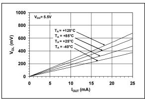
*FIGURE 2-24:* Output Headroom vs. Output Current.
