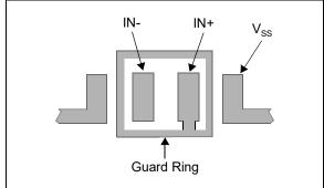
**FIGURE 4-9:** Example Guard Ring Layout for Inverting Circuit.
