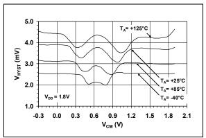
**FIGURE 2-11:** Input Hysteresis Voltage vs. Common-Mode Input Voltage.
