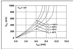
FIGURE 2-21: Output Headroom vs. Output Current.
