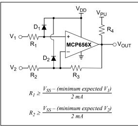
FIGURE 4-3: Protecting the Analog Inputs.
