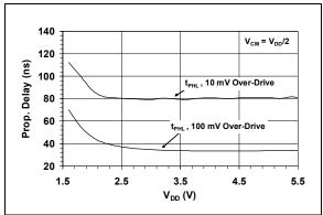
FIGURE 2-27: Propagation Delay vs. Supply Voltage.
