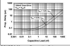
FIGURE 2-32: Propagation Delay vs. Capacitive Load.
