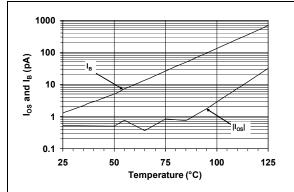
**FIGURE 2-39:** Input Offset Current and Input Bias Current vs. Temperature.
