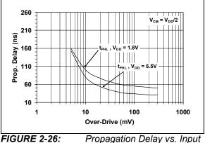
FIGURE 2-26: Propagation D Overdrive.
