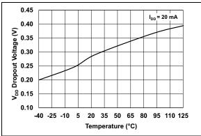
**FIGURE 7-6:** V<sub>DD</sub> Dropout Voltage vs. Temperature.
