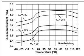
FIGURE 7-1: I<sub>O</sub> vs. Temperature.
