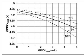
FIGURE 7-16: Average GPIO Output Voltage vs. Current.
