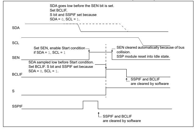
FIGURE 28-26: BUS COLLISION DURING A START CONDITION (SCL = 0)
