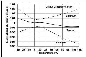
**FIGURE 7-13:** Normalized Output Demand vs. Temperature.
