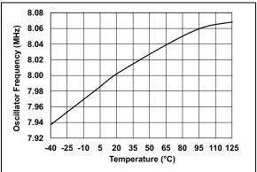
**FIGURE 7-12:** Oscillator Frequency vs. Temperature.
