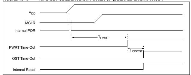
FIGURE 13-5: TIME-OUT SEQUENCE ON POWER-UP (DELAYED MCLR): CASE 2
