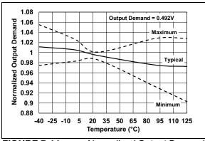
**FIGURE 7-14:** Normalized Output Demand vs. Temperature.
