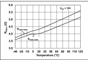
**FIGURE 7-9:** Sinking Output Driver R<sub>DSon</sub> vs. Temperature.
