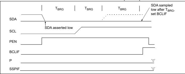
FIGURE 28-31: BUS COLLISION DURING A STOP CONDITION (CASE 2)
