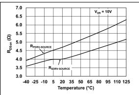
FIGURE 7-8: Sourcing Output Driver R<sub>DSon</sub> vs. Temperature.
