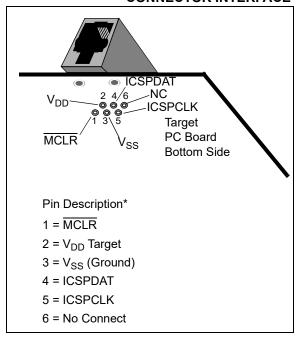
Another connector often found in use with the PICkit™ programmers is a standard 6-pin header with 0.1 inch spacing. Refer to Figure 30-2.
