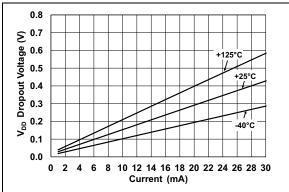
**FIGURE 7-5:** V<sub>DD</sub> Dropout Voltage vs. Output Current (mA).
