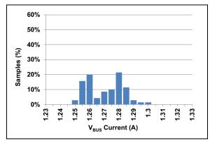
**FIGURE 2-16:** ILIM4 Trip Current Distribution<sup>(1)</sup>.
