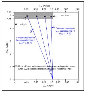
FIGURE 6-3: Current Limiting in CC Mode.
