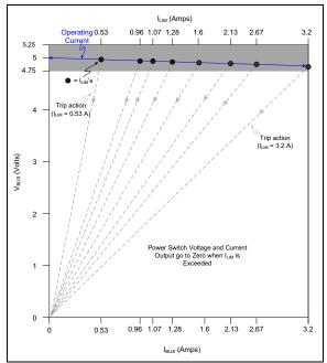
FIGURE 6-1: Current Limiting in Trip Mode.
