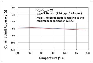
**FIGURE 2-9:** Trip Current Limit Operation vs. Temperature.
