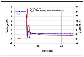
FIGURE 2-3: Internal Power Switch Short Response.
