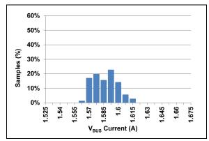
**FIGURE 2-17:** ILIM5 Trip Current Distribution<sup>(1)</sup>.
