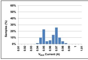
**FIGURE 2-14:** ILIM2 Trip Current Distribution<sup>(1)</sup>.
