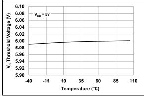
**FIGURE 2-7:**  $V_S$  Overvoltage Threshold vs. Temperature.
