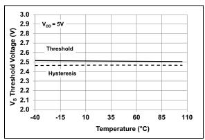
**FIGURE 2-8:**  $V_S$  Undervoltage Threshold vs. Temperature.
