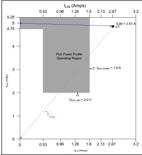
FIGURE 6-5:  $I_{LIM} > I_{BUS\_R2MIN}$  Example.
