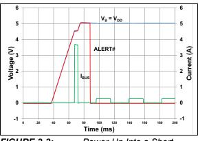
FIGURE 2-2: Power-Up Into a Short.
