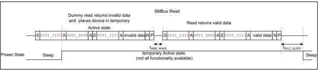
FIGURE 5-2: Wake from Sleep using SMBus Read.
