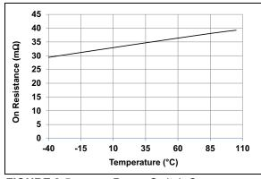
Power Switch On FIGURE 2-5: Resistance vs. Temperature.
