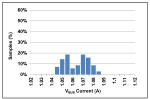
**FIGURE 2-15:** ILIM3 Trip Current Distribution<sup>(1)</sup>.
