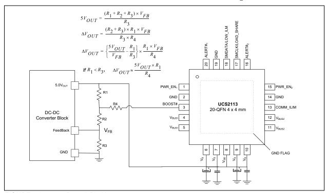
FIGURE 5-3: Boost# Pin Usage.
