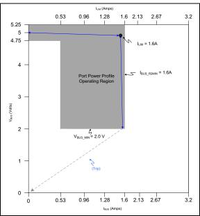
FIGURE 6-4: I<sub>LIM</sub> < I<sub>BUS R2MIN</sub> Example.
