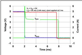
FIGURE 2-1: Short Applied After Power-Up.
