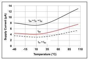
**FIGURE 2-12:** Sleep State Current vs. Temperature.
