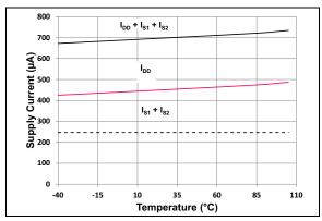
FIGURE 2-11: Active State Current vs. Temperature (both channels on, PWR\_EN1 = PWR\_EN2 = 1).
