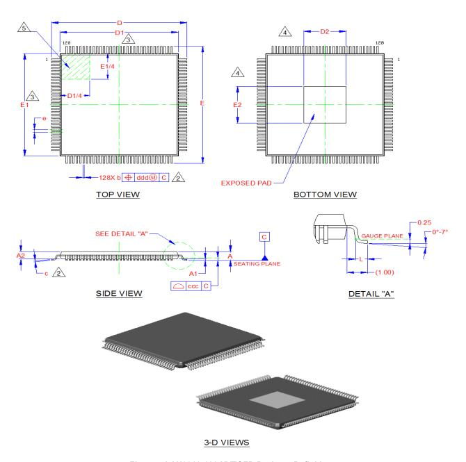
Figure 5 LAN9312 128-XVTQFP Package Definition
