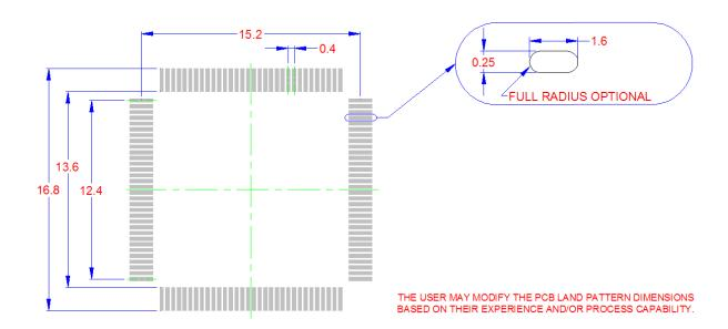
Figure 4 LAN9312 128-VTQFP Recommended PCB Land Pattern
