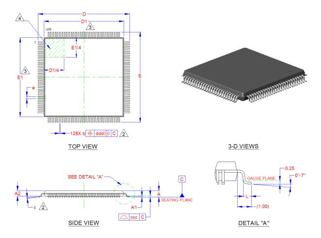
Figure 3 LAN9312 128-VTQFP Package Definition
