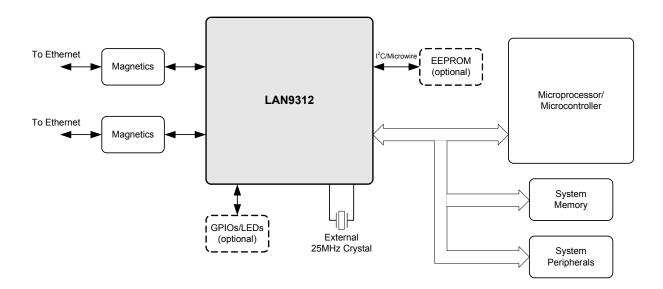
Figure 1 System Level Block Diagram Utilizing the LAN9312
