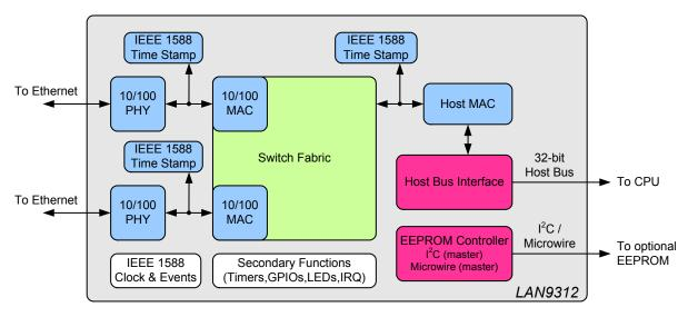
Figure 2 LAN9312 Internal Block Diagram
