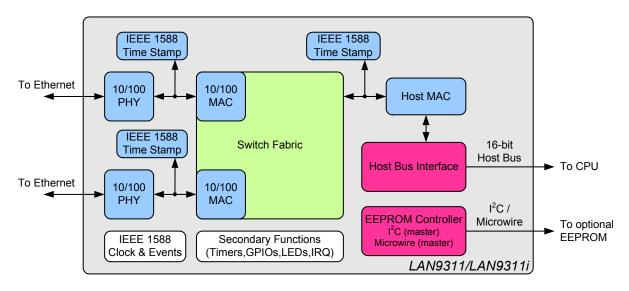
Figure 2 LAN9311/LAN9311i Internal Block Diagram
