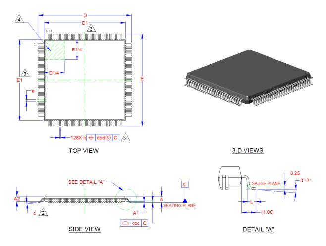
Figure 3 LAN9311 128-VTQFP Package Definition
