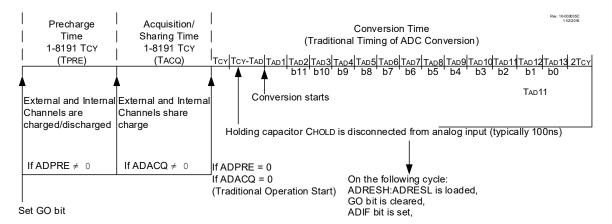
For correct conversion, the appropriate T<sub>AD</sub> specification must be met. Access the "ADC Timing Specifications" section for more information. The following table below gives examples of appropriate ADC clock selections.
