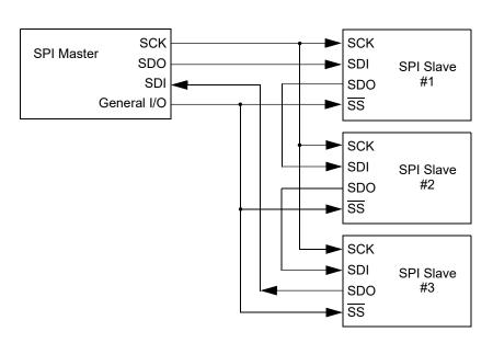
In a daisy-chain configuration, only the most recent byte on the bus is required by the slave. Setting the BOEN bit will enable writes to the SSPxBUF register, even if the previous byte has not been read. This allows the software to ignore data that may not apply to it.
