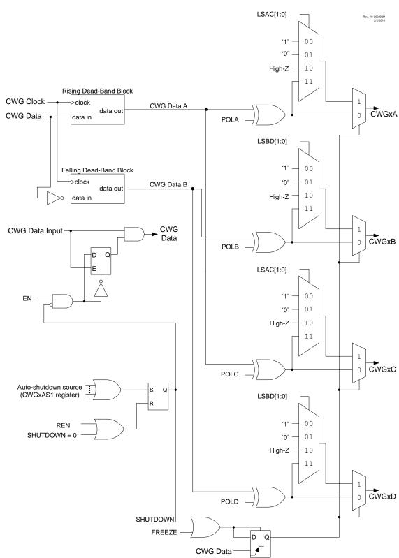
Figure 25-2. Simplified CWG Block Diagram (Half-Bridge Mode, MODE[2:0] = 100)
