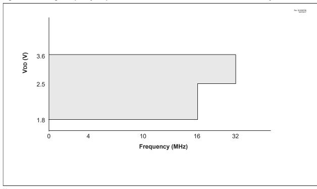
Figure 40-2. Voltage Frequency Graph, -40°C ≤ T<sub>A</sub>≤ +125°C, for PIC16LF18455/56 Devices only
