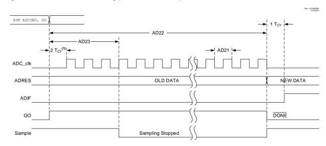
Figure 40-11. ADC Conversion Timing (ADC Clock from F<sub>RC</sub>)
