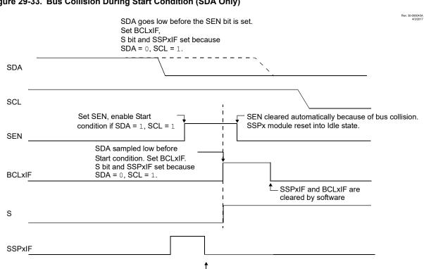
Figure 29-33. Bus Collision During Start Condition (SDA Only)
