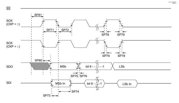
Figure 40-18. SPI Master Mode Timing (CKE = 1, SMP = 1)
