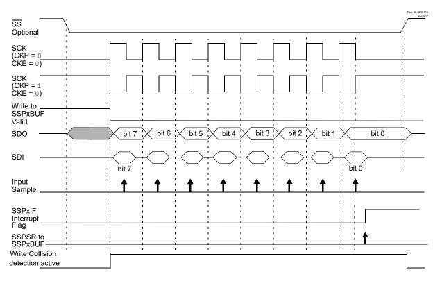
Figure 29-7. SPI Mode Waveform (Slave Mode with CKE = 0)
