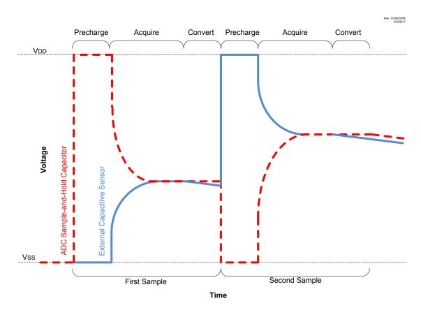
Figure 32-7. Differential CVD Measurement Waveform
