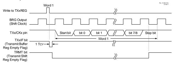
Figure 28-4. Asynchronous Transmission (Back-to-Back)
