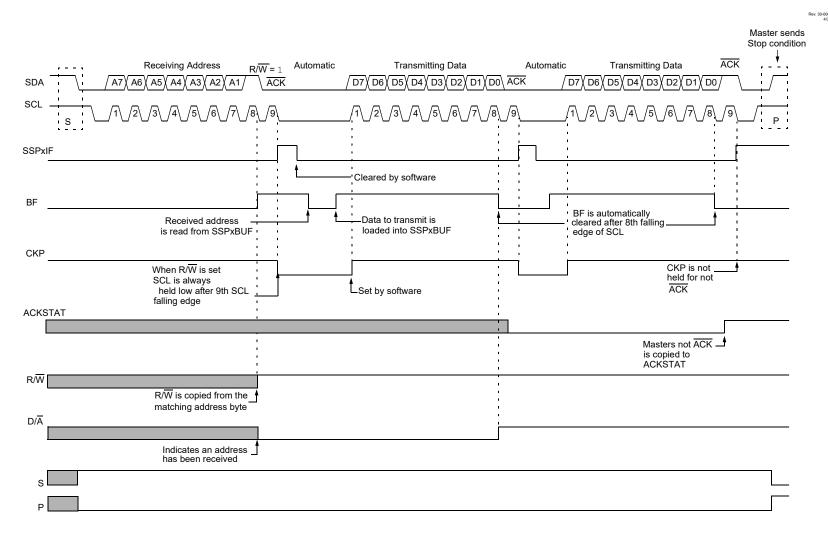
**MSSP - Master Synchronous Serial Port Module**
