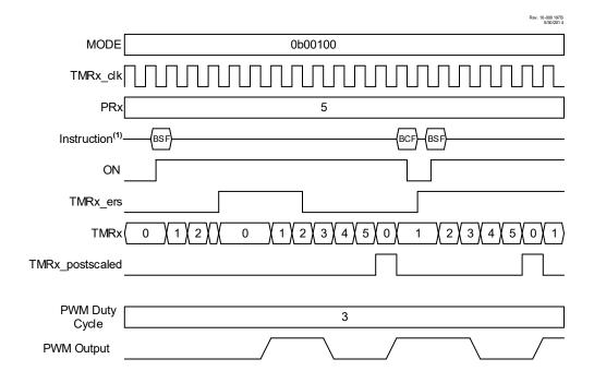
1. BSF and BCF represent Bit-Set File and Bit-Clear File instructions executed by the CPU to set or clear the ON bit of TxCON. CPU execution is asynchronous to the timer clock input.
