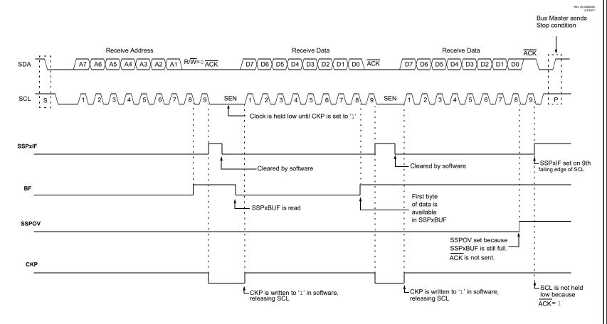
Figure 29-16. I<sup>2</sup>C Slave, 7-bit Address, Reception (SEN = 0, AHEN = 1, DHEN = 1)
