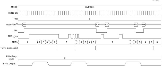
1. BSF and BCF represent Bit-Set File and Bit-Clear File instructions executed by the CPU to set or clear the ON bit of TxCON. CPU execution is asynchronous to the timer clock input.
