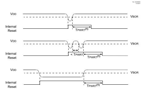
**Note:** T<sub>PWRT</sub> delay only if PWRTS bit field is programmed to a value different from '11'.
