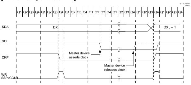
Figure 29-23. Clock Synchronization Timing
