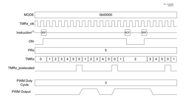
BSF and BCF represent Bit-Set File and Bit-Clear File instructions executed by the CPU to set or clear the ON bit of TxCON. CPU execution is asynchronous to the timer clock input.
