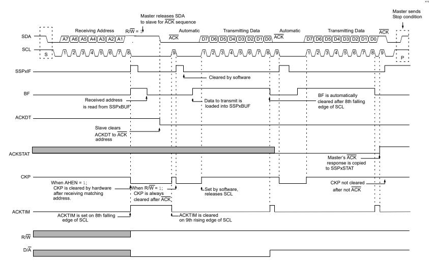
**MSSP - Master Synchronous Serial Port Module**
