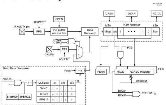
Figure 28-2. EUSART Receive Block Diagram
