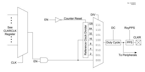
Figure 9-2. Clock Reference Timing
