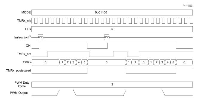
1. BSF and BCF represent Bit-Set File and Bit-Clear File instructions executed by the CPU to set or clear the ON bit of TxCON. CPU execution is asynchronous to the timer clock input.
