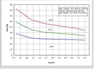
Figure 41-85. Comparator Response Time Falling Edge, PIC16LF18455/56 only
