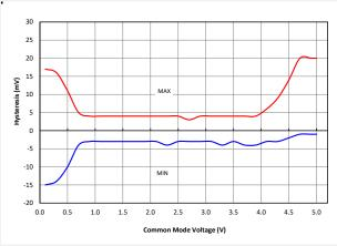
Figure 41-82. Comparator Offset, Normal Power Mode (CxSP = 1),  $V_{DD}$  = 5.5V, Typical Measured Values from -40°C to 125°C, PIC16F18455/56 only
