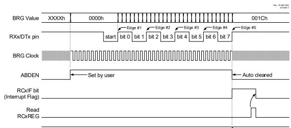
Figure 28-6. Automatic Baud Rate Calibration
