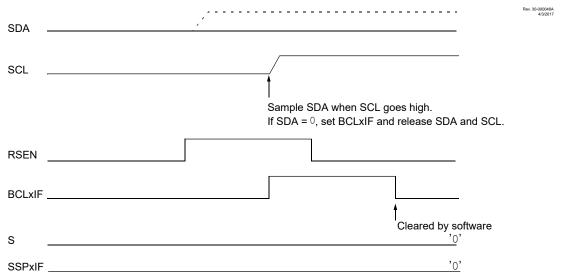
If SCL goes from high-to-low before the BRG times out and SDA has not already been asserted, a bus collision occurs. In this case, another master is attempting to transmit a data '1' during the Repeated Start condition, see Figure 29-37.
