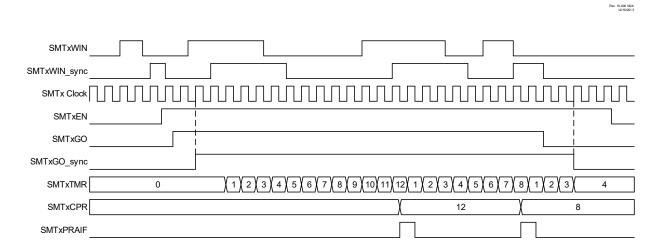
Figure 21-10. Windowed Measurement Mode, Single Acquisition Timing Diagram
