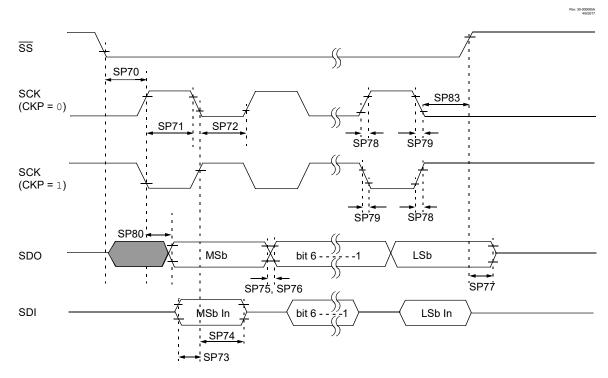
Figure 40-20. SPI Slave Mode Timing (CKE = 1)
