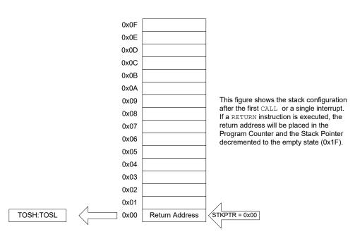
Figure 5-6. Accessing the Stack Example 3
