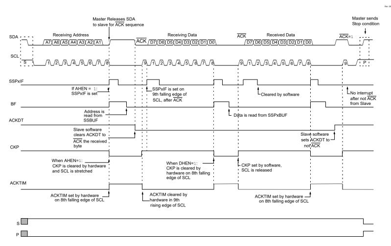
**MSSP - Master Synchronous Serial Port Module**
