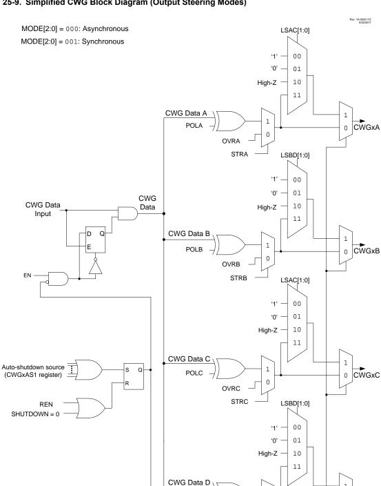
Figure 25-9. Simplified CWG Block Diagram (Output Steering Modes)
