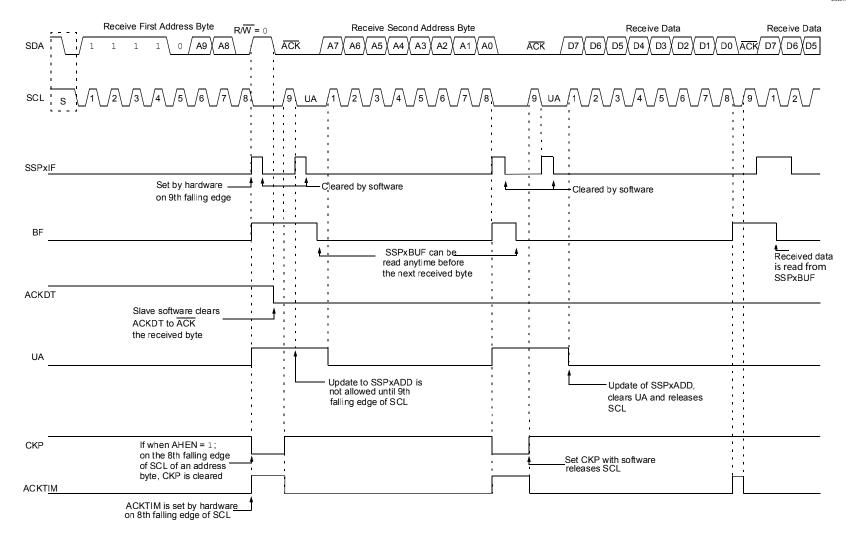
Figure 29-22. I<sup>2</sup>C Slave, 10-bit Address, Transmission (SEN = 0, AHEN = 0, DHEN = 0)
