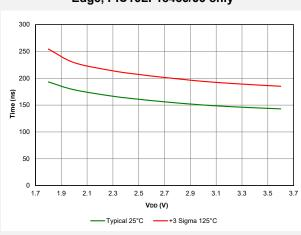
Figure 41-86. Comparator Response Time Falling Edge, PIC16F18455/56 only
