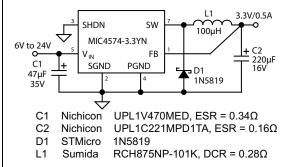
FIGURE 4-1: 6V<sub>IN</sub> - 24V<sub>IN</sub> to 3.3V/0.5A Buck Converter Through Hole.
