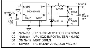
**FIGURE 4-3:**  $16V_{IN}$  -  $24V_{IN}$  to 12V/0.5A Buck Converter Through Hole.
