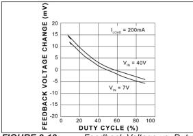
**FIGURE 2-13:** Feedback Voltage vs. Duty Cycle (Adjustable Version Only).
