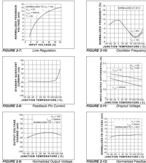
**FIGURE 2-12:** Normalized Feedback Voltage (Adjustable Version Only).
