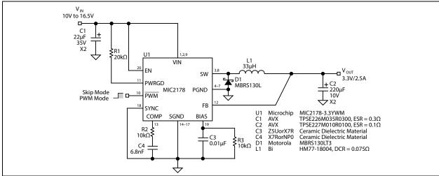
FIGURE 5-4: MIC2178 10V - 16.5V to 3.3V/2.5A Regulator.
