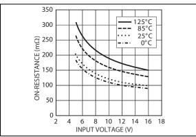
FIGURE 2-9: Low-Side Switch On-Resistance.
