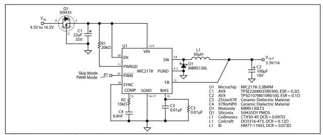
FIGURE 5-6: MIC2178 Reversed Battery Protected Regulator.
