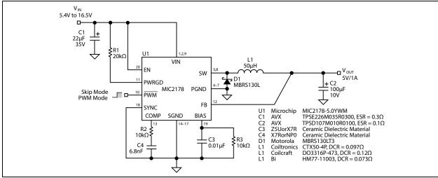
FIGURE 5-2: MIC2178 5.4V - 16.5V to 5V/1A Regulator.
