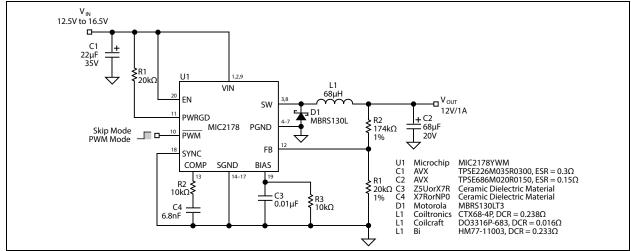
FIGURE 5-3: MIC2178 12.5V - 16.5V to 12V/1A Regulator.
