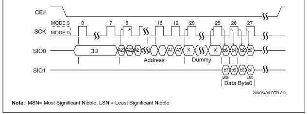
FIGURE 5-17: SPI DUAL OUTPUT READ – DTR
