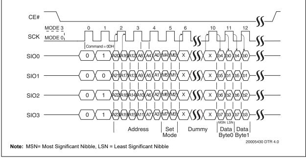
FIGURE 5-19: SQI HIGH-SPEED READ – DTR
