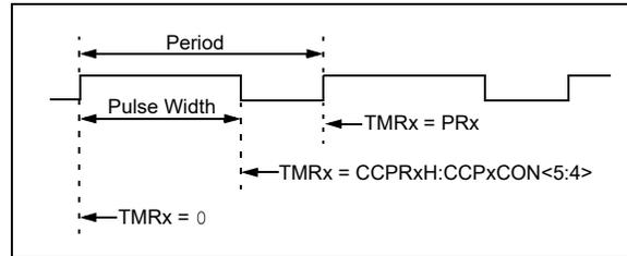
FIGURE 23-4: SIMPLIFIED PWM BLOCK DIAGRAM
