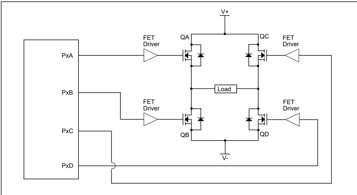
**FIGURE 23-11: EXAMPLE OF FULL-BRIDGE PWM OUTPUT**
