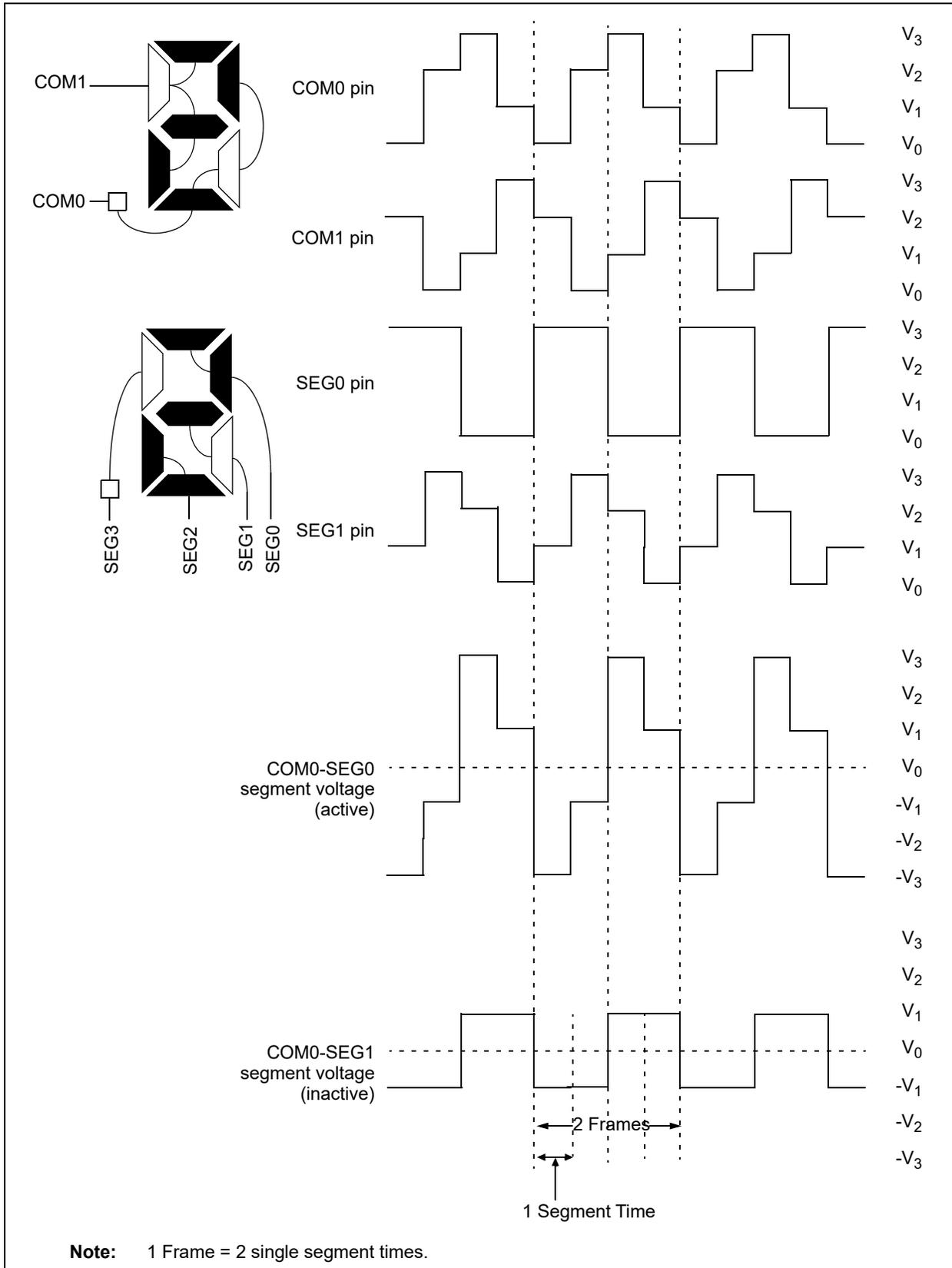
**FIGURE 27-13: TYPE-A WAVEFORMS IN 1/3 MUX, 1/2 BIAS DRIVE**
