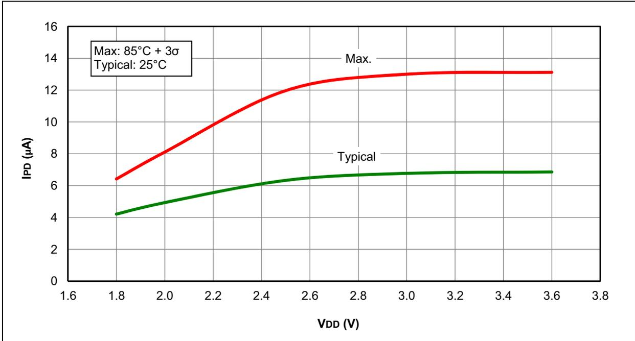
**FIGURE 31-44: I<sub>PD</sub>, CAPACITIVE SENSING (CPS) MODULE, MEDIUM-CURRENT RANGE (CPSRM = 0, CPSRNG = 10), PIC16F1938/9 ONLY**
