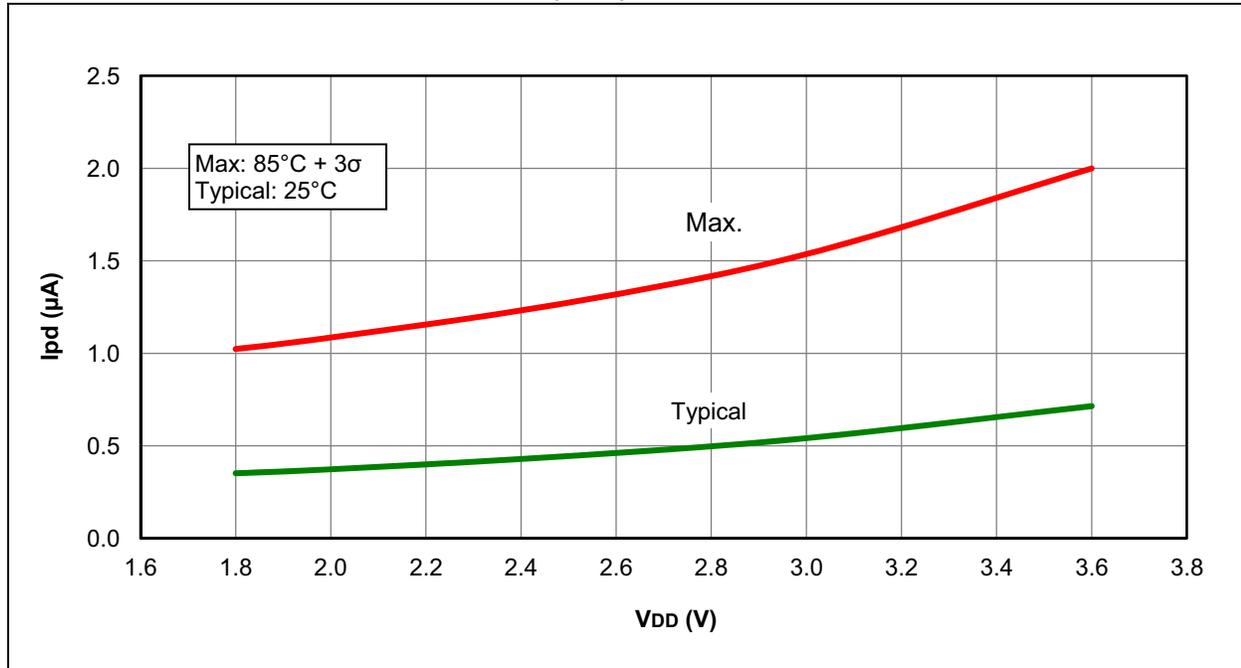
FIGURE 31-34: I<sub>PD</sub>, WATCHDOG TIMER (WDT), PIC16F1938/9 ONLY
