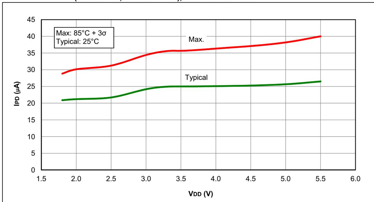
**FIGURE 31-43: I<sub>PD</sub>, CAPACITIVE SENSING (CPS) MODULE, MEDIUM-CURRENT RANGE (CPSRM = 0, CPSRNG = 10), PIC16LF1938/9 ONLY**
