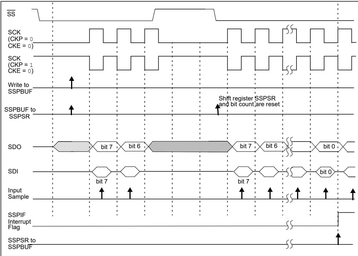
**FIGURE 24-9: SPI MODE WAVEFORM (CLIENT MODE WITH CKE = 0)**
