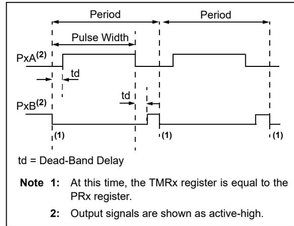
**FIGURE 23-9: EXAMPLE OF HALF-BRIDGE APPLICATIONS**
