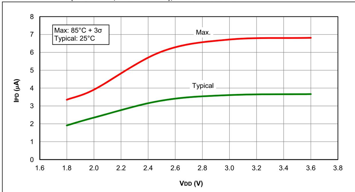
**FIGURE 31-42: I<sub>PD</sub>, CAPACITIVE SENSING (CPS) MODULE, LOW-CURRENT RANGE (CPSRM = 0, CPSRNG = 01), PIC16LF1938/9 ONLY**
