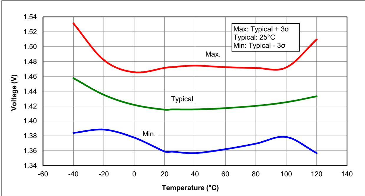
**FIGURE 31-59: BROWN-OUT RESET VOLTAGE, BORV = 1**
