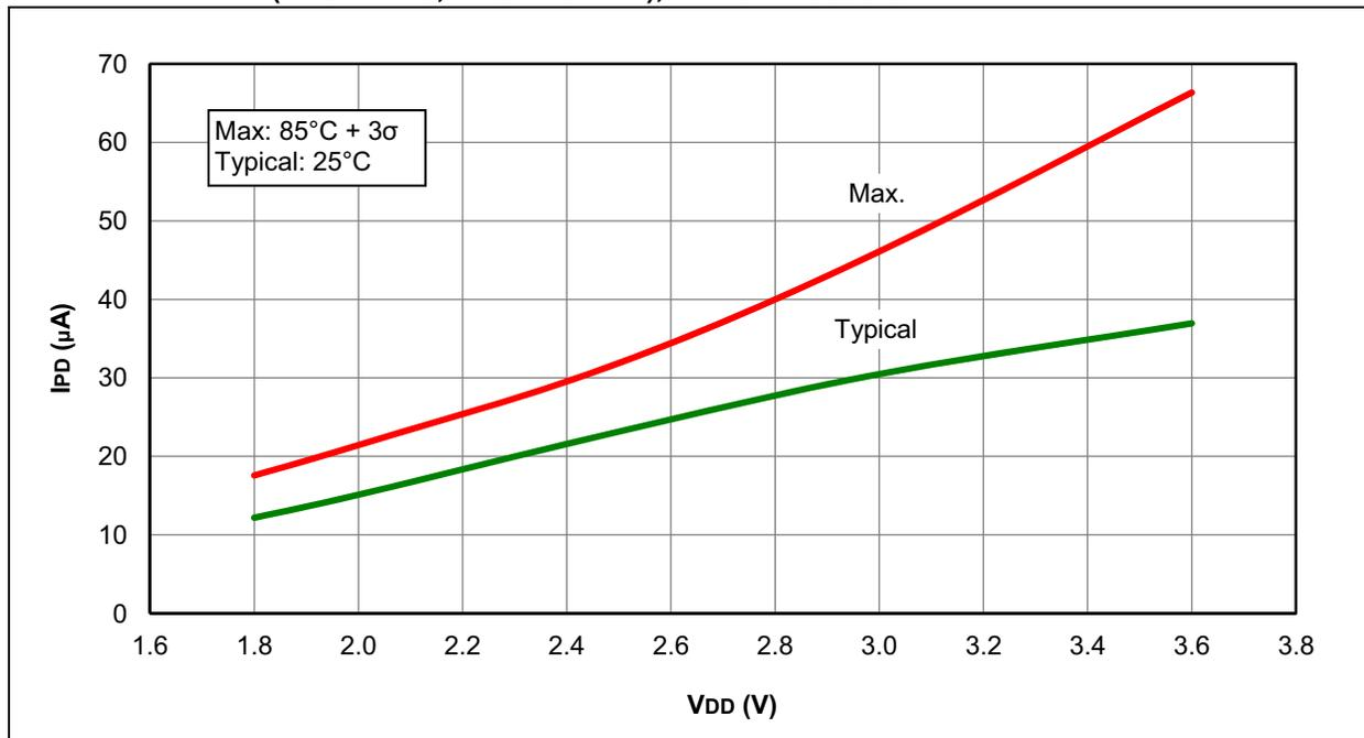
**FIGURE 31-46: I<sub>PD</sub>, CAPACITIVE SENSING (CPS) MODULE, HIGH-CURRENT RANGE (CPSRM = 0, CPSRNG = 11), PIC16F1938/9 ONLY**
