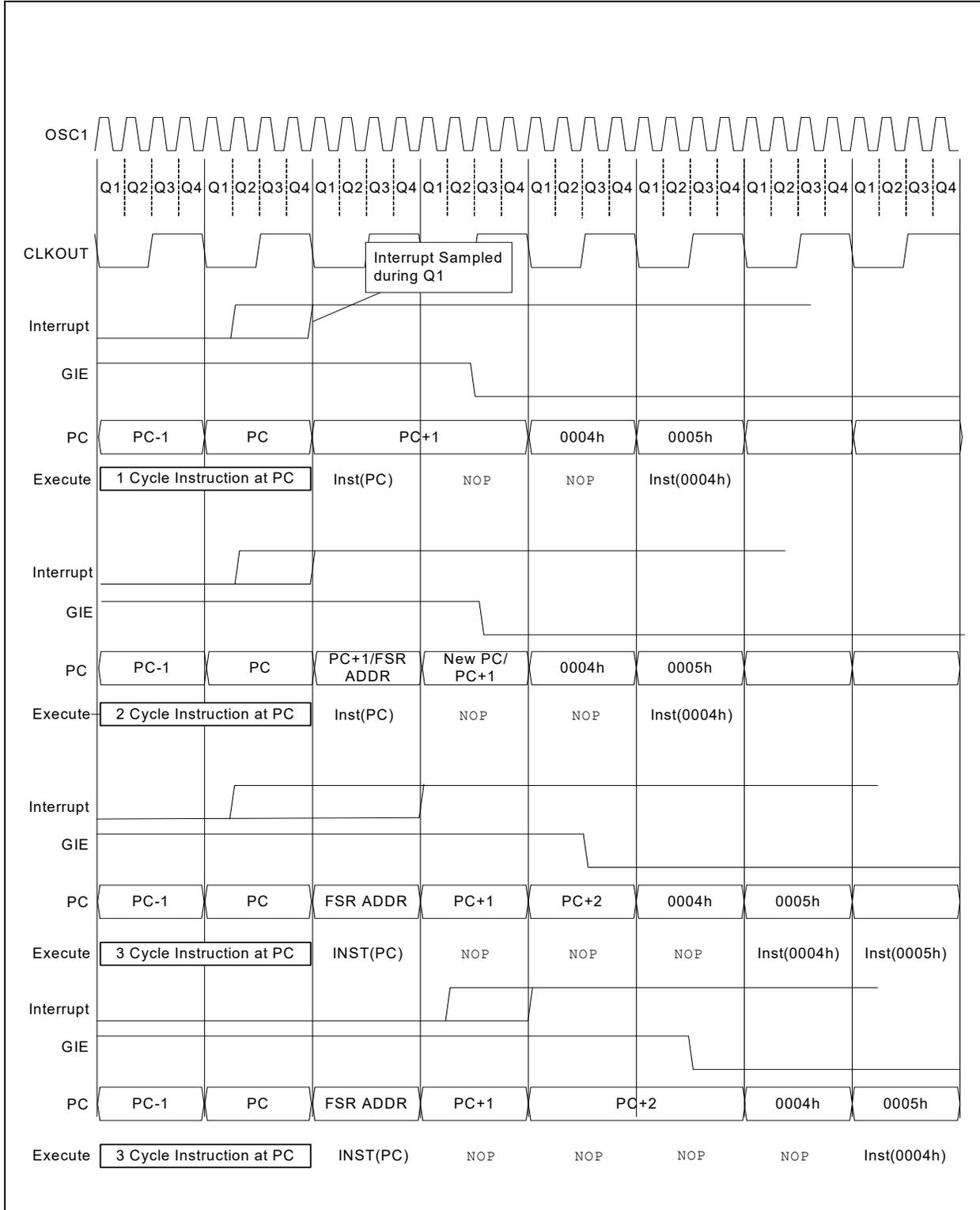
**FIGURE 7-3: INT PIN INTERRUPT TIMING**
