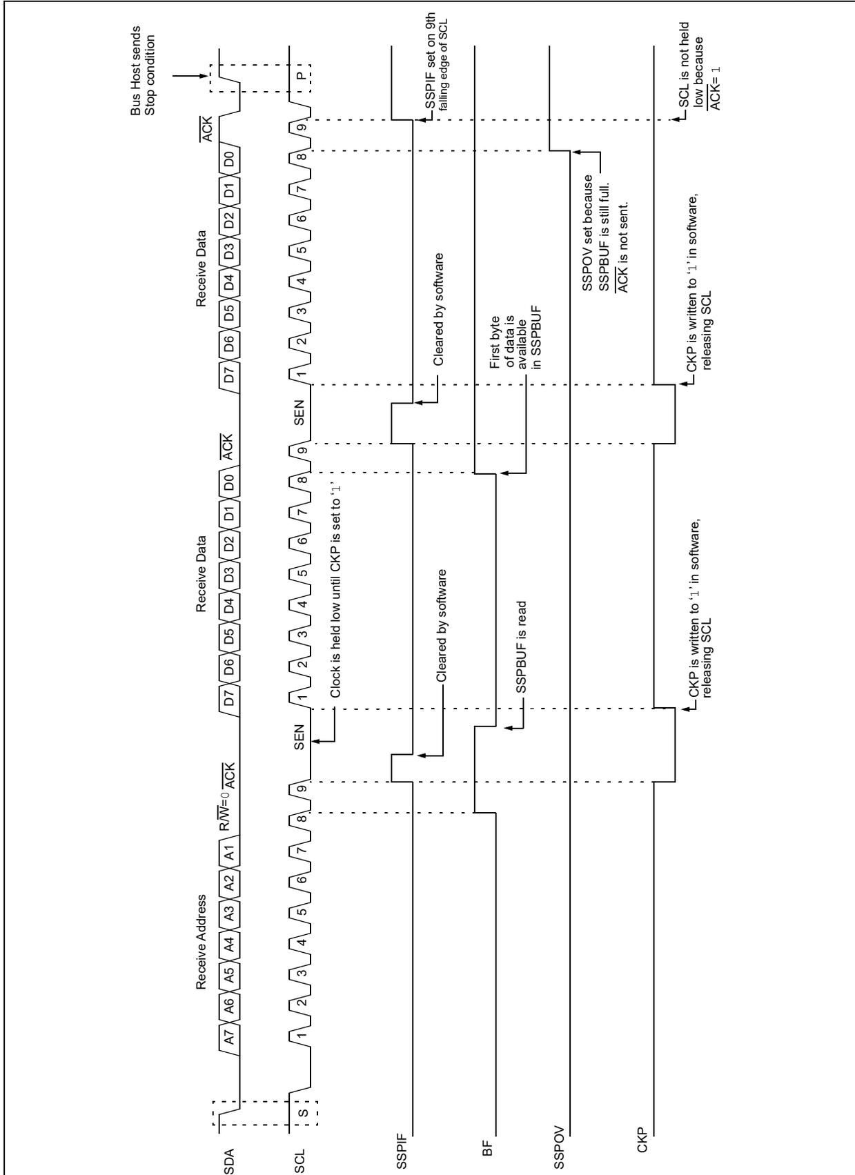
**FIGURE 24-16: I<sup>2</sup>C CLIENT, 7-BIT ADDRESS, RECEPTION (SEN = 0, AHEN = 1, DHEN = 1)**
