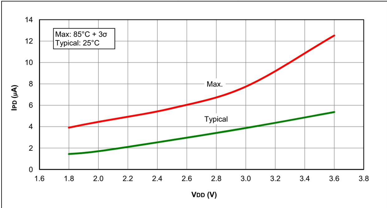
**FIGURE 31-40: I<sub>PD</sub>, TIMER1 OSCILLATOR, F<sub>osc</sub> = 32 kHz, PIC16F1938/9 ONLY**
