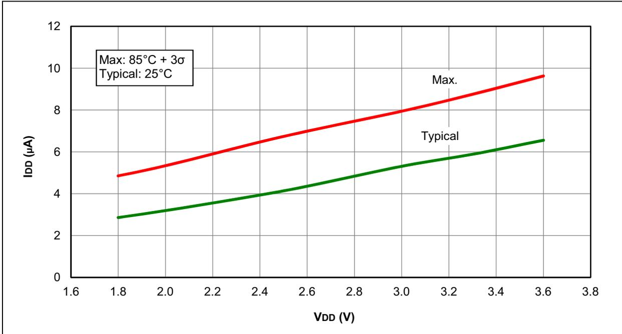
**FIGURE 31-8: I<sub>DD</sub>, EXTERNAL CLOCK (ECL), LOW-POWER MODE, F<sub>osc</sub> = 32 kHz, PIC16F1938/9 ONLY**
