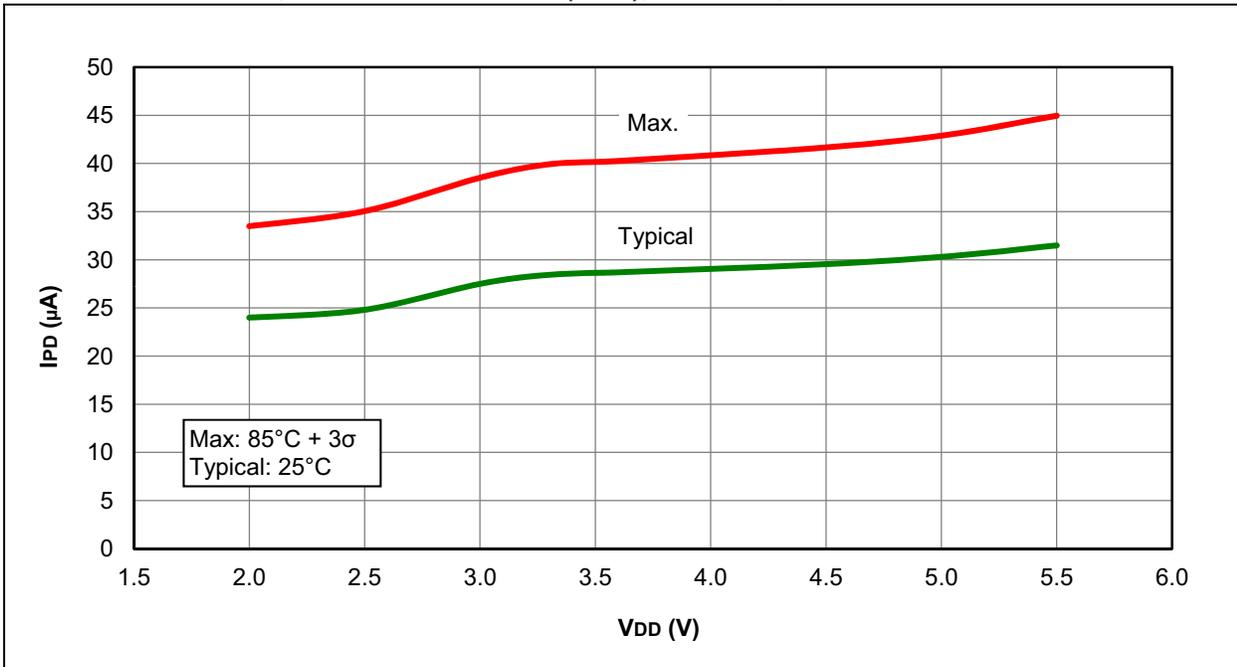
**FIGURE 31-39: I<sub>PD</sub>, TIMER1 OSCILLATOR, F<sub>osc</sub> = 32 kHz, PIC16LF1938/9 ONLY**
