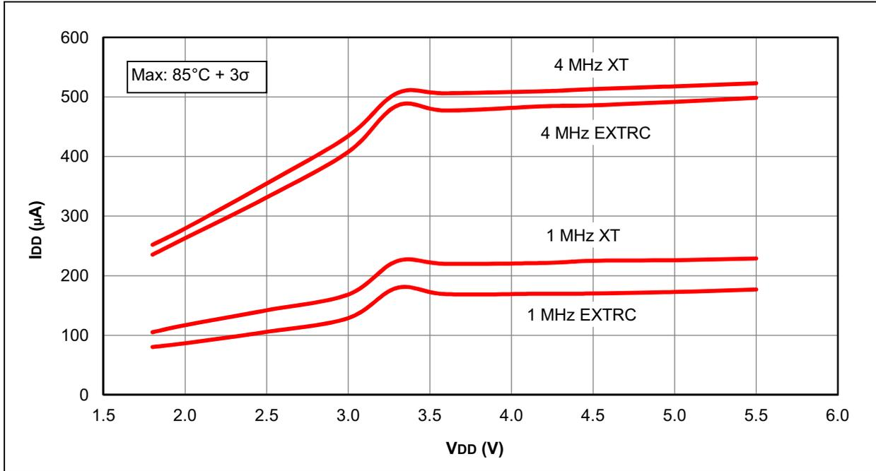
**FIGURE 31-7: I<sub>DD</sub>, EXTERNAL CLOCK (ECL), LOW-POWER MODE, F<sub>osc</sub> = 32 kHz, PIC16LF1938/9 ONLY**
