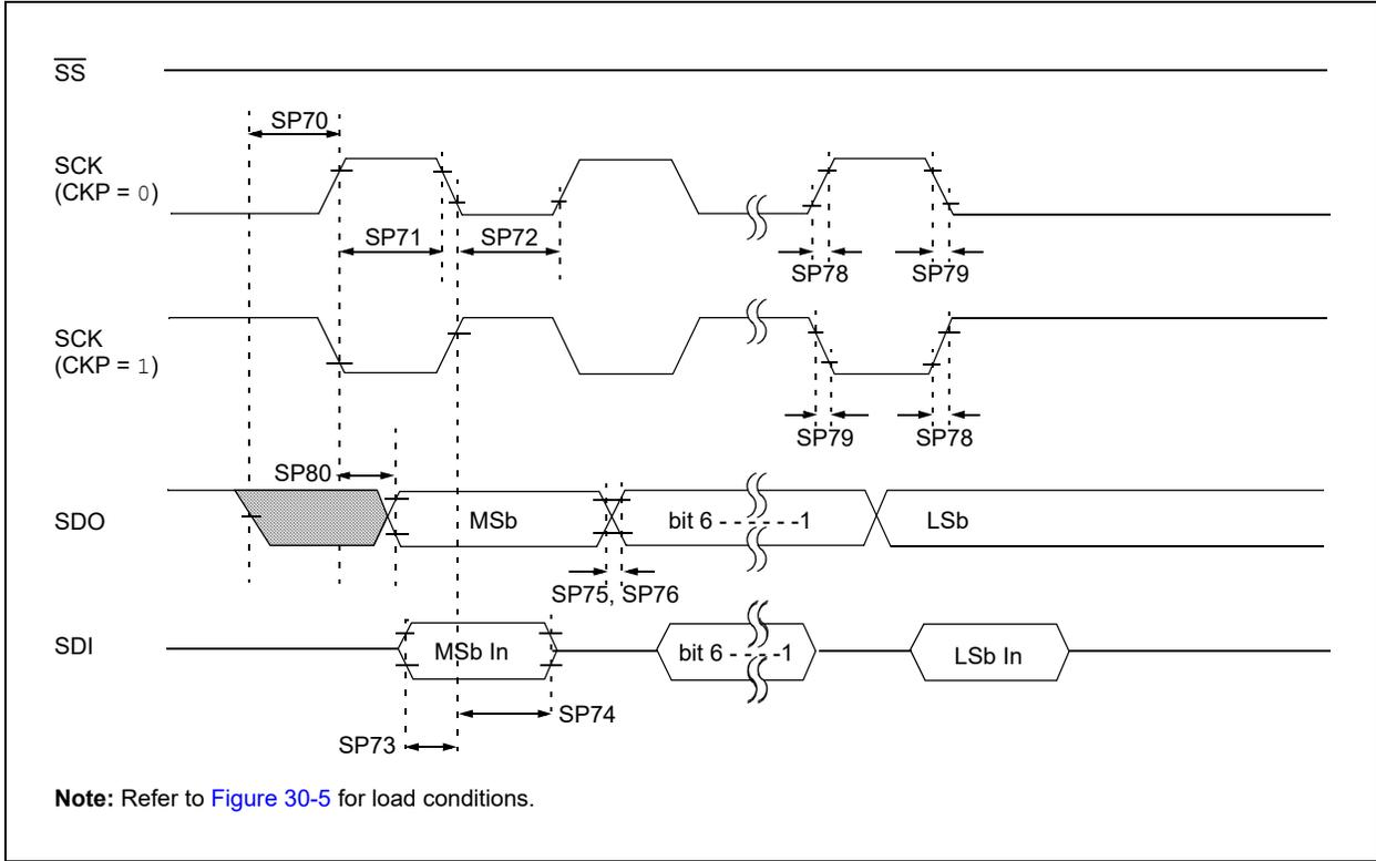
**FIGURE 30-17: SPI HOST MODE TIMING (CKE = 1, SMP = 1)**
