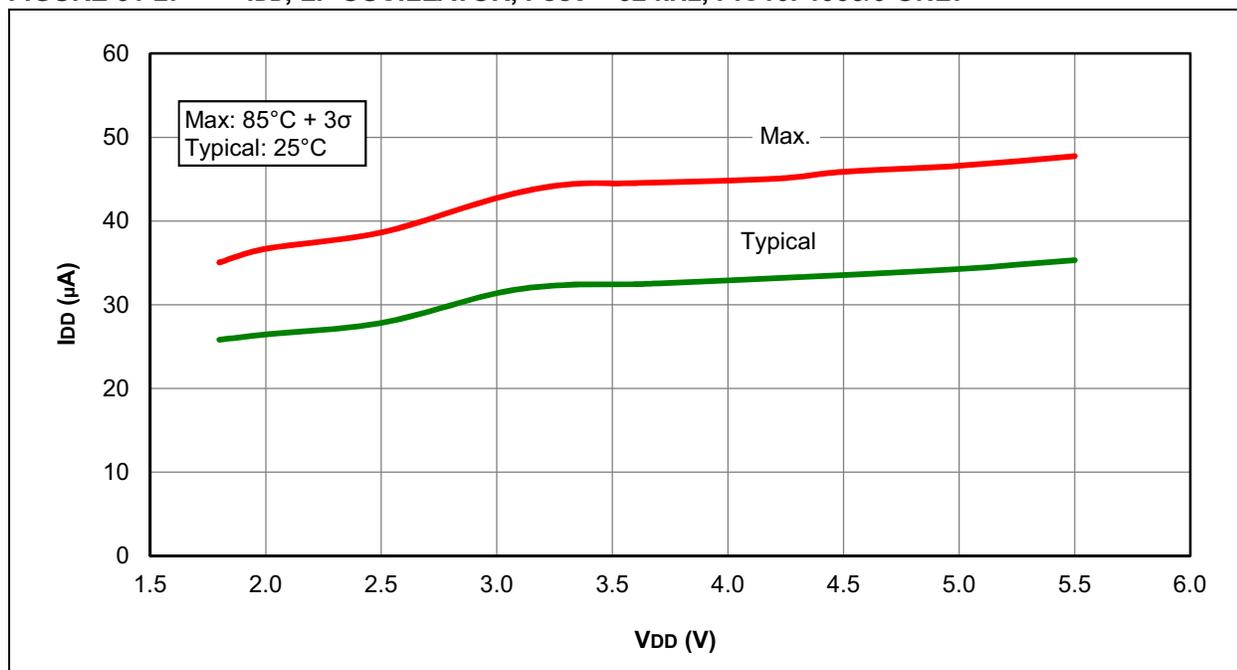
**FIGURE 31-3: I<sub>DD</sub> TYPICAL, XT AND EXTRC OSCILLATOR, PIC16LF1938/9 ONLY**
