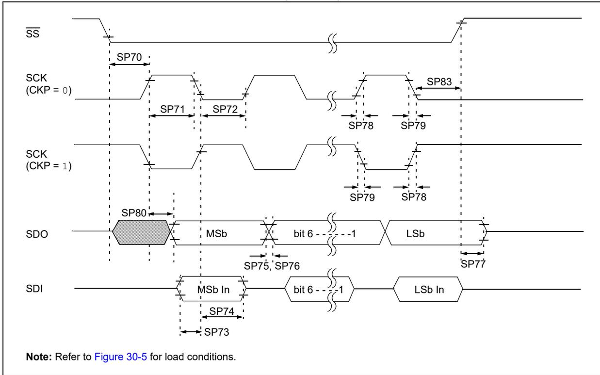
**FIGURE 30-19: SPI CLIENT MODE TIMING (CKE = 1)**
