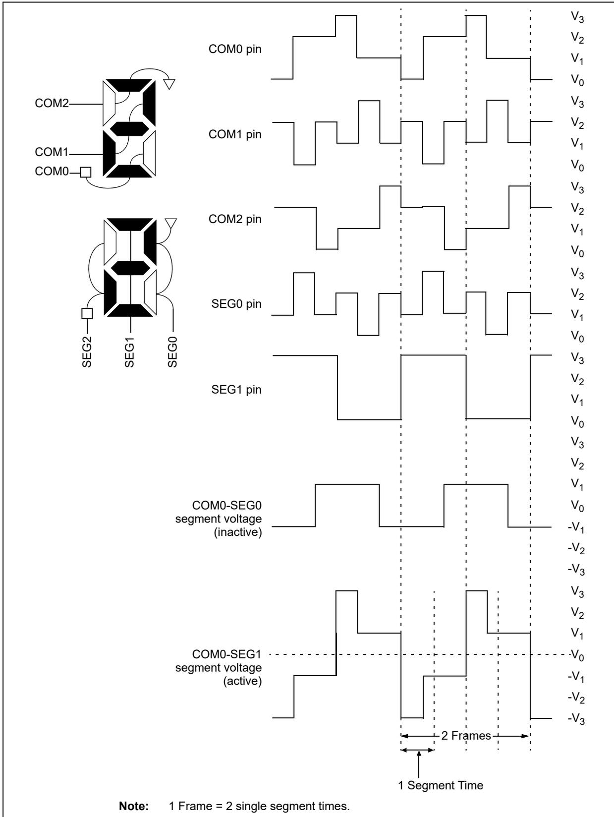
**FIGURE 27-17: TYPE-A WAVEFORMS IN 1/4 MUX, 1/3 BIAS DRIVE**
