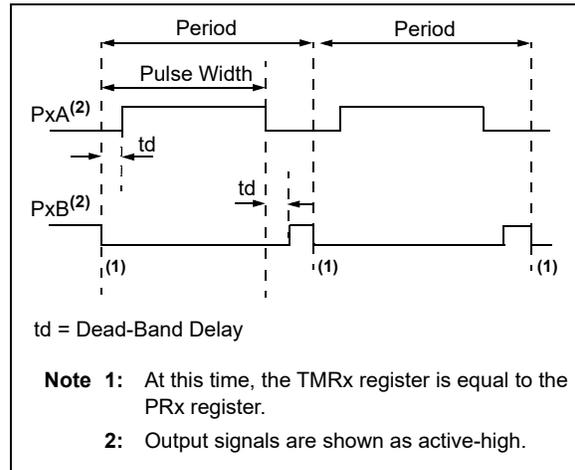
**FIGURE 23-17: EXAMPLE OF HALF-BRIDGE APPLICATIONS**
