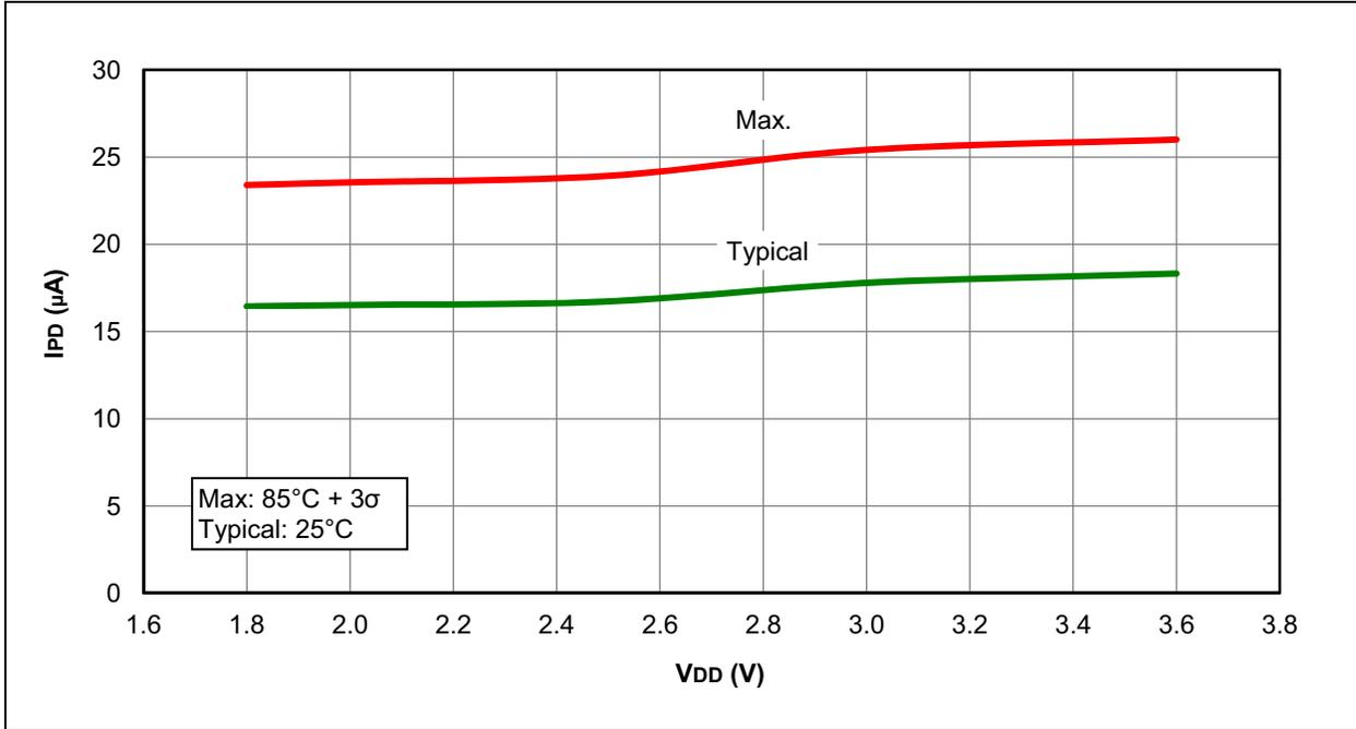
**FIGURE 31-48: I<sub>PD</sub>, COMPARATOR, LOW-POWER MODE, (C<sub>xSP</sub> = 0), PIC16F1938/9 ONLY**
