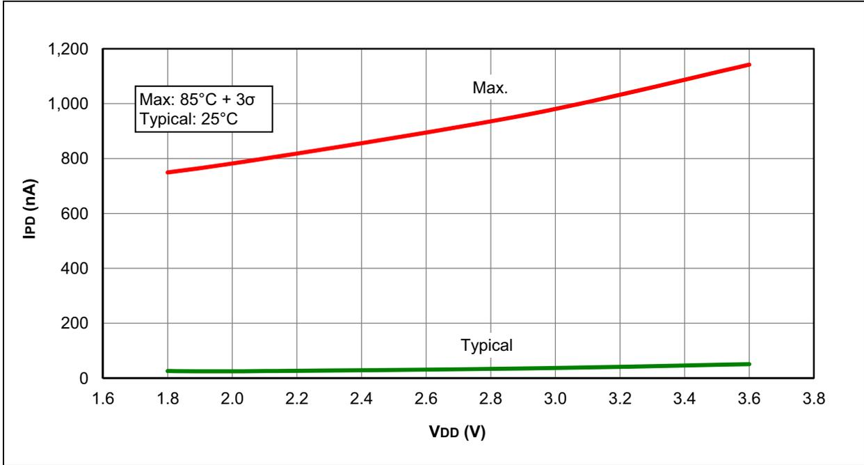
**FIGURE 31-32: I<sub>PD</sub> BASE, LOW-POWER SLEEP MODE, PIC16F1938/9 ONLY**
