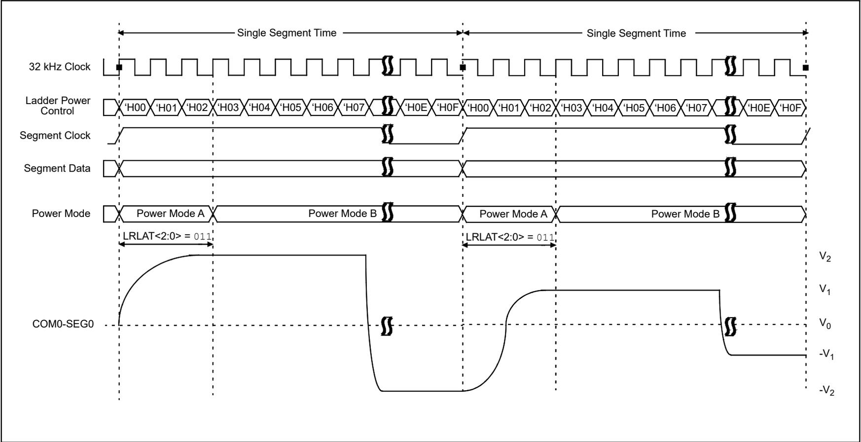
**FIGURE 27-6: LCD INTERNAL REFERENCE LADDER POWER MODE SWITCHING DIAGRAM – TYPE B WAVEFORM (1/2 MUX, 1/2 BIAS DRIVE)**
