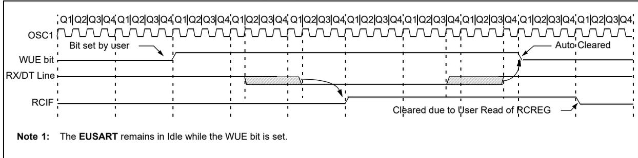
**FIGURE 25-8: AUTO-WAKE-UP BIT (WUE) TIMINGS DURING SLEEP**
