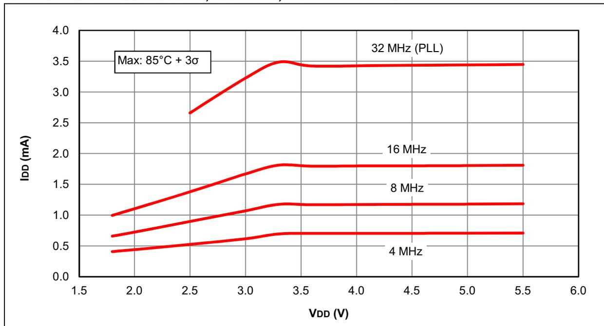
**FIGURE 31-27: I<sub>DD</sub> TYPICAL, HS OSCILLATOR, PIC16LF1938/9 ONLY**
