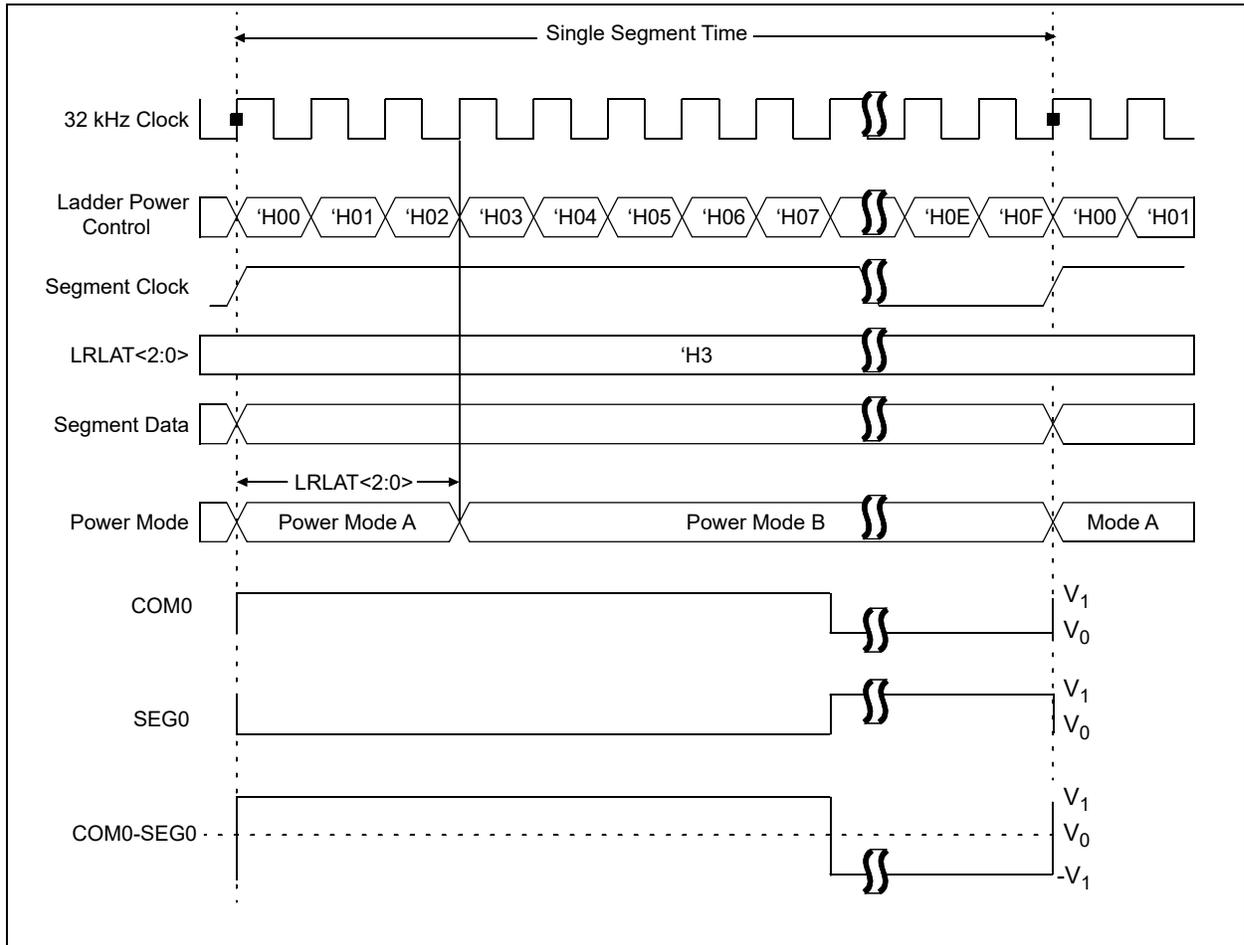
FIGURE 27-5: LCD INTERNAL REFERENCE LADDER POWER MODE SWITCHING DIAGRAM – TYPE A WAVEFORM (1/2 MUX, 1/2 BIAS DRIVE)
