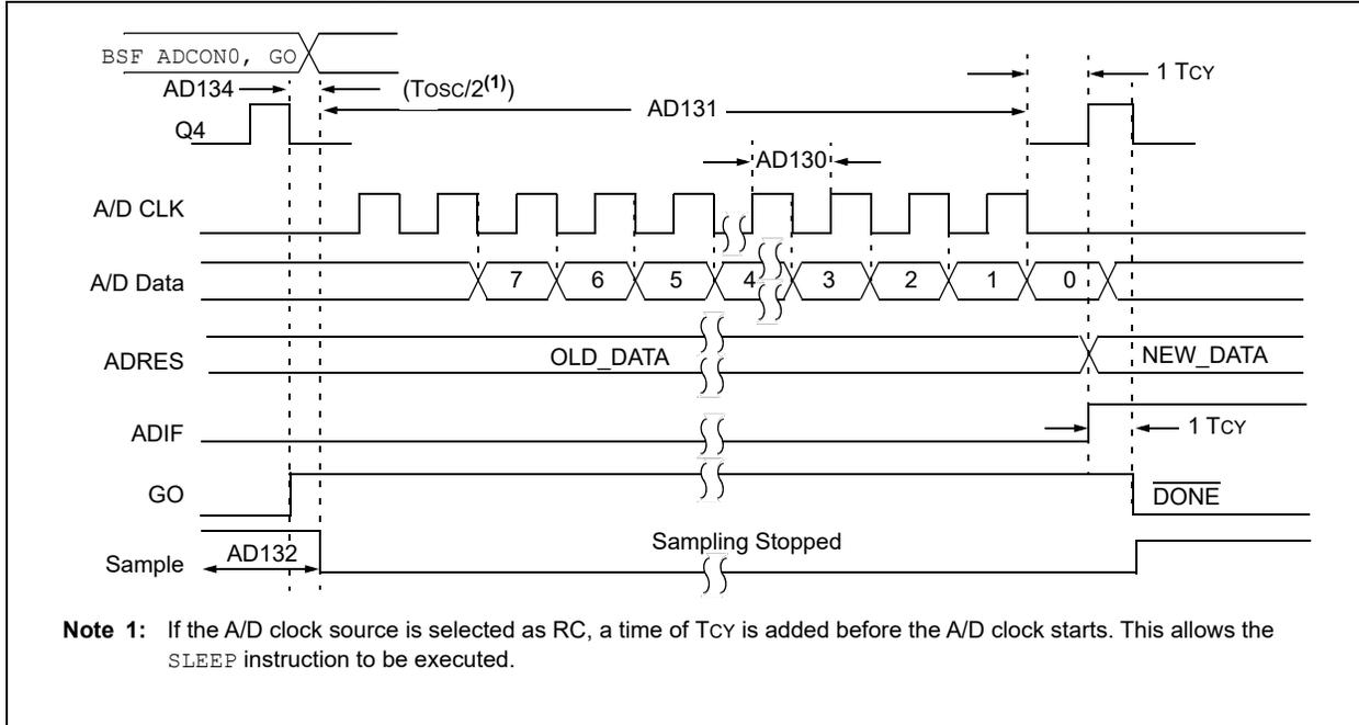
**FIGURE 30-13: PIC16(L)F1938/39 A/D CONVERSION TIMING (SLEEP MODE)**
