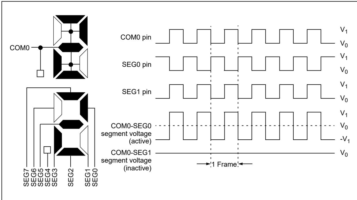
**FIGURE 27-9: TYPE-A WAVEFORMS IN 1/2 MUX, 1/2 BIAS DRIVE**
