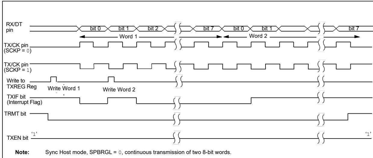
**FIGURE 25-11: SYNCHRONOUS TRANSMISSION (THROUGH TXEN)**
