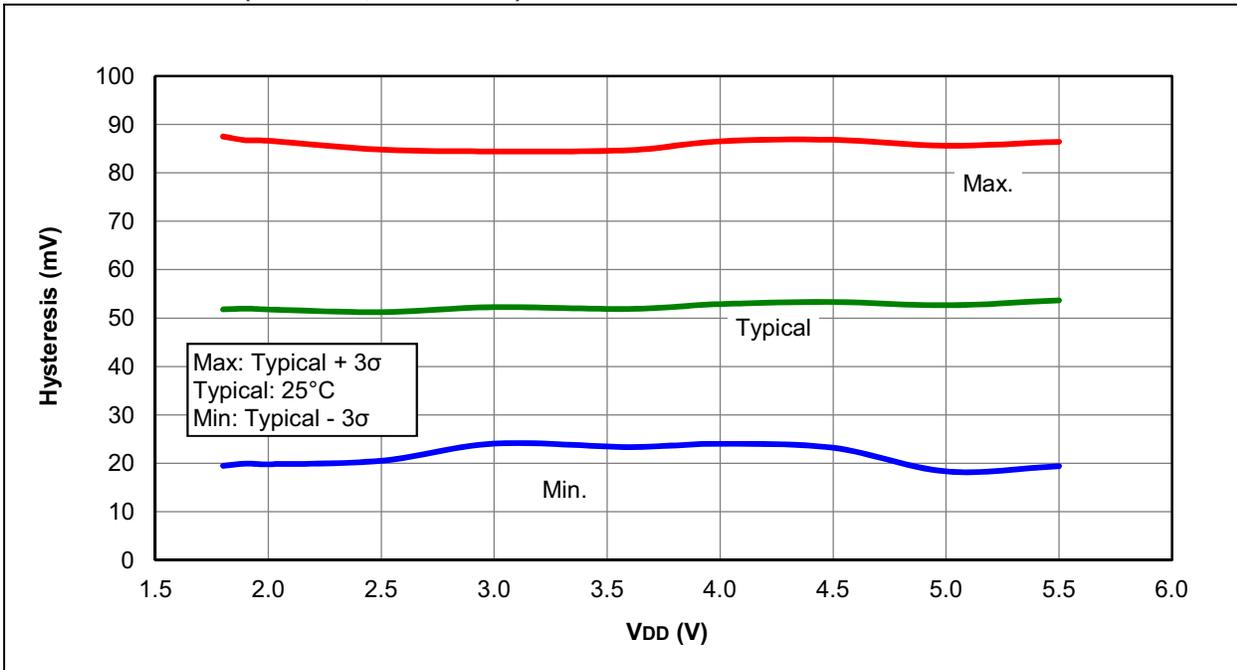
**FIGURE 31-66: COMPARATOR HYSTERESIS, LOW-POWER MODE**
