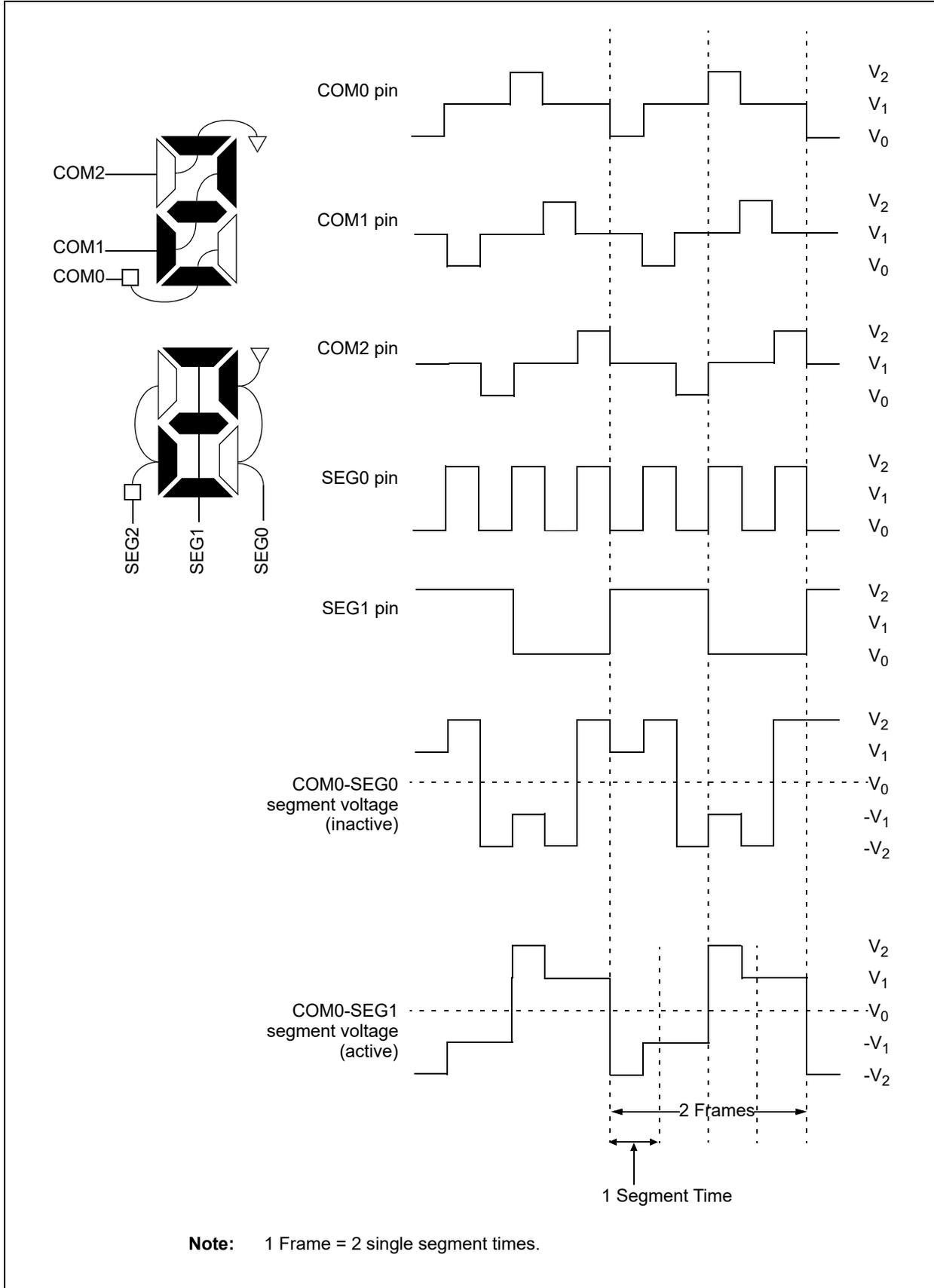
**FIGURE 27-15: TYPE-A WAVEFORMS IN 1/3 MUX, 1/3 BIAS DRIVE**
