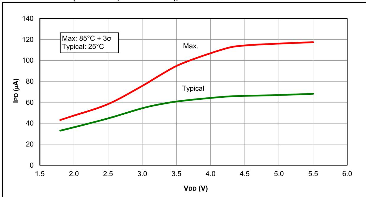
**FIGURE 31-47: I<sub>PD</sub>, COMPARATOR, LOW-POWER MODE, (C<sub>xSP</sub> = 0), PIC16LF1938/9 ONLY**
