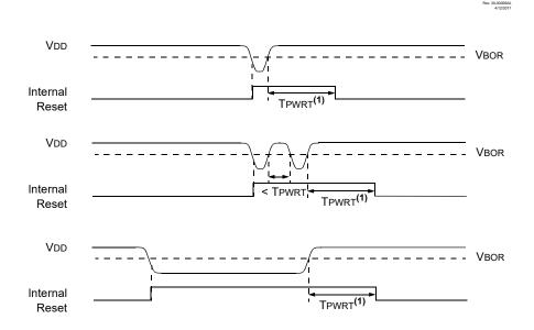
**Note:**  $T_{PWRT}$  delay only if  $\overline{PWRTE}$  bit is programmed to '0'.
