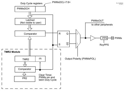
Note 1: 8-bit timer is concatenated with the two Least Significant bits of 1/Fosc adjusted by the Timer2 prescaler to create a 10-bit time base.
