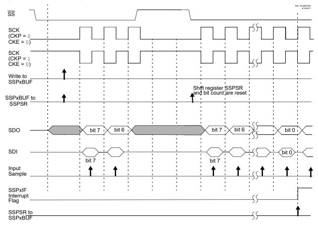
Figure 27-6. Slave Select Synchronous Waveform
