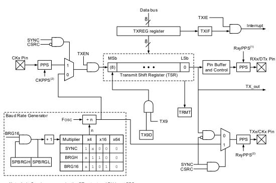
Note 1: In Synchronous mode, the DT output and RX input PPS selections should enable the same pin.
