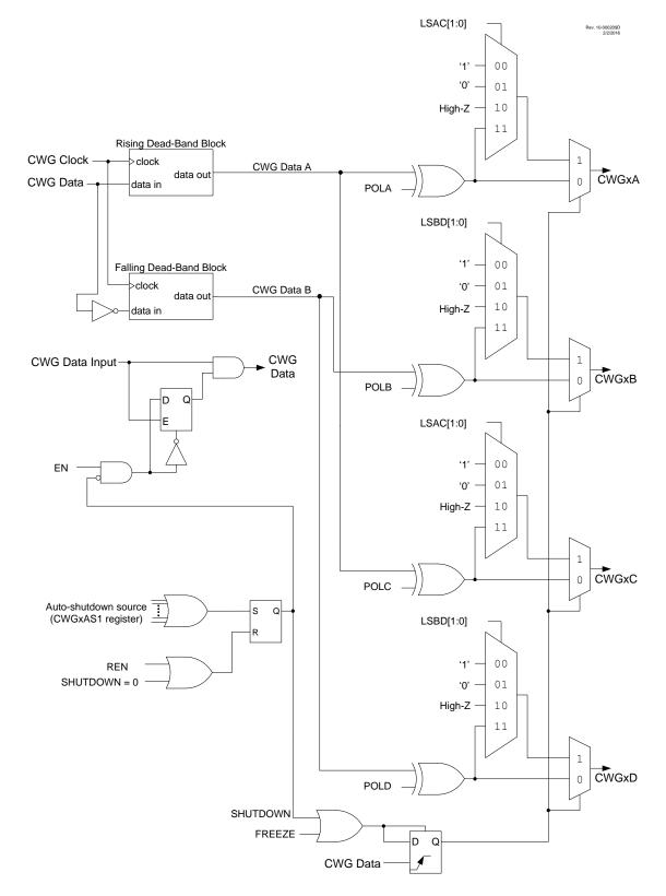
Figure 24-2. Simplified CWG Block Diagram (Half-Bridge Mode, MODE[2:0] = 100)
