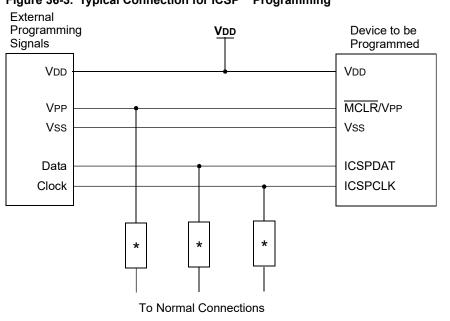
Figure 36-3. Typical Connection for ICSP<sup>™</sup> Programming
