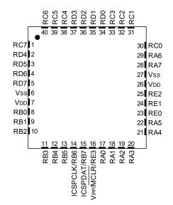
**Note:** It is recommended that the exposed bottom pad be connected to  $V_{SS}$ , however it must not be the only  $V_{SS}$  connection to the device.
