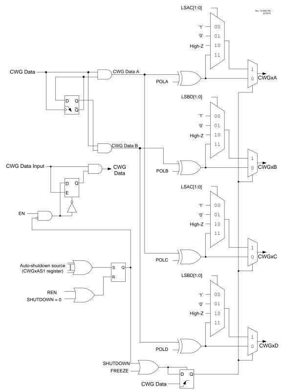
Figure 24-4. Simplified CWG Block Diagram (Push-Pull Mode, MODE[2:0] = 101)
