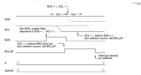
If the SDA pin is sampled low during this count, the BRG is reset and the SDA line is asserted early (Figure 27-35). If, however, a '1' is sampled on the SDA pin, the SDA pin is asserted low at the end of the BRG count. The Baud Rate
