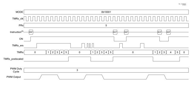
Figure 20-11. Rising Edge-Triggered Monostable Mode Timing Diagram (MODE = 10001)
