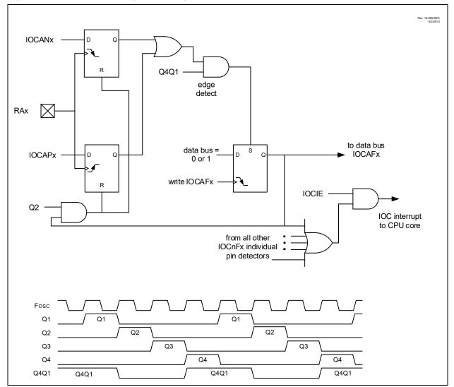
Figure 16-1. Interrupt-on-Change Block Diagram (PORTA Example)
