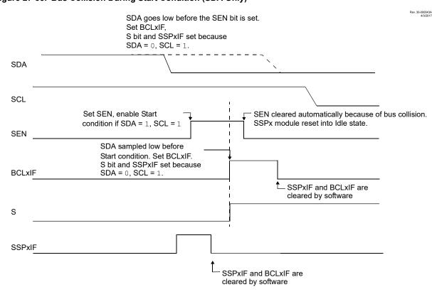
Figure 27-33. Bus Collision During Start Condition (SDA Only)
