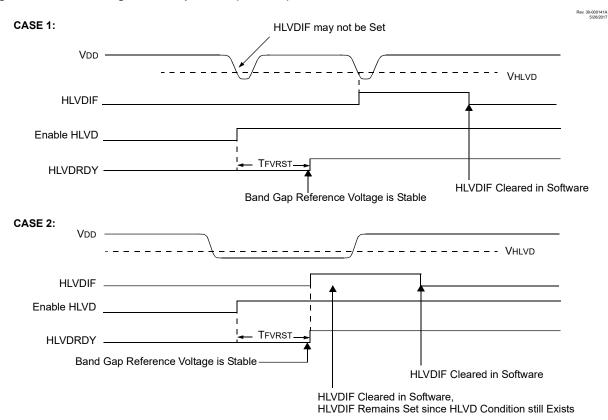
Figure 34-2. Low-Voltage Detect Operation (INTL = 1)
