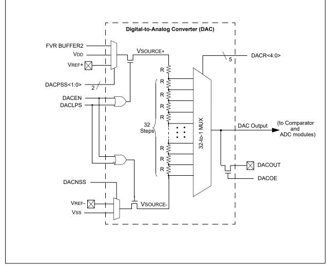
FIGURE 17-2: VOLTAGE REFERENCE OUTPUT BUFFER EXAMPLE
