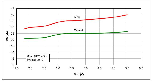
FIGURE 31-35: IPD, FIXED VOLTAGE REFERENCE (FVR), PIC16LF1938/9 ONLY 14 Max. 12 10 Typical 8 (Pu (JuA) 6 4 Max: 85°C + 3σ 2 Typical: 25°C 0 2.0 1.6 1.8 2.2 2.4 2.6 2.8 3.0 3.2 3.4 3.6 3.8 VDD (V)
