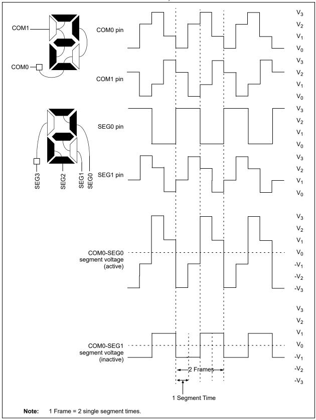
FIGURE 27-12: TYPE-B WAVEFORMS IN 1/2 MUX, 1/3 BIAS DRIVE
