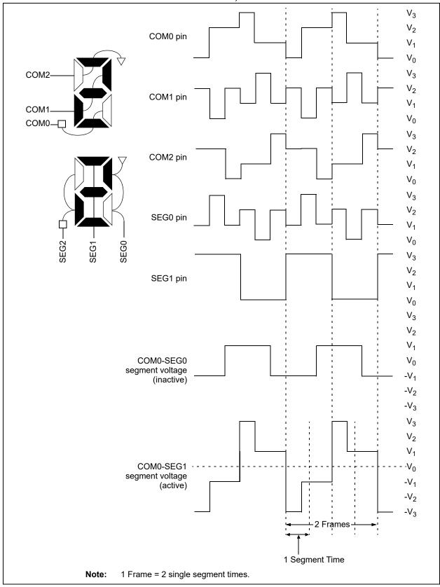
FIGURE 27-16: TYPE-B WAVEFORMS IN 1/3 MUX, 1/3 BIAS DRIVE
