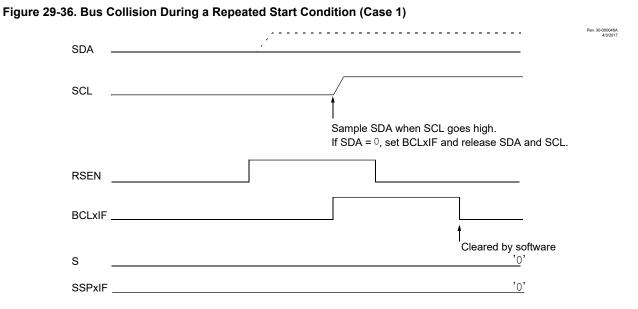
If SCL goes from high-to-low before the BRG times out and SDA has not already been asserted, a bus collision occurs. In this case, another host is attempting to transmit a data '1' during the Repeated Start condition, see Figure 29-37.
