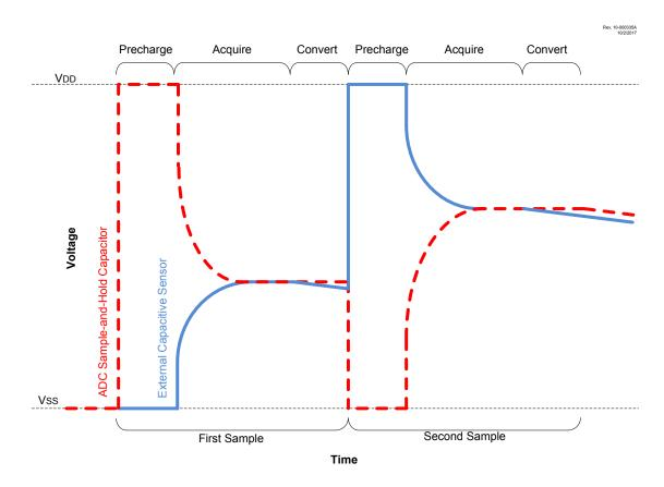
Figure 32-7. Differential CVD Measurement Waveform
