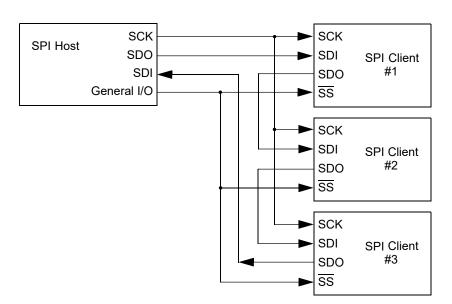
In a daisy-chain configuration, only the most recent byte on the bus is required by the client. Setting the BOEN bit will enable writes to the SSPxBUF register, even if the previous byte has not been read. This allows the software to ignore data that may not apply to it.
