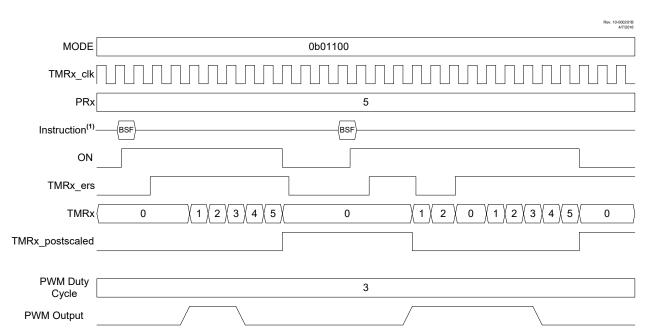
Figure 20-9. Edge-Triggered Hardware Limit One Shot Mode Timing Diagram (MODE = 01100)
