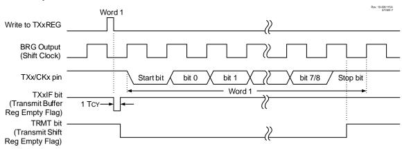
Figure 28-4. Asynchronous Transmission (Back-to-Back)
