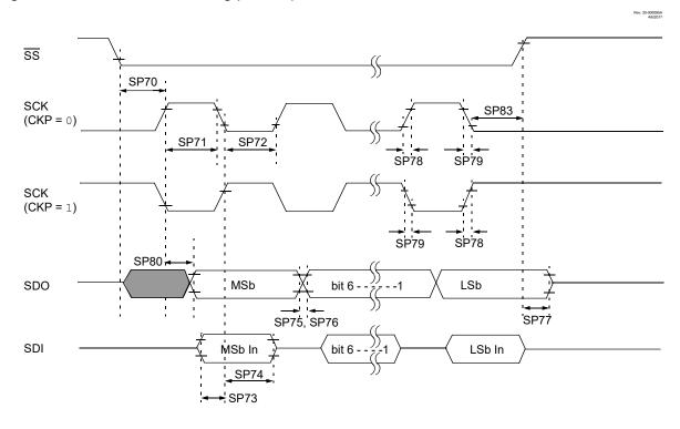
Figure 39-20. SPI Client Mode Timing (CKE = 1)
