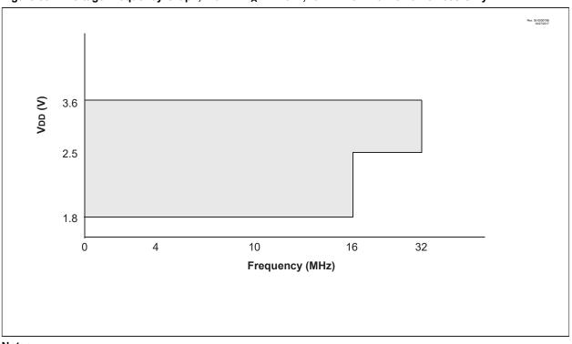
Figure 39-2. Voltage Frequency Graph, -40°C ≤ T<sub>A</sub>≤ +125°C, for PIC16LF18426/46 Devices Only
