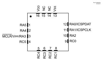
**Note:** It is recommended that the exposed bottom pad be connected to  $V_{SS}$ . See Table 3 for more information.
