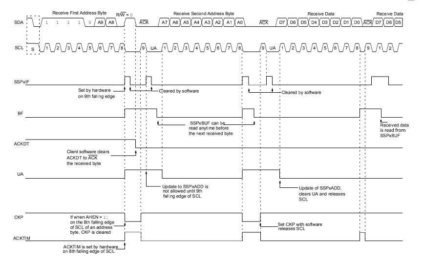
Figure 29-22. I<sup>2</sup>C Client, 10-Bit Address, Transmission (SEN = 0, AHEN = 0, DHEN = 0)
