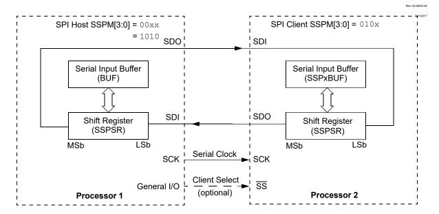
Data is shifted out of both Shift registers on the programmed clock edge and latched onto the opposite edge of the clock.
