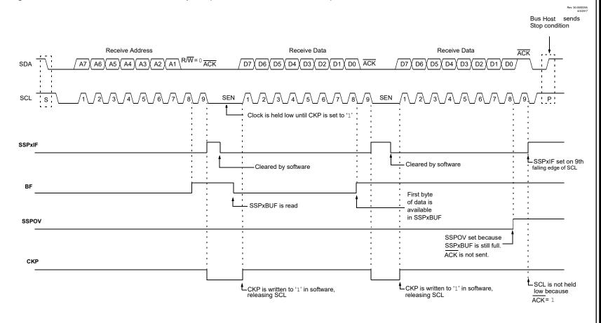
PIC16(L)F18426/46 MSSP - Host Synchronous Serial Port Module
