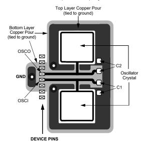
In planning the application's routing and I/O assignments, ensure that adjacent port pins and other signals in close proximity to the oscillator are benign (i.e., free of high frequencies, short rise and fall times, and other similar noise).
