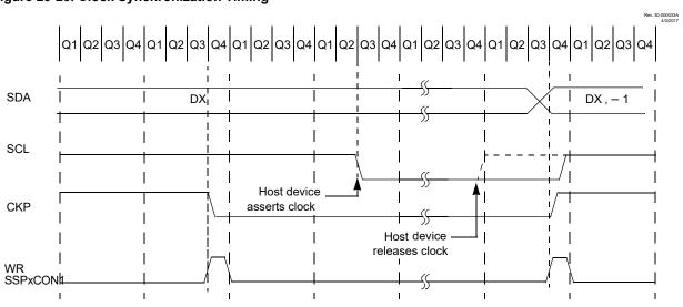
Figure 29-23. Clock Synchronization Timing
