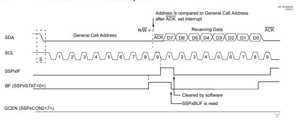
In 10-bit Address mode, the UA bit will not be set on the reception of the general call address. The client will prepare to receive the second byte as data, just as it would in 7-bit mode.
