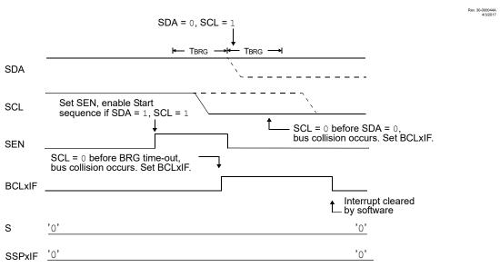
If the SDA pin is sampled low during this count, the BRG is reset and the SDA line is asserted early (Figure 29-35). If, however, a '1' is sampled on the SDA pin, the SDA pin is asserted low at the end of the BRG count. The Baud Rate
