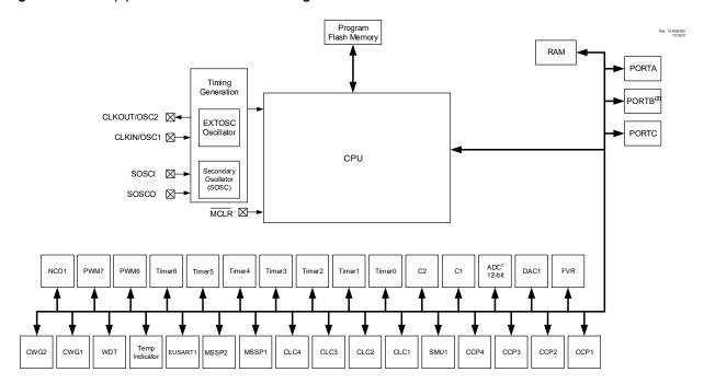
Figure 1-1. PIC16(L)F18426/46 Device Block Diagram
