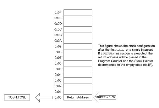
Figure 5-6. Accessing the Stack Example 3
