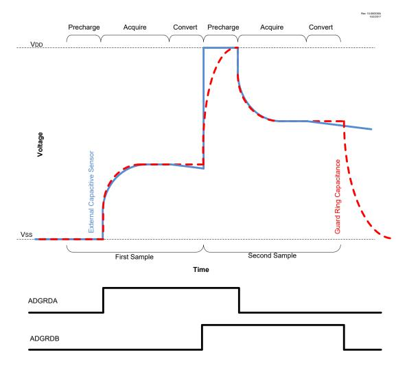
Figure 32-8. Differential CVD with Guard Ring Output Waveform
