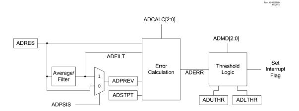
The operation of the ADC computational features is controlled by MD bits.
