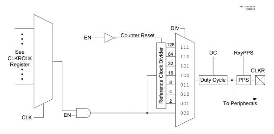
Figure 9-2. Clock Reference Timing
