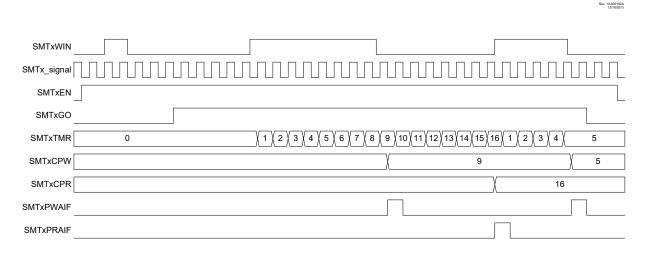
Figure 21-21. Windowed Counter Mode, Single Acquisition Timing Diagram
