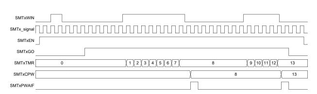
Figure 21-19. Gated Counter Mode, Single Acquisition Timing Diagram
