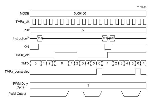
Figure 20-5. Edge-Triggered Hardware Limit Mode Timing Diagram (MODE = 00100)
