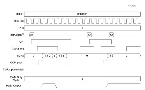
Figure 20-8. Edge-Triggered One Shot Mode Timing Diagram (MODE = 01001)
