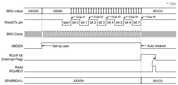
Figure 28-6. Automatic Baud Rate Calibration
