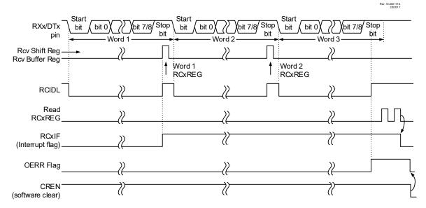
**Note:** This timing diagram shows three bytes appearing on the RXx input. The OERR flag is set because the RCxREG is not read before the third word is received.
