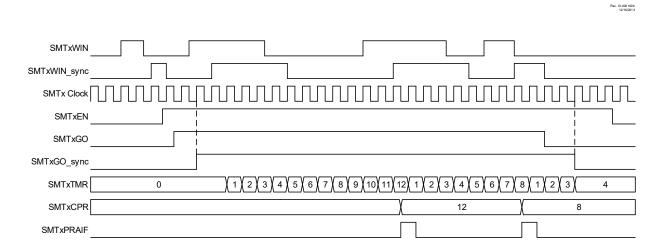
Figure 21-10. Windowed Measurement Mode, Single Acquisition Timing Diagram
