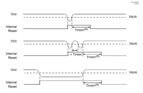
**Note:** T<sub>PWRT</sub> delay only if the PWRTS bit field is programmed to a value different from '11'.
