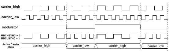
Figure 27-6. Full Synchronization (MDCHSYNC = 1, MDCLSYNC = 1)
