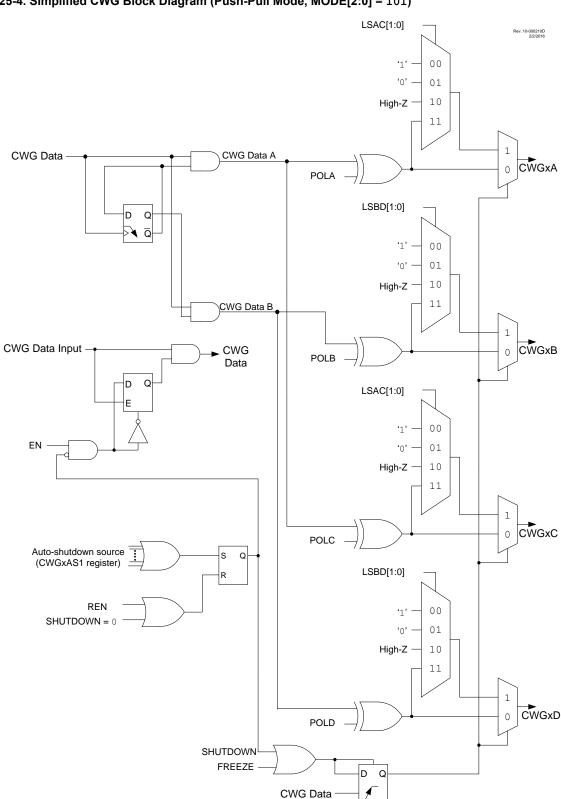
Figure 25-4. Simplified CWG Block Diagram (Push-Pull Mode, MODE[2:0] = 101)
