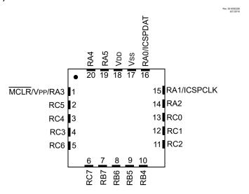
Note: It is recommended that the exposed bottom pad be connected to  $\ensuremath{V_{\text{SS}}}.$
