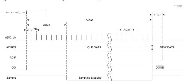
Figure 39-11. ADC Conversion Timing (ADC Clock from F<sub>RC</sub>)
