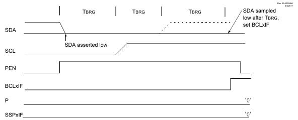
Figure 29-39. Bus Collision During a Stop Condition (Case 2)
