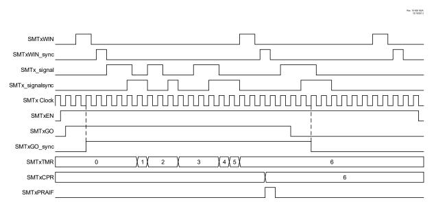
Figure 21-12. Gated Windowed Measurement Mode, Single Acquisition Timing Diagram
