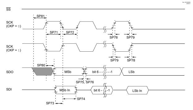
Figure 39-18. SPI Host Mode Timing (CKE = 1, SMP = 1)
