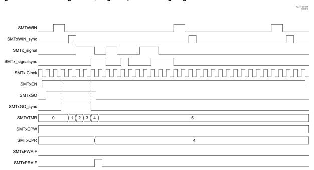
Figure 21-14. Time of Flight Mode, Single Acquisition Timing Diagram
