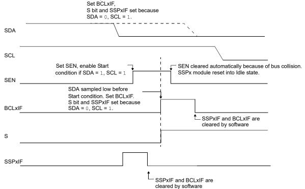
The Start condition begins with the SDA and SCL pins deasserted. When the SDA pin is sampled high, the Baud Rate Generator is loaded and counts down. If the SCL pin is sampled low while SDA is high, a bus collision occurs because it is assumed that another host is attempting to drive a data '1' during the Start condition.
