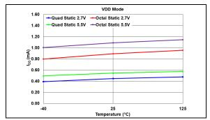
**FIGURE 2-4:** Average Device Supply Current - Inactive Interface (SCL =  $V_{IH}$  or  $V_{IL}$ ) vs. Voltage and Temperature, VRnB:VRnA = 00 ( $V_{DD}$  Mode).
