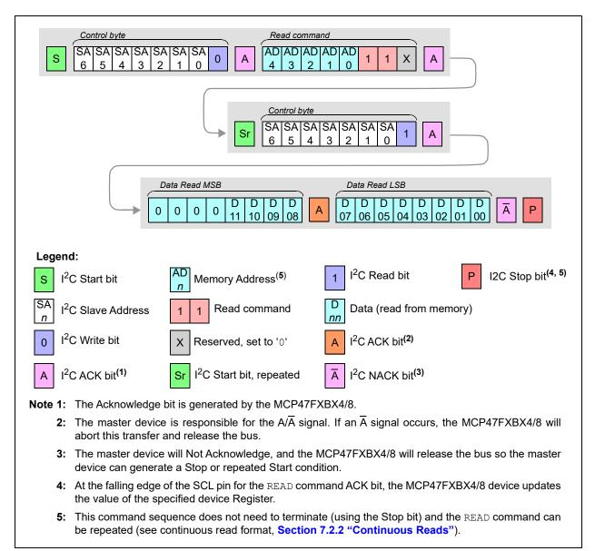
FIGURE 7-4: READ Command – Single Memory Address.
