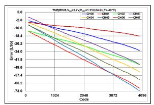
**FIGURE 2-65:** Total Unadjusted Error  $(V_{OUT})$  vs. DAC Code, T = -40°C,  $V_{DD} = 2.7$ V.
