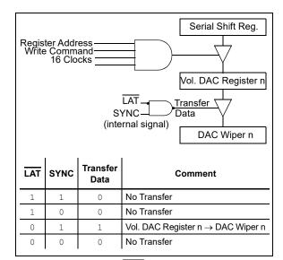
**FIGURE 5-9:**  $\overline{LAT}$  and DAC Interaction.
