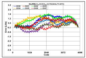
**FIGURE 2-110:** INL Error vs. DAC Code, T = -40°C,  $V_{DD} = 5.5V$ .
