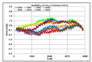
**FIGURE 2-78:** INL Error vs. DAC Code, T = +25°C,  $V_{DD} = 2.7V$ .
