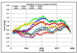
**FIGURE 2-18:** INL Error vs. DAC Code,  $T = +25^{\circ}\text{C}$ ,  $V_{DD} = 5.5V$ .
