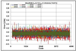
**FIGURE 2-90:** DNL Error vs. DAC Code,  $T = +25^{\circ}\text{C}$ ,  $V_{DD} = 2.7V$ .
