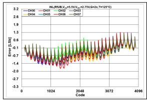
**FIGURE 2-76:** INL Error vs. DAC Code, T = +125°C,  $V_{DD} = 5.5$ V.
