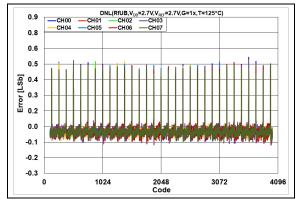
**FIGURE 2-85:** DNL Error vs. DAC Code,  $T = +125^{\circ}\text{C}$ ,  $V_{DD} = 2.7V$ .
