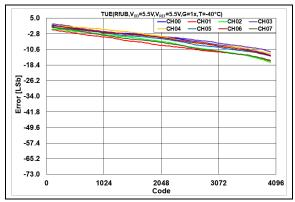
**FIGURE 2-56:** Total Unadjusted Error  $(V_{OUT})$  vs. DAC Code, T = -40°C,  $V_{DD} = 5.5$ V.
