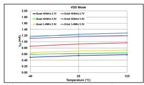
**FIGURE 2-1:** Average Device Supply Current vs.  $F_{SCL}$  Frequency, Voltage and Temperature - Active Interface, VRnB:VRnA = 00,  $(V_{DD} Mode)$ .
