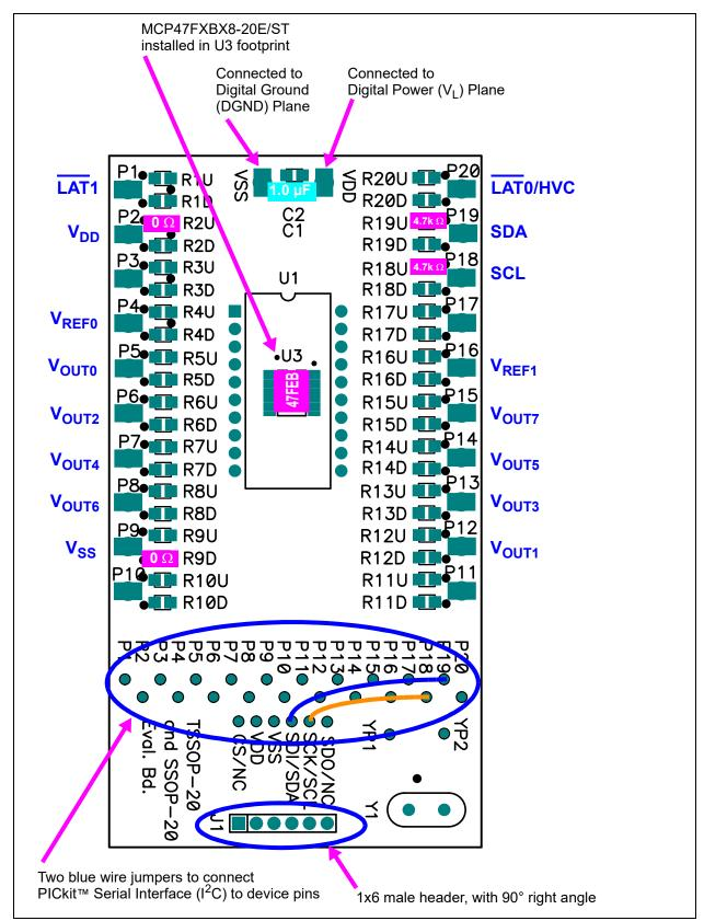
FIGURE 9-1: MCP47FXBX4/8 Evaluation Board Circuit Using TSSOP20EV.
