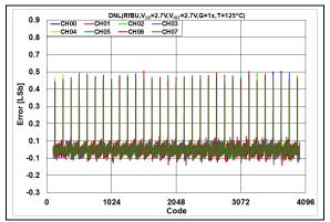
**FIGURE 2-121:** DNL Error vs. DAC Code, T = +125°C,  $V_{DD} = 2.7V$ .
