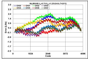
**FIGURE 2-42:** INL Error vs. DAC Code, T = +25°C,  $V_{DD} = 2.7V$ .
