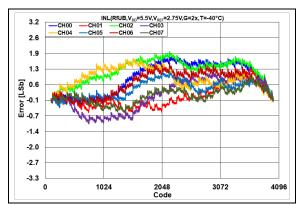
**FIGURE 2-74:** INL Error vs. DAC Code, T = -40°C,  $V_{DD} = 5.5V$ .
