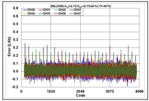
**FIGURE 2-26:** DNL Error vs. DAC Code, T = -40°C,  $V_{DD} = 2.7V$ .
