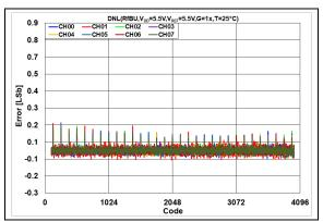
**FIGURE 2-117:** DNL Error vs. DAC Code,  $T = +25^{\circ}\text{C}$ ,  $V_{DD} = 5.5V$ .
