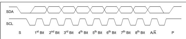
FIGURE B-7: TYPICAL 8-BIT I<sup>2</sup>C WAVEFORM FORMAT.
