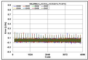
**FIGURE 2-116:** DNL Error vs. DAC Code, T = -40°C,  $V_{DD} = 5.5V$ .
