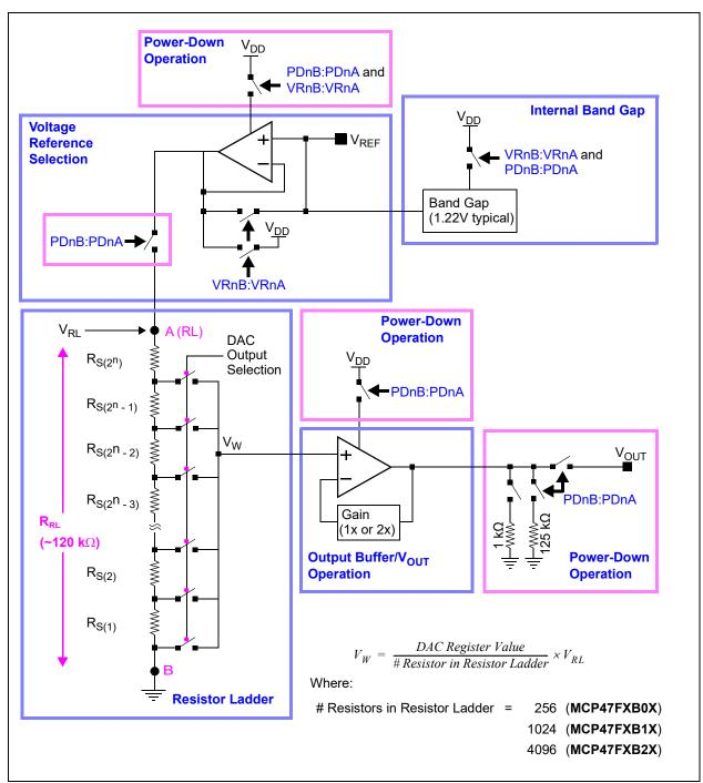
FIGURE 5-1: MCP47FXBX4/8 DAC Module Block Diagram.
