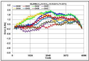
FIGURE 2-104: INL Error vs. DAC Code, T = -40°C,  $V_{DD} = 5.5V$ .
