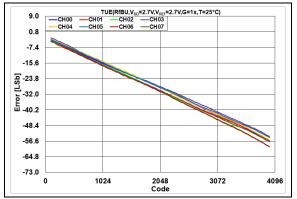
**FIGURE 2-96:** Total Unadjusted Error  $(V_{OUT})$  vs. DAC Code, T = +25°C,  $V_{DD} = 2.7V$ .
