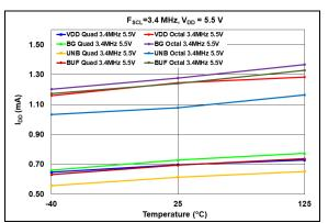
**FIGURE 2-8:** Average Device Supply Active Current ( $I_{DDA}$ ) (at 5.5V and  $F_{SCL}$  = 3.4 MHz) vs. Temperature and DAC Reference Voltage Mode.
