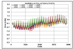
FIGURE 2-73: INL Error vs. DAC Code, T = +125°C,  $V_{DD} = 2.7V$ .
