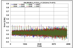
**FIGURE 2-53:** DNL Error vs. DAC Code, T = -40°C,  $V_{DD} = 5.5$ V.
