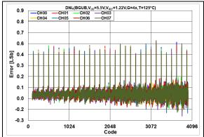
FIGURE 2-55: DNL Error vs. DAC Code,  $T = +125^{\circ}\text{C}$ ,  $V_{DD} = 5.5V$ .
