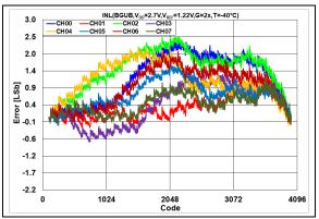
**FIGURE 2-41:** INL Error vs. DAC Code, T = -40°C,  $V_{DD} = 2.7V$ .
