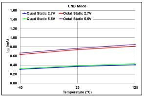
**FIGURE 2-9:** Average Device Supply Current - Inactive Interface (SCL =  $V_{IH}$  or  $V_{IL}$ ) vs. Voltage and Temperature, VRnB:VRnA = 10 ( $V_{RFF}$  Unbuffered Mode).
