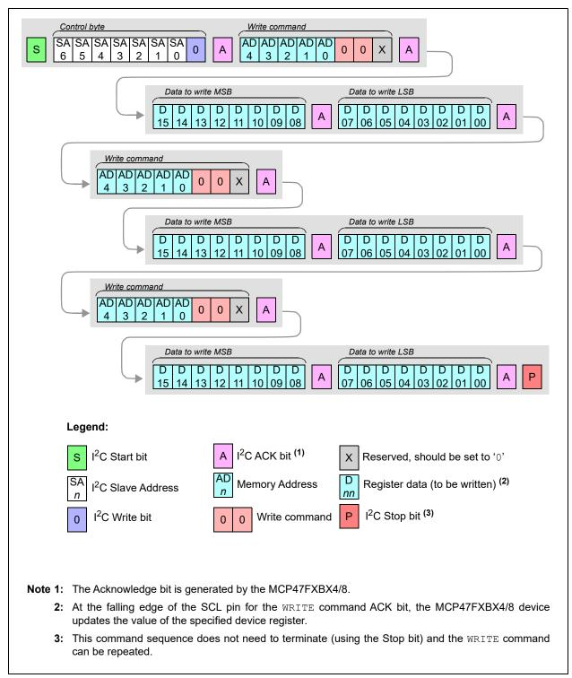
FIGURE 7-3: Continuous WRITE Commands (Volatile Memory Only).
