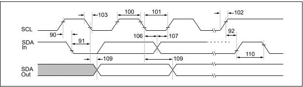
**FIGURE 1-7:** I<sup>2</sup>C Bus Timing Waveforms.
