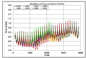
**FIGURE 2-22:** INL Error vs. DAC Code, T = +125°C,  $V_{DD} = 2.7V$ .
