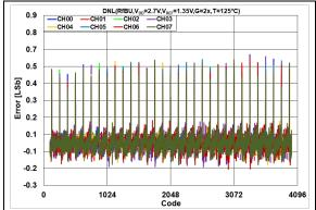
FIGURE 2-127: DNL Error vs. DAC Code,  $T = +125^{\circ}\text{C}$ ,  $V_{DD} = 2.7V$ .
