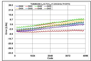
**FIGURE 2-34:** Total Unadjusted Error  $(V_{OUT})$  vs. DAC Code, T = +125°C,  $V_{DD} = 2.7V$ .
