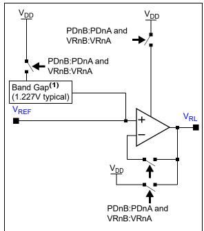
Note 1: The band gap voltage (V<sub>BG</sub>) is 1.22V typical. The band gap output goes through the buffer with a 2x gain to create the V<sub>RL</sub> voltage. See Table 5-1 for additional information on the band gap circuit.
