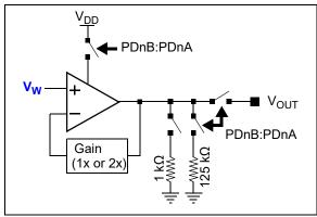
FIGURE 5-5: Output Driver Block Diagram.
