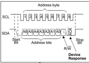
FIGURE 8-1: I<sup>2</sup>C Bus Connection Test.
