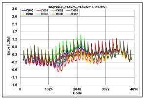
**FIGURE 2-19:** INL Error vs. DAC Code, T = +125°C,  $V_{DD} = 5.5V$ .
