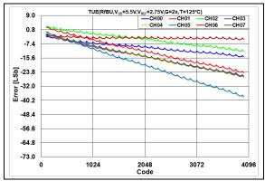
**FIGURE 2-100:** Total Unadjusted Error  $(V_{OUT})$  vs. DAC Code, T = +125°C,  $V_{DD} = 5.5$ V.
