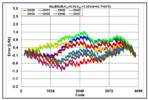
**FIGURE 2-45:** INL Error vs. DAC Code, T = +25°C,  $V_{DD} = 5.5$ V.
