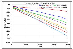
**FIGURE 2-62:** Total Unadjusted Error  $(V_{OUT})$  vs. DAC Code, T = -40°C,  $V_{DD} = 5.5$ V.
