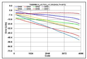
**FIGURE 2-101:** Total Unadjusted Error  $(V_{OUT})$  vs. DAC Code, T = -40°C,  $V_{DD} = 2.7V$ .
