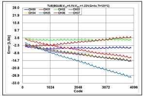
**FIGURE 2-37:** Total Unadjusted Error  $(V_{OUT})$  vs. DAC Code, T = +125°C,  $V_{DD} = 5.5$ V.
