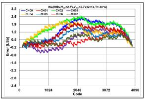
**FIGURE 2-107:** INL Error vs. DAC Code, T = -40°C,  $V_{DD} = 2.7V$ .
