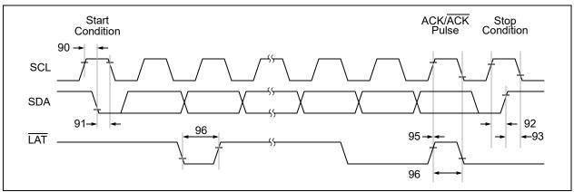
**FIGURE 1-5:**  $I^2C$  Bus Start/Stop Bits and  $\overline{LAT}$  Timing Waveforms.
