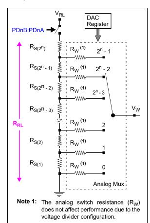
FIGURE 5-2: Resistor Ladder Model.
