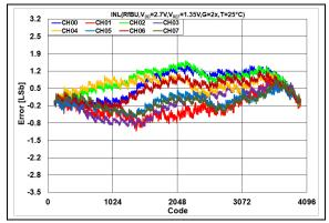
**FIGURE 2-114:** INL Error vs. DAC Code,  $T = +25^{\circ}\text{C}$ ,  $V_{DD} = 2.7V$ .
