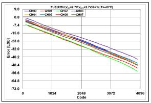
**FIGURE 2-95:** Total Unadjusted Error  $(V_{OUT})$  vs. DAC Code, T = -40°C,  $V_{DD} = 2.7$ V.
