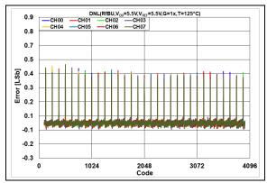
**FIGURE 2-118:** DNL Error vs. DAC Code,  $T = +125^{\circ}\text{C}$ ,  $V_{DD} = 5.5V$ .
