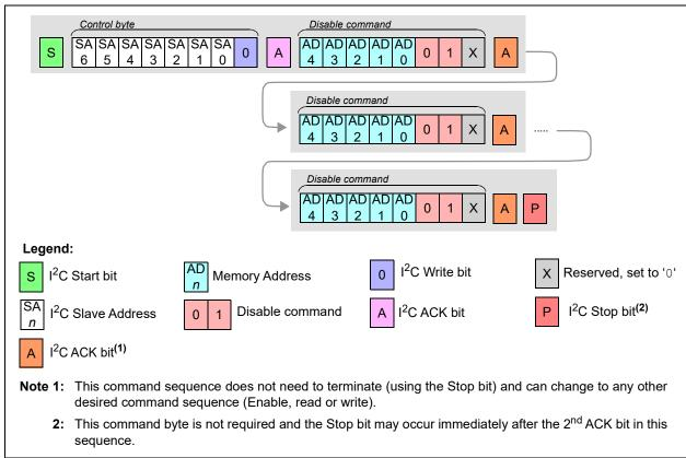
FIGURE 7-12: I<sup>2</sup>C Disable Command Sequence.
