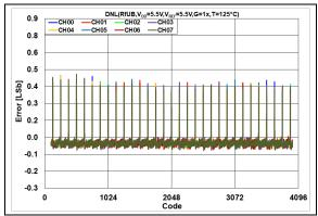
**FIGURE 2-82:** DNL Error vs. DAC Code,  $T = +125^{\circ}\text{C}$ ,  $V_{DD} = 5.5V$ .
