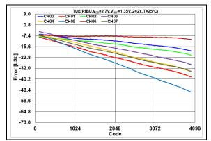
**FIGURE 2-102:** Total Unadjusted Error  $(V_{OUT})$  vs. DAC Code, T = +25°C,  $V_{DD} = 2.7$ V.
