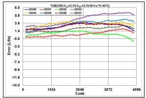
**FIGURE 2-11:** Total Unadjusted Error  $(V_{OUT})$  vs. DAC Code, T = -40°C,  $V_{DD} = 5.5$ V.
