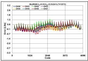
**FIGURE 2-70:** INL Error vs. DAC Code,  $T = +125^{\circ}\text{C}$ ,  $V_{DD} = 5.5\text{V}$ .
