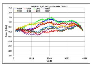
**FIGURE 2-105:** INL Error vs. DAC Code,  $T = +25^{\circ}C$ ,  $V_{DD} = 5.5V$ .
