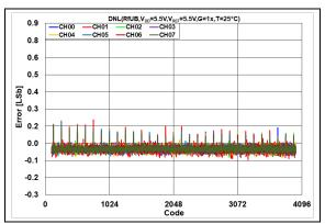
**FIGURE 2-81:** DNL Error vs. DAC Code,  $T = +25^{\circ}\text{C}$ ,  $V_{DD} = 5.5V$ .
