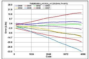
**FIGURE 2-35:** Total Unadjusted Error  $(V_{OUT})$  vs. DAC Code, T = -40°C,  $V_{DD} = 5.5$ V.
