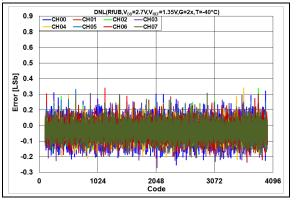
**FIGURE 2-89:** DNL Error vs. DAC Code, T = -40°C,  $V_{DD} = 2.7V$ .
