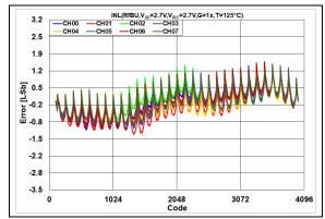
**FIGURE 2-109:** INL Error vs. DAC Code, T = +125°C,  $V_{DD} = 2.7V$ .
