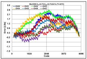
**FIGURE 2-20:** INL Error vs. DAC Code, T = -40°C,  $V_{DD} = 2.7V$ .
