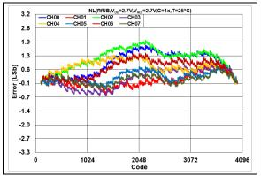
**FIGURE 2-72:** INL Error vs. DAC Code, T = +25°C,  $V_{DD} = 2.7V$ .
