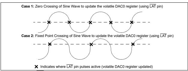
FIGURE 5-10: LAT Pin Operation Example.
