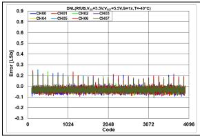
**FIGURE 2-80:** DNL Error vs. DAC Code, T = -40°C,  $V_{DD} = 5.5$ V.
