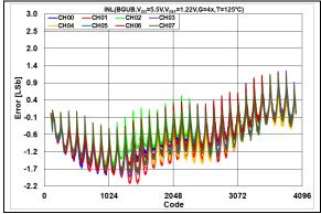
**FIGURE 2-46:** INL Error vs. DAC Code,  $T = +125^{\circ}\text{C}$ ,  $V_{DD} = 5.5V$ .
