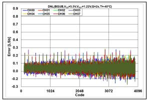
**FIGURE 2-47:** DNL Error vs. DAC Code, T = -40°C,  $V_{DD} = 5.5V$ .
