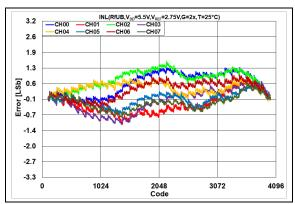
**FIGURE 2-75:** INL Error vs. DAC Code,  $T = +25^{\circ}C$ ,  $V_{DD} = 5.5V$ .
