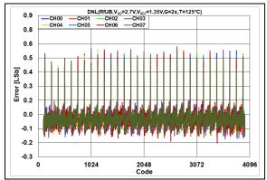
**FIGURE 2-91:** DNL Error vs. DAC Code,  $T = +125^{\circ}\text{C}$ ,  $V_{DD} = 2.7V$ .
