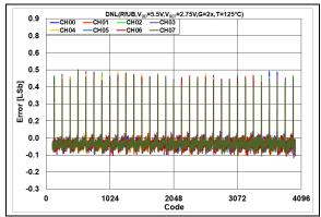
**FIGURE 2-88:** DNL Error vs. DAC Code,  $T = +125^{\circ}\text{C}$ ,  $V_{DD} = 5.5V$ .
