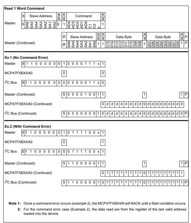
FIGURE 7-6: I<sup>2</sup>C ACK/NACK Behavior (READ Command Example).
