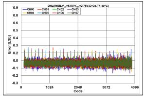
**FIGURE 2-86:** DNL Error vs. DAC Code, T = -40°C,  $V_{DD} = 5.5V$ .
