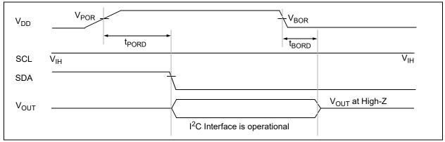
FIGURE 1-3: Power-on and Brown-out Reset Waveforms.
