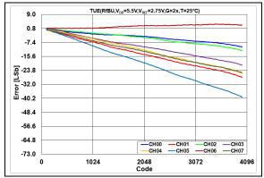
FIGURE 2-99: Total Unadjusted Error  $(V_{OUT})$  vs. DAC Code, T = +25°C,  $V_{DD} = 5.5$ V.
