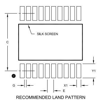
Units **MILLIMETERS** Dimension Limits MIN NOM MAX Contact Pitch 0.65 BSC Ε Contact Pad Spacing С 5.90 Contact Pad Width (X20) X1 0.45 Contact Pad Length (X20) Y1 1.45 Distance Between Pads G 0.20
