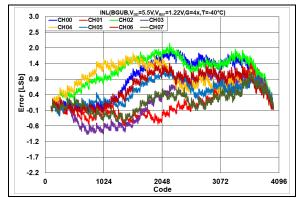
**FIGURE 2-44:** INL Error vs. DAC Code, T = -40°C,  $V_{DD} = 5.5V$ .
