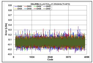
**FIGURE 2-125:** DNL Error vs. DAC Code,  $T = -40^{\circ}C$ ,  $V_{DD} = 2.7V$ .
