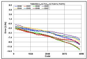
**FIGURE 2-15:** Total Unadjusted Error  $(V_{OUT})$  vs. DAC Code, T = +25°C,  $V_{DD} = 2.7V$ .
