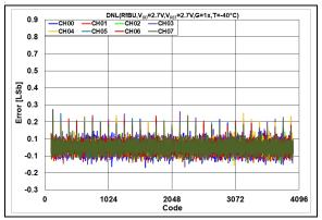
**FIGURE 2-119:** DNL Error vs. DAC Code, T = -40°C,  $V_{DD} = 2.7V$ .
