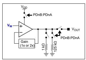
**FIGURE 5-8:** V<sub>OUT</sub> Power-Down Block Diagram.
