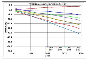
**FIGURE 2-98:** Total Unadjusted Error  $(V_{OUT})$  vs. DAC Code, T = -40°C,  $V_{DD} = 5.5$ V.
