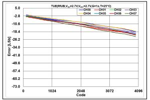
**FIGURE 2-60:** Total Unadjusted Error  $(V_{OUT})$  vs. DAC Code, T = +25°C,  $V_{DD} = 2.7V$ .
