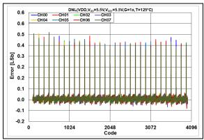
**FIGURE 2-25:** DNL Error vs. DAC Code,  $T = +125^{\circ}\text{C}$ ,  $V_{DD} = 5.5V$ .
