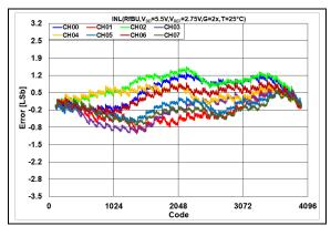
FIGURE 2-111: INL Error vs. DAC Code, T = +25°C,  $V_{DD} = 5.5$ V.
