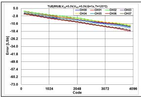
**FIGURE 2-58:** Total Unadjusted Error  $(V_{OUT})$  vs. DAC Code, T = +125°C,  $V_{DD} = 5.5$ V.
