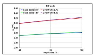
**FIGURE 2-5:** Average Device Supply Current - Inactive Interface (SCL =  $V_{IH}$  or  $V_{IL}$ ) vs. Voltage and Temperature, VRnB:VRnA = 01 (Band Gap Mode).
