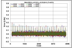
**FIGURE 2-23:** DNL Error vs. DAC Code, T = -40°C,  $V_{DD} = 5.5V$ .
