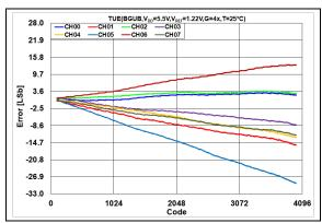
**FIGURE 2-36:** Total Unadjusted Error  $(V_{OUT})$  vs. DAC Code, T = +25°C,  $V_{DD} = 5.5$ V.
