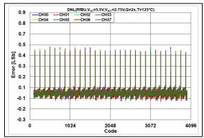
**FIGURE 2-124:** DNL Error vs. DAC Code,  $T = +125^{\circ}\text{C}$ ,  $V_{DD} = 5.5V$ .
