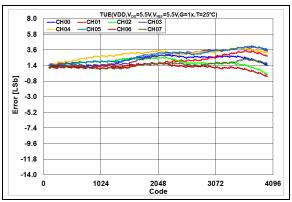
**FIGURE 2-12:** Total Unadjusted Error  $(V_{OUT})$  vs. DAC Code, T = +25°C,  $V_{DD} = 5.5$ V.
