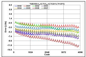
**FIGURE 2-16:** Total Unadjusted Error  $(V_{OUT})$  vs. DAC Code,  $T = +125^{\circ}\text{C}$ ,  $V_{DD} = 2.7V$ .
