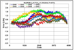
**FIGURE 2-77:** INL Error vs. DAC Code, T = -40°C,  $V_{DD} = 2.7V$ .
