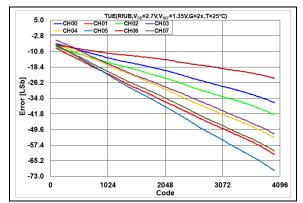
**FIGURE 2-66:** Total Unadjusted Error  $(V_{OUT})$  vs. DAC Code, T = +25°C,  $V_{DD} = 2.7$ V.
