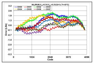
**FIGURE 2-68:** INL Error vs. DAC Code, T = -40°C,  $V_{DD} = 5.5V$ .
