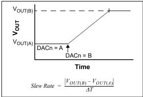
FIGURE 5-6: V<sub>OUT</sub> Pin Slew Rate.
