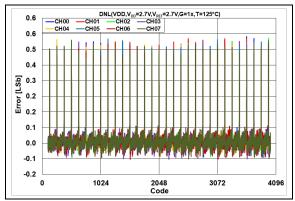
**FIGURE 2-28:** DNL Error vs. DAC Code, T = +125°C,  $V_{DD} = 2.7V$ .
