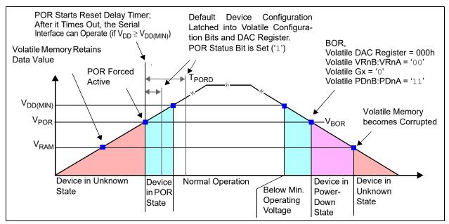
FIGURE 4-1: Power-On/Brown-Out Reset Operation.
