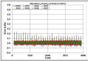
**FIGURE 2-24:** DNL Error vs. DAC Code,  $T = +25^{\circ}\text{C}$ ,  $V_{DD} = 5.5V$ .
