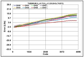
FIGURE 2-33: Total Unadjusted Error  $(V_{OUT})$  vs. DAC Code, T = +25°C,  $V_{DD} = 2.7V$ .
