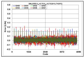
**FIGURE 2-27:** DNL Error vs. DAC Code,  $T = +25^{\circ}\text{C}$ ,  $V_{DD} = 2.7V$ .
