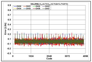
**FIGURE 2-120:** DNL Error vs. DAC Code,  $T = +25^{\circ}\text{C}$ ,  $V_{DD} = 2.7V$ .
