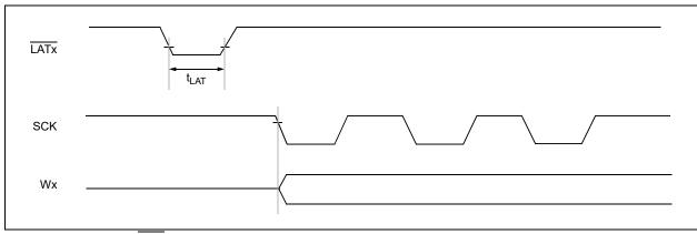
FIGURE 1-2: LAT Pin Waveforms.
