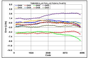
**FIGURE 2-14:** Total Unadjusted Error  $(V_{OUT})$  vs. DAC Code, T = -40°C,  $V_{DD} = 2.7$ V.
