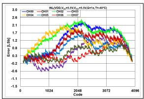
**FIGURE 2-17:** INL Error vs. DAC Code, T = 40°C,  $V_{DD} = 5.5$ V.
