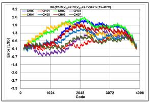
**FIGURE 2-71:** INL Error vs. DAC Code, T = -40°C,  $V_{DD} = 2.7V$ .
