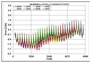
**FIGURE 2-40:** INL Error vs. DAC Code,  $T = +125^{\circ}\text{C}$ ,  $V_{DD} = 5.5V$ .
