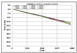
**FIGURE 2-93:** Total Unadjusted Error  $(V_{OUT})$  vs. DAC Code,  $T = +25^{\circ}C, V_{DD} = 5.5V$ .
