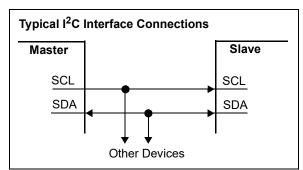
FIGURE B-1: TYPICAL I<sup>2</sup>C INTERFACE.
