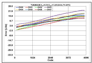
**FIGURE 2-29:** Total Unadjusted Error  $(V_{OUT})$  vs. DAC Code, T = -40°C,  $V_{DD} = 5.5$ V.
