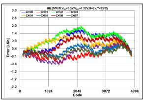
**FIGURE 2-39:** INL Error vs. DAC Code,  $T = +25^{\circ}C$ ,  $V_{DD} = 5.5V$ .
