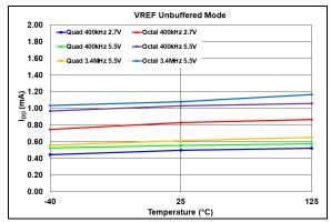
FIGURE 2-7: Average Device Supply Current vs. F<sub>SCL</sub> Frequency, Voltage and Temperature - Active Interface, VRnB:VRnA = 10 (V<sub>REF</sub> Unbuffered Mode).
