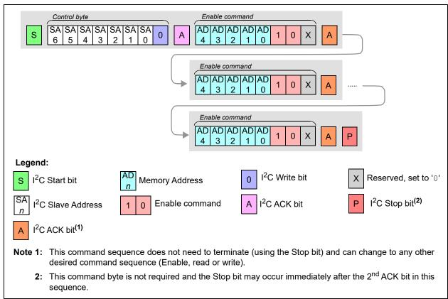
FIGURE 7-11: I<sup>2</sup>C Enable Command Sequence.
