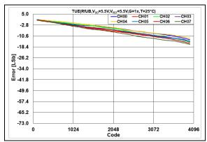
**FIGURE 2-57:** Total Unadjusted Error  $(V_{OUT})$  vs. DAC Code,  $T = +25^{\circ}C, V_{DD} = 5.5V$ .
