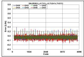
**FIGURE 2-84:** DNL Error vs. DAC Code,  $T = +25^{\circ}C$ ,  $V_{DD} = 2.7V$ .
