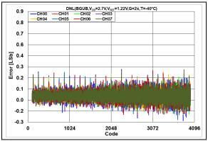
**FIGURE 2-50:** DNL Error vs. DAC Code, T = -40°C,  $V_{DD} = 2.7V$ .
