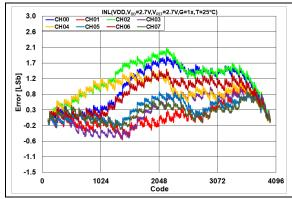
**FIGURE 2-21:** INL Error vs. DAC Code, T = +25°C,  $V_{DD} = 2.7V$ .
