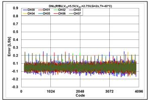
**FIGURE 2-122:** DNL Error vs. DAC Code, T = -40°C,  $V_{DD} = 5.5V$ .
