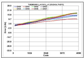
**FIGURE 2-30:** Total Unadjusted Error  $(V_{OUT})$  vs. DAC Code, T = +25°C,  $V_{DD} = 5.5$ V.
