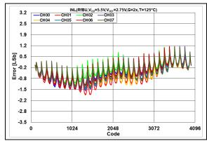
**FIGURE 2-112:** INL Error vs. DAC Code, T = +125°C,  $V_{DD} = 5.5$ V.
