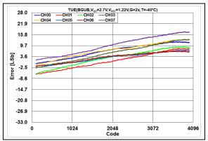
**FIGURE 2-32:** Total Unadjusted Error  $(V_{OUT})$  vs. DAC Code, T = -40°C,  $V_{DD} = 2.7$ V.
