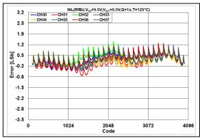
**FIGURE 2-106:** INL Error vs. DAC Code,  $T = +125^{\circ}\text{C}$ ,  $V_{DD} = 5.5\text{V}$ .
