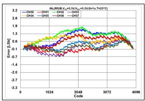
**FIGURE 2-69:** INL Error vs. DAC Code,  $T = +25^{\circ}C$ ,  $V_{DD} = 5.5V$ .
