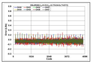
**FIGURE 2-87:** DNL Error vs. DAC Code,  $T = +25^{\circ}\text{C}$ ,  $V_{DD} = 5.5V$ .
