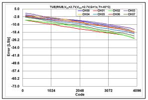
**FIGURE 2-59:** Total Unadjusted Error  $(V_{OUT})$  vs. DAC Code, T = -40°C,  $V_{DD} = 2.7$ V.
