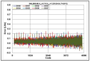
FIGURE 2-51: DNL Error vs. DAC Code, T = +25°C  $V_{DD} = 2.7V$ .
