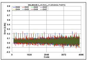
**FIGURE 2-48:** DNL Error vs. DAC Code,  $T = +25^{\circ}\text{C }V_{DD} = 5.5\text{V}.$
