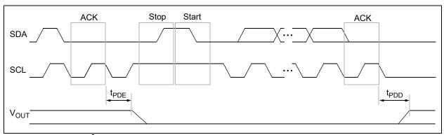
FIGURE 1-4: I<sup>2</sup>C Power-Down Command Waveforms.
