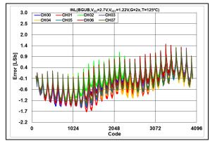
**FIGURE 2-43:** INL Error vs. DAC Code, T = +125°C,  $V_{DD} = 2.7V$ .
