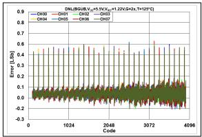
**FIGURE 2-49:** DNL Error vs. DAC Code,  $T = +125^{\circ}\text{C}$ ,  $V_{DD} = 5.5V$ .
