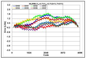
**FIGURE 2-108:** INL Error vs. DAC Code,  $T = +25^{\circ}\text{C}$ ,  $V_{DD} = 2.7V$ .
