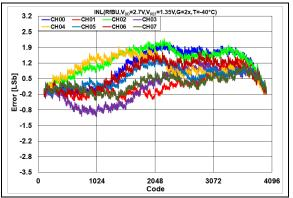
FIGURE 2-113: INL Error vs. DAC Code, T = -40°C,  $V_{DD} = 2.7V$ .
