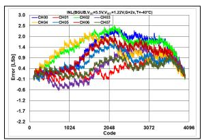
**FIGURE 2-38:** INL Error vs. DAC Code, T = -40°C,  $V_{DD} = 5.5V$ .
