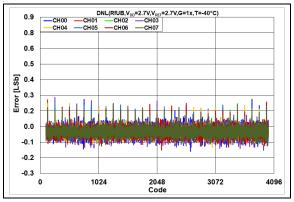
FIGURE 2-83: DNL Error vs. DAC Code, T = -40°C,  $V_{DD} = 2.7V$ .
