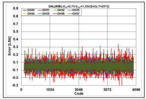
**FIGURE 2-126:** DNL Error vs. DAC Code,  $T = +25^{\circ}\text{C}$ ,  $V_{DD} = 2.7V$ .
