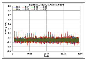
**FIGURE 2-123:** DNL Error vs. DAC Code,  $T = +25^{\circ}C$ ,  $V_{DD} = 5.5V$ .
