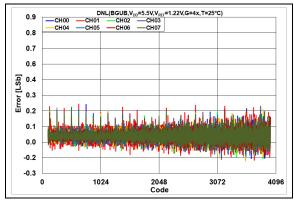
**FIGURE 2-54:** DNL Error vs. DAC Code, T = +25°C,  $V_{DD} = 5.5$ V.
