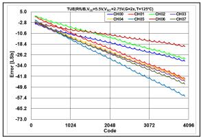
**FIGURE 2-64:** Total Unadjusted Error  $(V_{OUT})$  vs. DAC Code, T = +125°C,  $V_{DD} = 5.5$ V.
