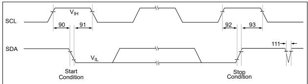
FIGURE 1-6: I<sup>2</sup>C Bus Start/Stop Bits Timing Waveforms.
