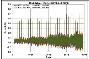
FIGURE 2-52: DNL Error vs. DAC Code,  $T = +125^{\circ}\text{C}$ ,  $V_{DD} = 2.7V$ .
