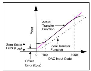
FIGURE C-2: OFFSET ERROR (ZERO GAIN ERROR).
