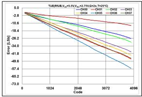
**FIGURE 2-63:** Total Unadjusted Error  $(V_{OUT})$  vs. DAC Code,  $T = +25^{\circ}C$ ,  $V_{DD} = 5.5V$ .
