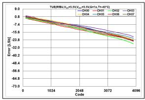
**FIGURE 2-92:** Total Unadjusted Error  $(V_{OUT})$  vs. DAC Code, T = -40°C,  $V_{DD} = 5.5$ V.
