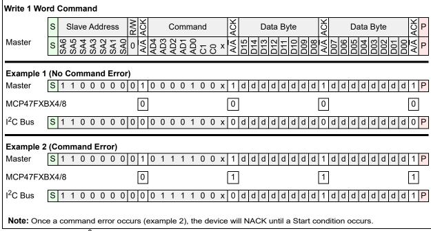
**FIGURE 7-2:**  $I^2C$  ACK/NACK Behavior (Write Command Example).
