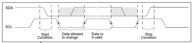
FIGURE B-8: I<sup>2</sup>C DATA STATES AND BIT SEQUENCE.
