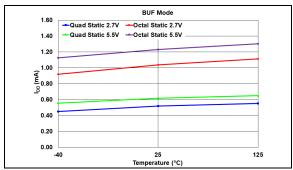
**FIGURE 2-6:** Average Device Supply Current - Inactive Interface (SCL =  $V_{IH}$  or  $V_{IL}$ ) vs. Voltage and Temperature, VRnB:VRnA = 11 ( $V_{RFF}$  Buffered Mode).
