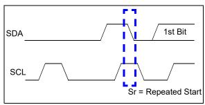
FIGURE B-5: REPEAT START CONDITION WAVEFORM.
