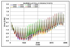
**FIGURE 2-79:** INL Error vs. DAC Code, T = +125°C,  $V_{DD} = 2.7V$ .
