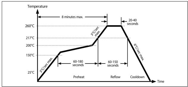
FIGURE 6-1: Solder Reflow Profile.
