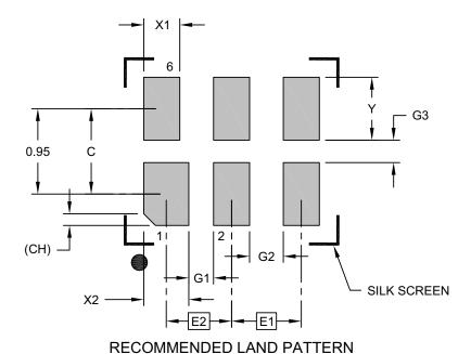
MILLIMETERS Units **Dimension Limits** MIN NOM MAX Contact Pitch E1 0.78 BSC Contact Pitch E2 0.73 BSC Contact Spacing С Contact Width (X4) X1 0.40 Contact Width (X2) X2 0.45 Contact Pad Length (X6) Υ 0.70 Space Between Contacts (X4) G1 0.28 Space Between Contacts (X3) G2 0.38 G3 0.25 Space Between Contacts (X3) СН 0.13 X 45° REF Contact 1 Index Chamfer
