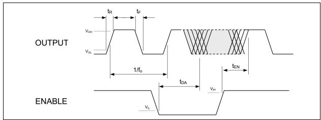
FIGURE 4-1: DSC612 Output Waveform.
